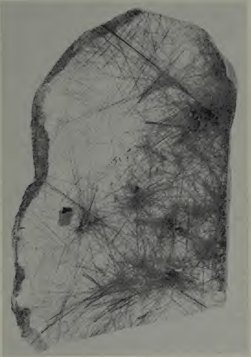
FIG. 96. Rutile needles enclosed in quartz crystal. Minas Gerais, Brazil. Polished section, approximately 6 \times 9 in. Harvard coll.
