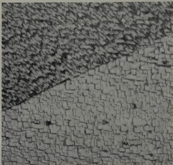
FIG. 81. Dauphiné twin in etched section of quartz. Bottom part nearly parallel to r , top part nearly parallel to z . Photomicrograph.
