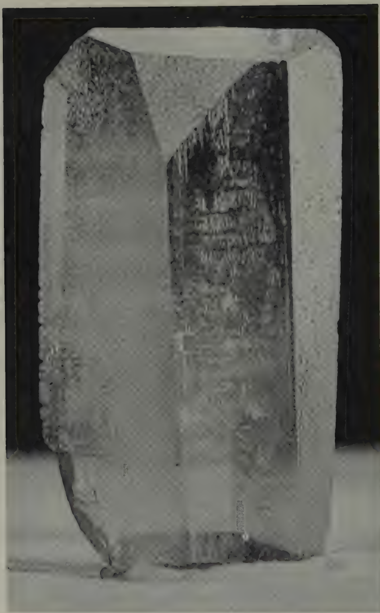
FIG. 44. Twisted crystal of smoky quartz elongated along an a -axis. The crystal is oriented with an a -axis vertical and the c -axis horizontal. The triangular face at top is x(51\bar{6}1) , the vertical faces to left and right are r and z and the vertical face in front is (10\bar{1}0) . Right-handed. Crystal about 2 in. long. Switzerland. Amer. Mus. Nat. Hist. coll.
