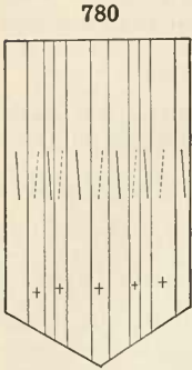
Plagioclase with twinning lamellæ. Fig. 780 section \parallel c (001) showing vibration-directions (cf. Fig. 784), ordinary light; Fig. 781 section in polarized light.
