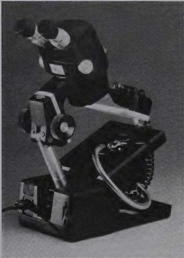
FIG. 20.4 A low-power stereoscopic wide-field microscope, designed to provide several different methods for illuminating gemstones (courtesy of Gemological Institute of America, GEM Instruments Corporation, Santa Monica, California).
