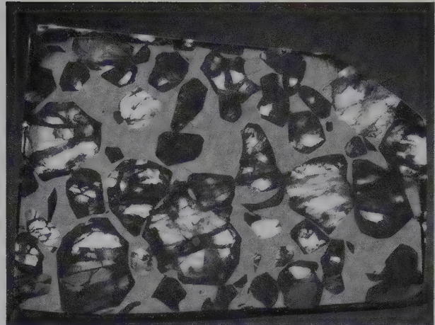
FIG. 5.6 A polished and etched slab of the Imilac pallasite (a silicate-metal meteorite) displaying centimeter-sized, well-rounded olivines dispersed in metal (an iron-nickel alloy). The width of the sample is about 7 cm. (Photograph courtesy of the Smithsonian Institution, Washington, D.C.)
