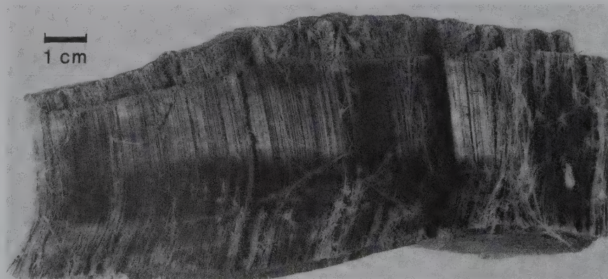
FIG. 19.53 Crocidolite, an asbestiform variety of the amphibole riebeckite (in the trade this is also known as “blue asbestos”), Kuruman, Cape Province, Republic of South Africa (compare with Figs. 19.50 and 19.55).
