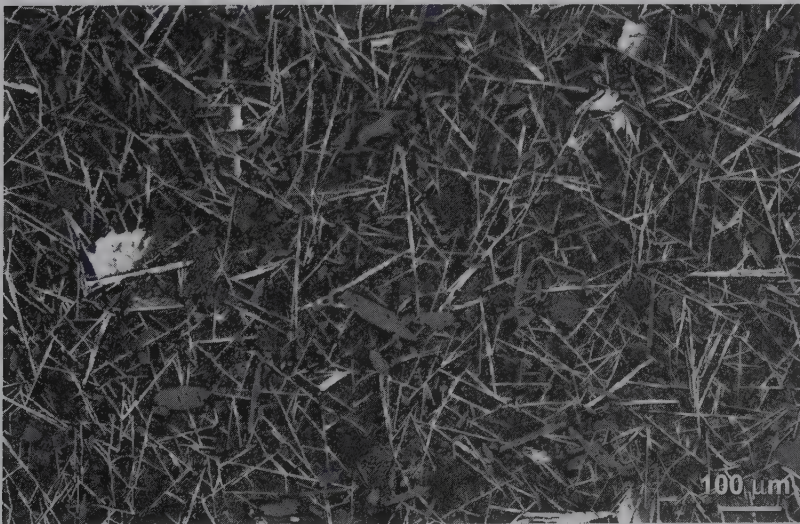
FIG. 13.28 Photomicrograph taken in reflected light of a polished section of minerals from the Salton Sea geothermal field, California, USA. The minerals are: chalcopyrite, white clumps; hematite, white acicular crystals; anhydrite, gray crystals; chlorite, dark gray matrix. Here, the spatial distribution of minerals is easily observed. (Photograph by B. Dutrow.)
