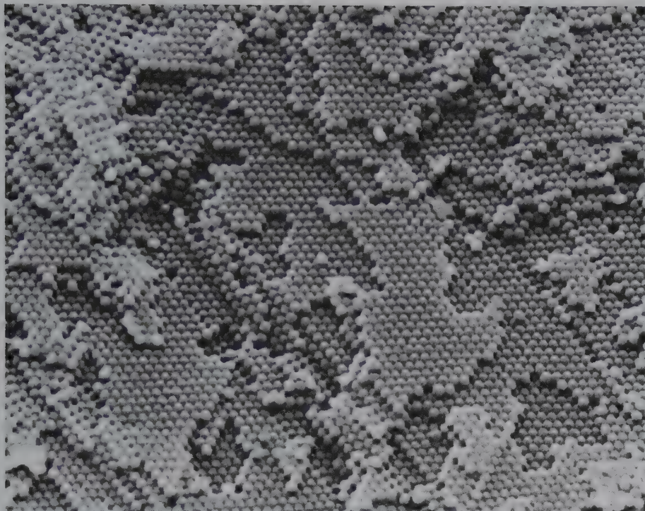
FIG. 2.6 Scanning electron micrograph of an opal with chalky appearance, showing hexagonal closest packing of silica spheres (diameter of spheres is approximately 3,000 \text{ \AA} ). Because of weak bonding between the spheres, they are completely intact; in typical precious opal samples, many of the spheres are cleaved. (Courtesy of Darragh, P. J., A. J. Gaskin, and J. V. Sanders. 1976. Opals. Scientific American 234, no. 4: 84–95.)
