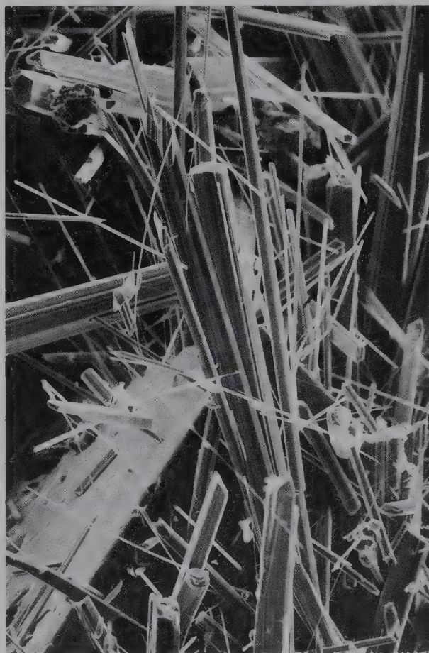
FIG. 14.23 Scanning electron microscope (SEM) photograph, using secondary electrons, of fibrous hollandite, \text{BaMn}_8\text{O}_{16} . (Photograph courtesy of M. Spilde, Institute of Meteoritics, University of New Mexico, Albuquerque.)
