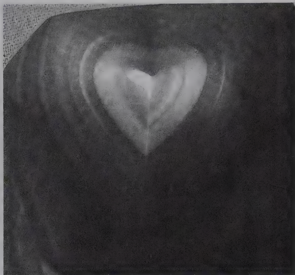
FIG. 2.8 Play of colors in rainbow obsidian (volcanic glass) caused by parallel alignment of very fine, needlelike rutile, \text{TiO}_2 , inclusions. The specimen has been polished to highlight the concentric color bands. Field of view \sim 5 cm. (Photograph from B. Dutrow.)
