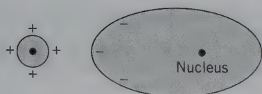
FIG. 3.10 Polarization effect of a small, highly charged cation on a large anion.
