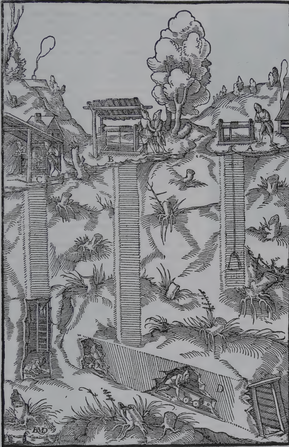
FIG. 1.10 An illustration from Agricola, De Re Metallica (1556) shows ore mined underground, moved through horizontal tunnels, and hoisted through vertical shafts. (From Agricola, De Re Metallica , translated into English. Published in 1950 by Dover Publications, Inc., New York.)
