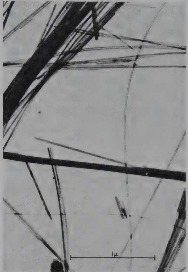
FIG. 18.38 Electron micrograph showing tubular fibers of chrysotile from Globe, Arizona. Magnification 35,000 \times . (After Hagy, B. and G. T. Gaust. 1956. Serpentine: Natural mixtures of chrysotile and antigorite. American Mineralogist 41: 817–38.)
