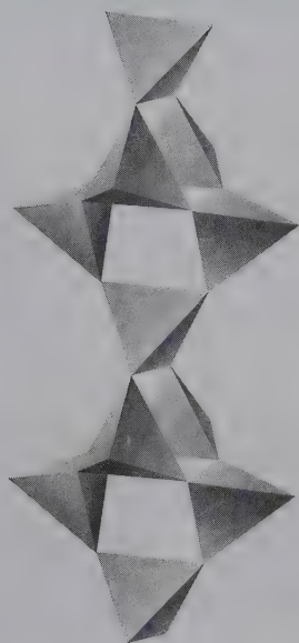
FIG. A (c) Tetrahedral linkage in zeolites (1977)
