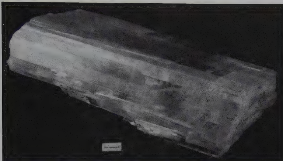
FIG. 17.32 Kernite showing typically excellent {100} and {001} cleavage. Scale = 1 cm. From Boron, Kern County, California.
