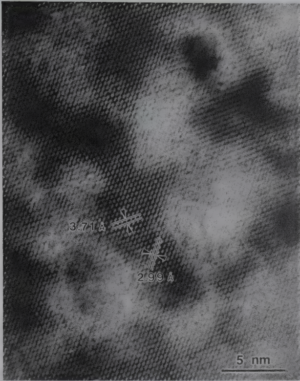
FIG. 12.21 High-resolution transmission electron microscope (HRTEM) structural image of radiation-induced metamict domains inside a well-crystallized host of olivine, (\text{Mg, Fe})_2\text{SiO}_4 . The damage was artificially produced by subjecting the original olivine crystal to a high-kilovoltage ion beam. Scale bar is in nanometers (nm): 1 \text{ nm} = 10 \text{ \AA} . (From Wang, L. M., M. L. Miller, and R. C. Ewing. 1991. High-resolution TEM observation of displacement cascades in krypton-irradiated silicate minerals. Proceedings of the 49th Annual Meeting of the Electron Microscopy Society of America , EMSA, 910–11).
