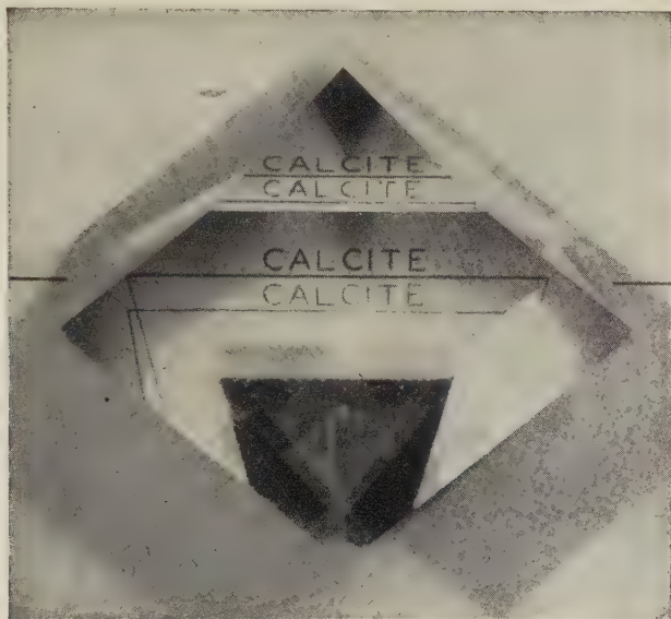
Fig. 369. Calcite, Viewed Normal to the Rhombohedron Face Showing Double Refraction. The double repetition of "calcite" at the top of the photograph is seen through a face cut on the specimen parallel to the base.
