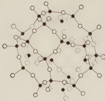
Fig. 601. Three-Dimensional Linkage. (From Harry Berman, "Constitution and Classification of the Natural Silicates," Am. Min. , 1937.)
