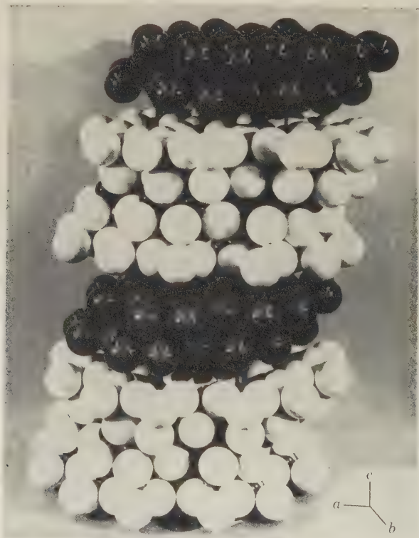
Fig. 594. Chlorite, Mg_3Si_4O_{10}(OH)_2 \cdot Mg_3(OH)_6 , Packing Model. O white, (OH) large black, Mg small black; c axis vertical. The model shows "t-o-t" sheets alternating with "o" sheets. Fe II , Fe III and Al may substitute for Mg and Al for Si.
