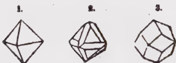
Fig. 1. The primary, the regular octahedron. Fig. 2. The same with the edges replaced, and by an enlargement of these planes the rhombic dodecahedron is formed, as in Fig. 3.
