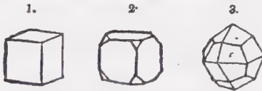
Fig. 1. The primary cube. Fig. 2. The same of which each solid angle is truncated or replaced by three planes. Fig. 3. The secondary plane of fig. 2, complete. The trapezoidal planes incline on the primary 144^{\circ} 44' and on each other at angles of 146^{\circ} 26' .
