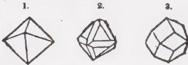
Fig. 1. The regular octahedron, which is the primary form. Fig. 2. Edges of the octahedron replaced. Fig. 3. Rhombic dodecahedron.
