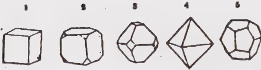
Fig. 1. The primary; a cube. Fig. 2. Cube of which the solid angles are replaced by triangular planes. Fig. 3. These planes are so increased as to reduce the primary planes to small cubes or squares. In Fig. 4. the primary planes entirely disappear, producing the regular octahedron. Fig. 5. Is a pentagonal dodecahedron formed by a replacement of the edges of the cube, by irregular six-sided planes, alternately in different directions.
