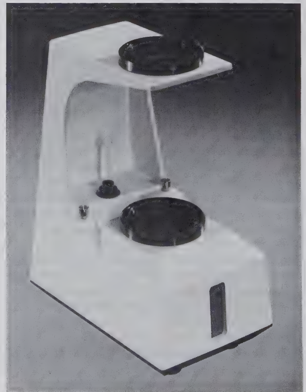
FIG. 15.5. Polariscopes used for distinguishing isotropic from anisotropic materials, determining pleochroism, and obtaining interference figures. (Courtesy of Gemological Institute of America, GEM Instruments Corp., Santa Monica, Calif.)
