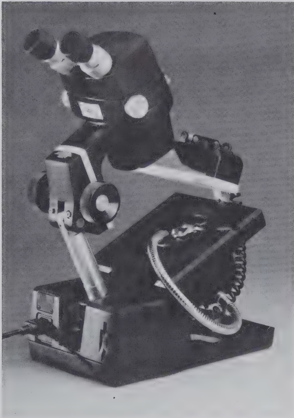
FIG. 15.4. A low-power stereoscopic wide-field microscope, designed to provide several different methods for illuminating gemstones. (Courtesy of Gemological Institute of America, GEM Instruments Corp., Santa Monica, Calif.)
