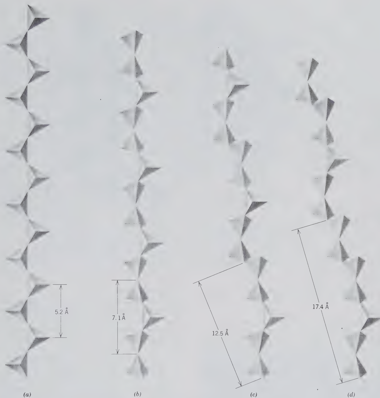
FIG. 13.59. \text{SiO}_3 chains in pyroxene (a) and pyroxenoids. (b) Wollastonite. (c) Rhodonite. (d) Pyroxmangite. (After Liebau, F., 1959, Über die Kristallstruktur des Pyroxmangits (Mn, Fe, Ca, Mg) \text{SiO}_3 , Acta Crystallographica , v. 12, pp. 177–181.)
