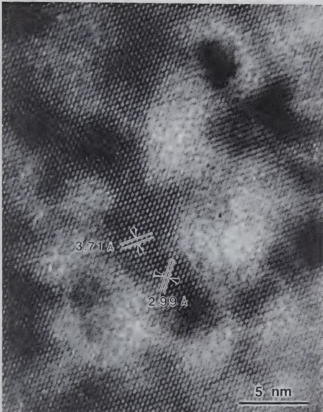
FIG. 3.48. High-resolution transmission electron microscopic (HRTEM) structural image of radiation-induced metamict domains inside a well-crystallized host of olivine ( (\text{Mg}, \text{Fe})_2\text{SiO}_4 ). The damage was artificially produced by subjecting the original olivine crystal to a high-kilovoltage ion beam. Scale bar is in nanometers (nm): 1 \text{ nm} = 10 \text{ angstroms} . (From Wang, L. M., Miller, M. L., and Ewing, R. C., 1991, High-resolution TEM observation of displacement cascades in krypton-irradiated silicate minerals, in Proceedings of the 49th Annual Meeting of the Electron Microscopy Society of America, EMSA , pp. 910–911).
