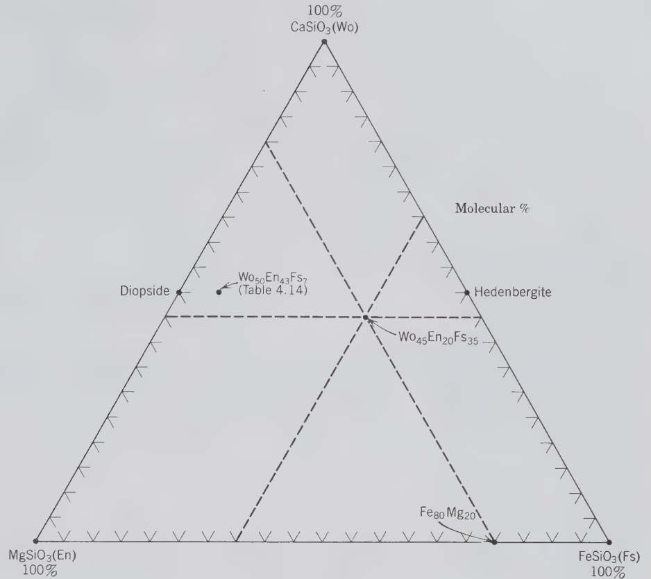
FIG. 5.25 Plotting of chemical compositions on triangular coordinate paper. The specific compositions represented are for the pyroxene family of silicates. See text for explanation of plotting procedure.
