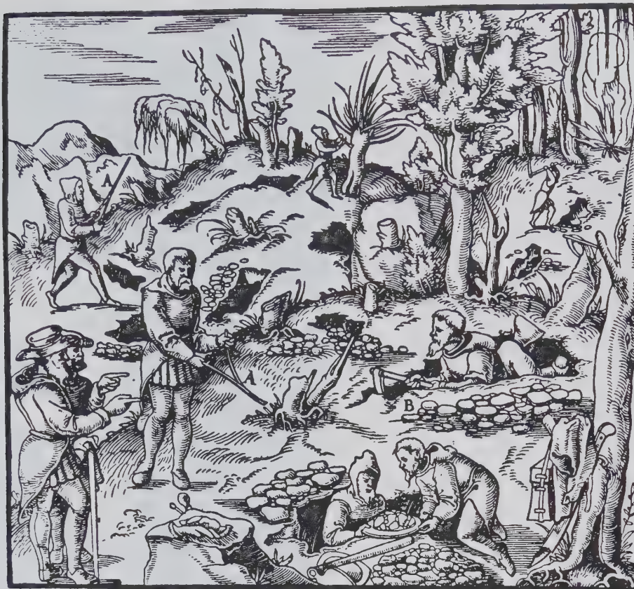
FIG. 1.1. Prospecting with a forked stick (A) and trenching (B) in the fifteenth century. (From Agricola, De Re Metallica , translated into English. Dover Publications, New York, 1950.)
