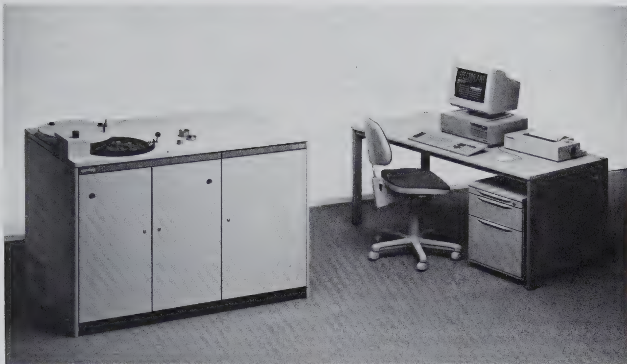
FIG. 5.10 The Siemens SRS 303 X-ray fluorescence spectrometer. The left-hand cabinet contains the X-ray source, X-ray spectrometer, and an automatic sample changer. The desk area, on the right, is the control and data handling center of the equipment. (Courtesy of Siemens Industrial Automation, Inc., Madison, Wis.)
