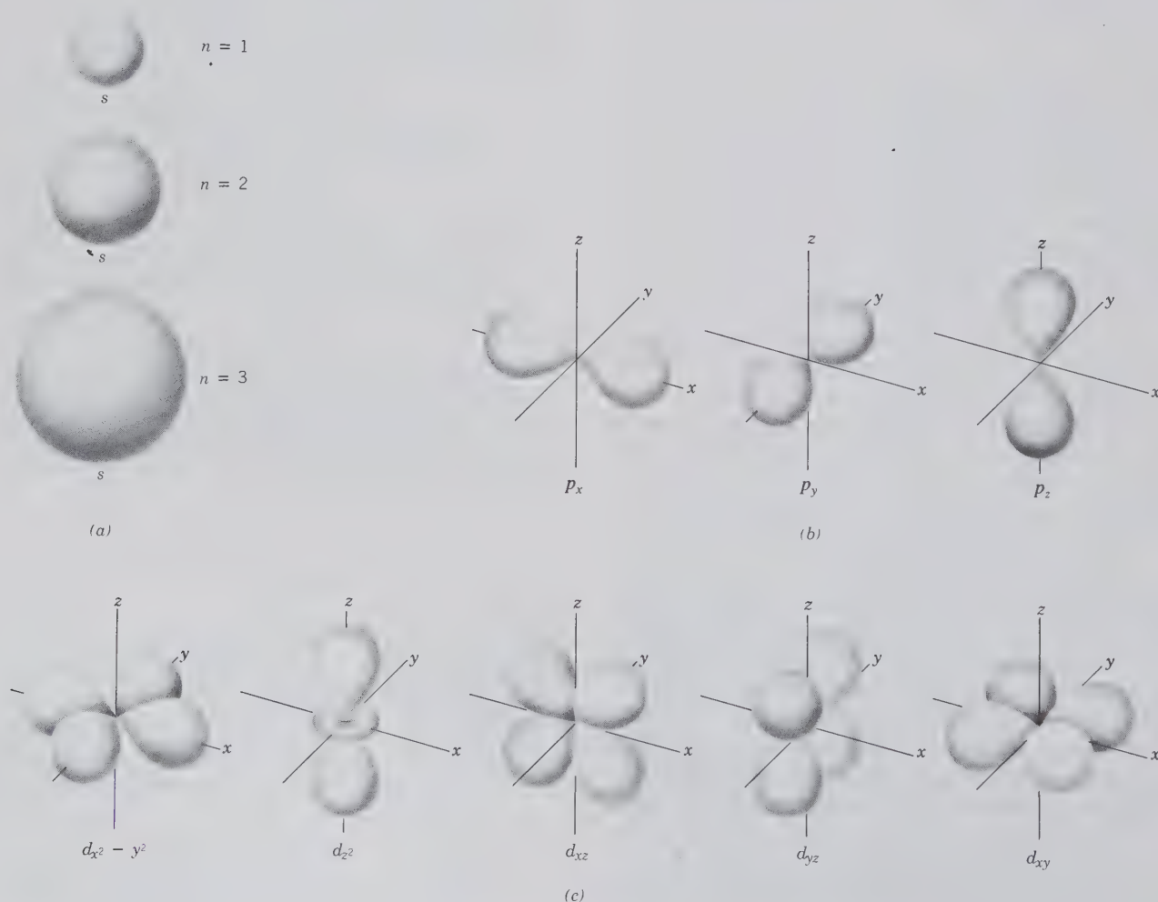
FIG. 4.10 Surfaces showing the angular dependence of the function \psi^2 for s , p , and d -orbitals of the hydrogen atom. These angular wave functions can be regarded as probability distributions of electrons.
