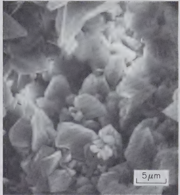
FIG. 11.36. Scanning electron micrograph of very small prismatic crystals of gibbsite (monoclinic) in bauxite from Surinam, South America. (Courtesy of H. H. Murray, Indiana University.)
