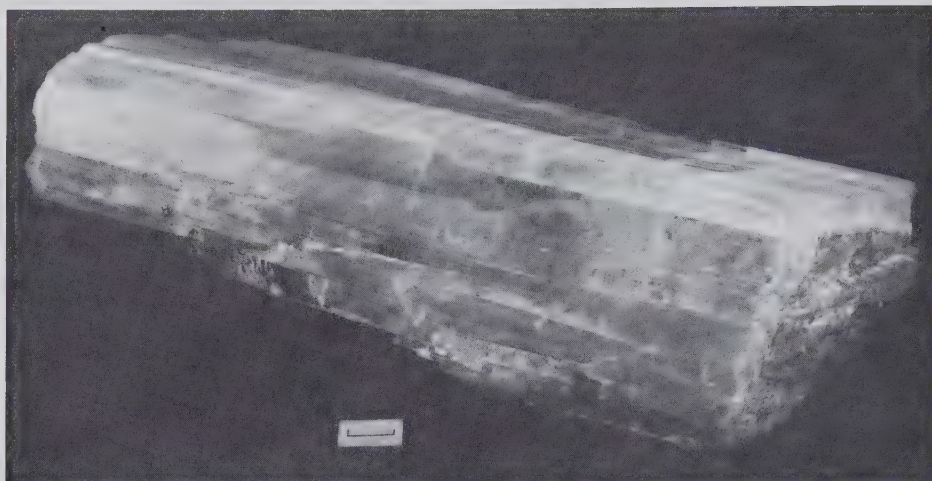
FIG. 12.24. Kernite showing typically excellent {100} and {001} cleavage. Scale = 1 cm. From Boron, Kern County, California.
