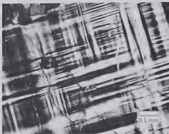
FIG. 2.114. Photomicrograph of transformation twinning (see p. 156) in microcline. The specimen is viewed under a microscope with crossed polarizers. The section of the photograph is approximately parallel to (001). The twin laws represented are albite with twin and composition plane (010), and pericline with twin axis direction [010].
