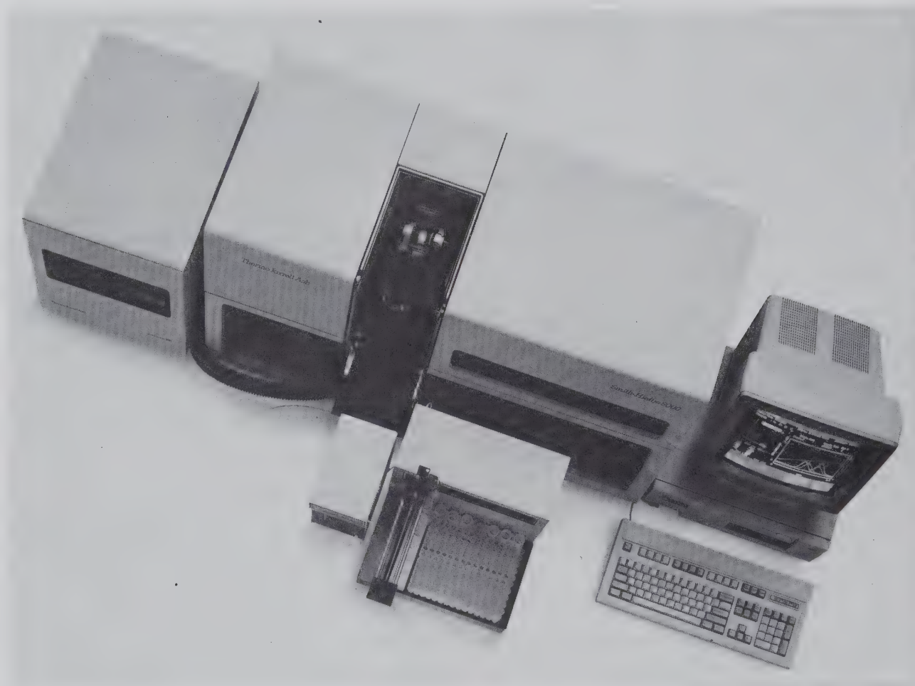
FIG. 5.5 Automated atomic absorption spectrometer. This specific instrument is the Smith-Hieftje 8000 Automatic AA Spectrophotometer. The hollow cathode lamp is at the left, the flame atomizer is in the center, and the spectrometer and automatic readout system are on the right. In the front of the instrument is an automated sample system by which 150 sample solutions can be analyzed automatically. (Courtesy of Thermo Jarrell Ash Corp., Franklin, Mass.)
