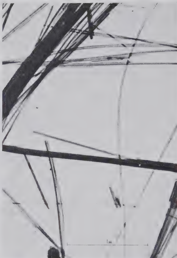
FIG. 13.88. Electron micrograph showing tubular fibers of chrysotile from Globe, Arizona, Magnification 35,000\times . (After Nagy, B., and Faust, G. T., 1956, Serpentines: natural mixtures of chrysotile and antigorite , American Mineralogist , v. 41, pp. 817-838.)
