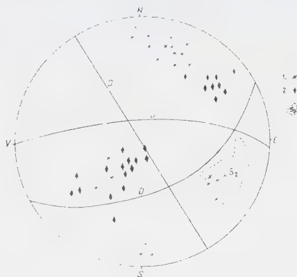
Fig. 2. Projection of poles of syenites veins directions (1), and lamprophyres (2), from Valea Mare and Güdutz fields as compared to the projection of the main fissure planes (D) and of foliation planes ( S_2 ) poles).
