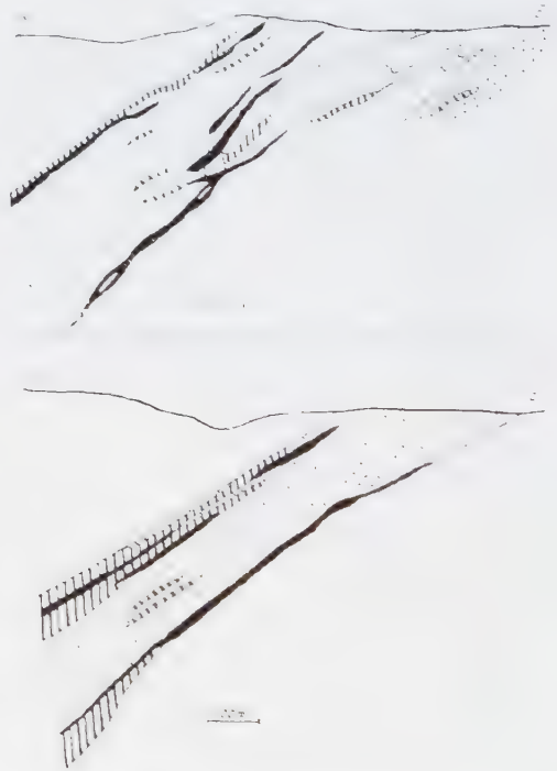
Fig. 2. W-E profile through the Stănăpări Plateau, based on the drill-hole data by I.P.E.G. Banatul: 1. Banatites weakly impregnated with sulfides 2. recrystallized limestones, 3. Garnet vesuvianite-bearing skarns, 4. Mineralization in skarns, 5. Mineralization in silicified banatites.
