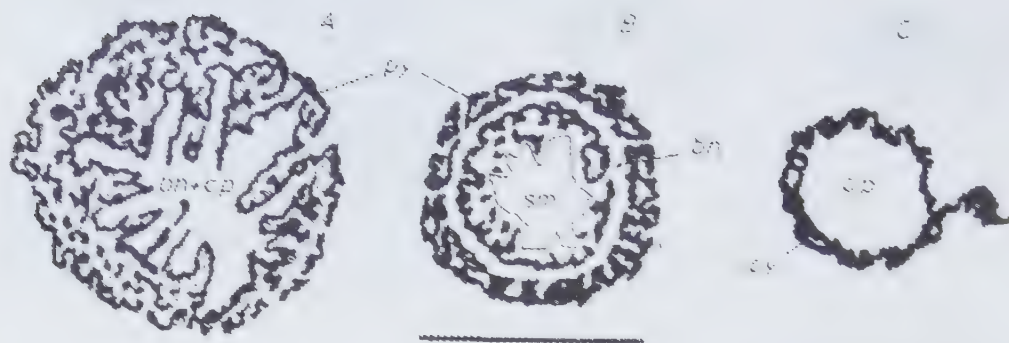
Fig. 8 A-C. Globular pyrite "grains" consisting of very fine pyrite micrograins (py) associated with secondary copper minerals. Inside the pyrite aggregate there is a mixture of bn+cp sometimes developed in flower-like pattern (A). Alternating bands of pyrite and bn with a nucleus of secondary copper minerals (sm) (B). Simple atoll- or shell-like pyrite grains in cp. Scale bar is 0.5 mm.
