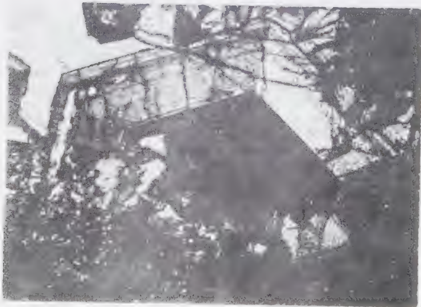
Fig. 1. Sectorial-type optical anomaly of garnets (Anton brook-Ciclova) N +, 250 x. Fig. 2. Concentric-type optical anomaly of garnets (Chinisea Valley) N +, 250 x.
