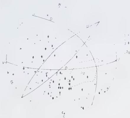
Fig. 1. Projection of poles of syenites veins direction. (1) porphyritic microsyenites; (2) lamprophyric microsyenites; (3) from Pietrari-Teascului and Jolotca vein fields as compared to the main fissure planes (D) and of foliation planes ( S_2 ) poles).
