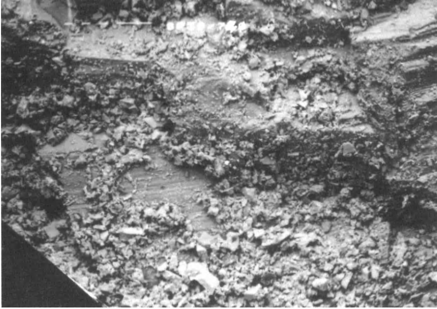
Fig. 6. Surface of coarse (1 cm) fluorite showing adherent coating of particles of magnetite up to 50\ \mu\text{m} diameter after treatment with fatty acid and diesel oil. The fluorite was recovered in the magnetic product of a rare-earth roll separator. Width of field of view = 1 mm.
