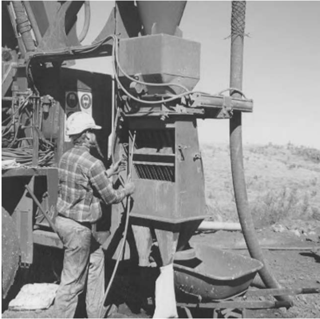
Fig. 1. Riffle divider underneath a cyclone for division of drill cuttings.
