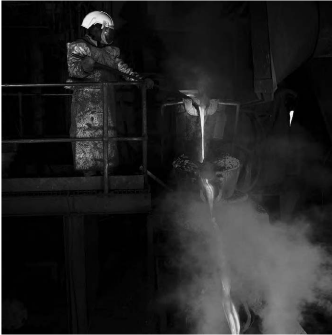
Fig. 12. Slag tapping from the arc furnace.
