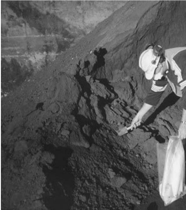
Fig. 8. Sampling from the side of a stockpile with a scoop will not provide a representative sample.
