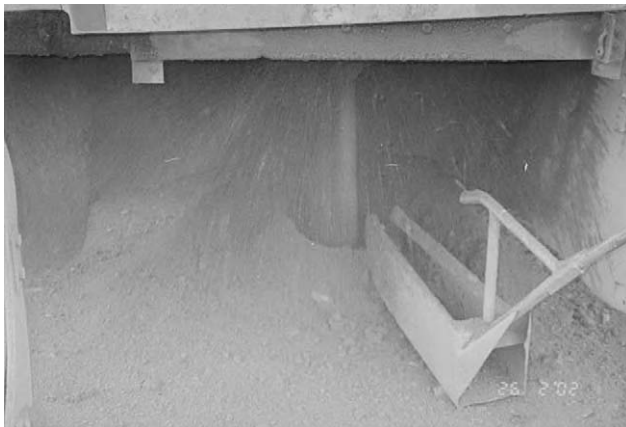
Fig. 3. Example of a manual sector cutter for sampling blast holes.
