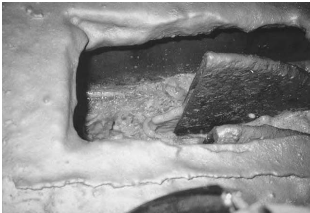
Fig. 6. Shark-fin cutters are unsatisfactory sampling devices, because they do not take a full cross-section of the slurry stream.
