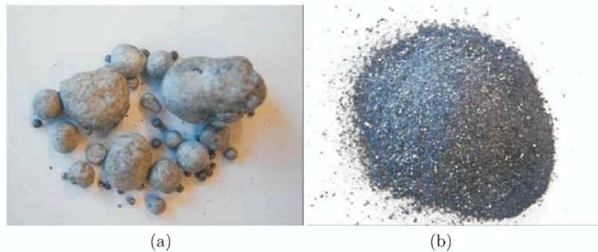
Figure 13.23: Hylite after melting, with (a) metal phase and (b) salt flux
