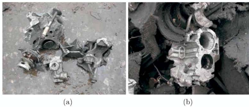
Figure 9.12: (a) Fragments of cylinder heads - cast aluminium and steel, valves - steel, and valve guide - copper; (b) Fragment of gear box housing - cast aluminium with steel bolts
