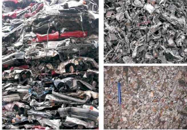
Figure 1.9: Diverse and distributed nature of the population of end-of-life vehicles in the Netherlands (2003) and an example of the grade of its recycling (intermediate) products
