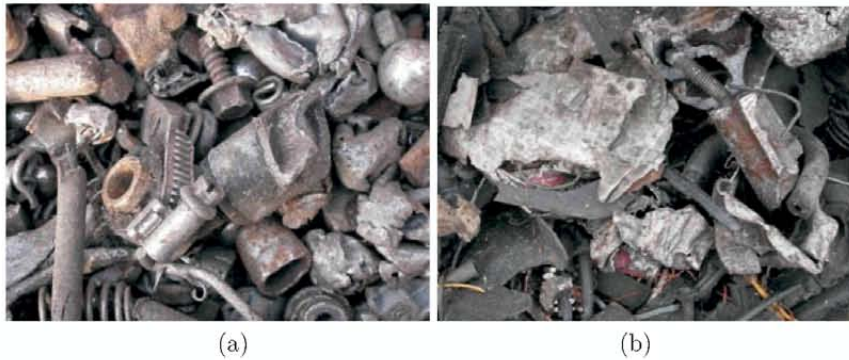
Figure 9.6: (a) Hose clamp (steel) with rubber hose and copper; (b) Fragment of engine block - cast aluminium and steel
