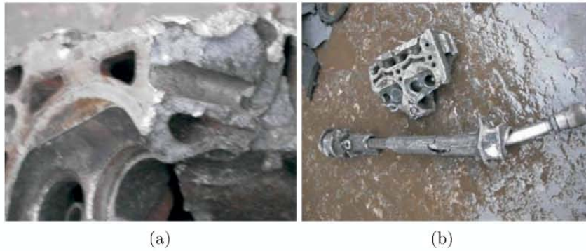
Figure 9.11: (a) Cylinder head - cast aluminium with steel insert; (b) 1 - Steering house - cast aluminium and steel, 2 - Cylinder head - cast aluminium and steel
