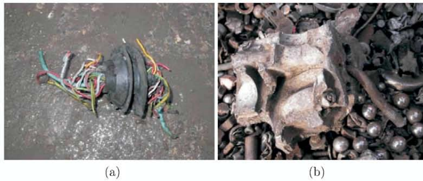
Figure 9.8: (a) Rubber with cable tree (copper and plastics); (b) Fragment of engine block - cast aluminium and steel bolts
