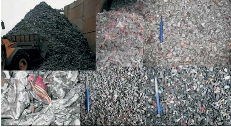
Figure 10.3: Diverse properties of recycling materials (in which clockwise: steel ca. 650 t. from 1153 ELV's; Cu fraction; Al/Mg/Cu/Zn fraction; plastic fraction; Al/Mg/Cu/Zn fraction; steel fraction)
