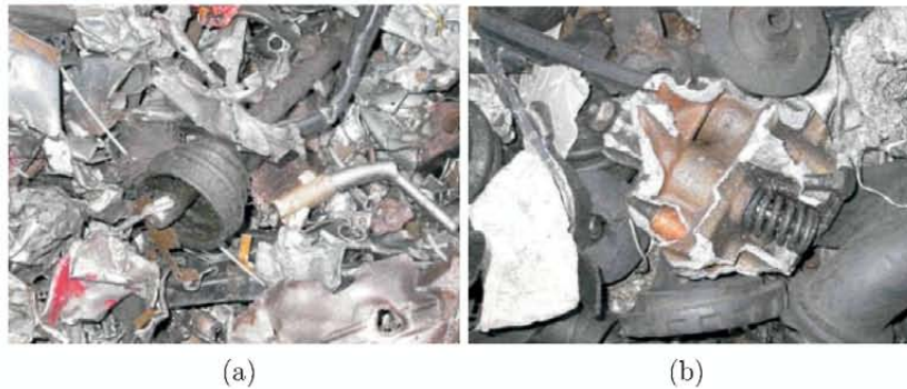
Figure 9.7: (a) Drive shaft - steel and rubber; (b) Fragment of cylinder head - cast aluminium, steel and copper (valve guide)
