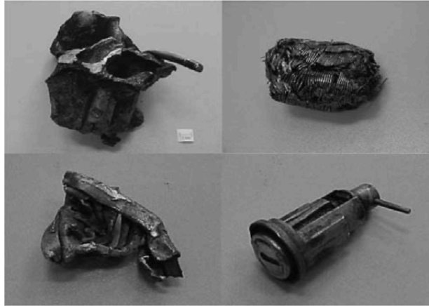
Figure 4.5: Limits of liberation processes: complex mechanically connected components [52]
