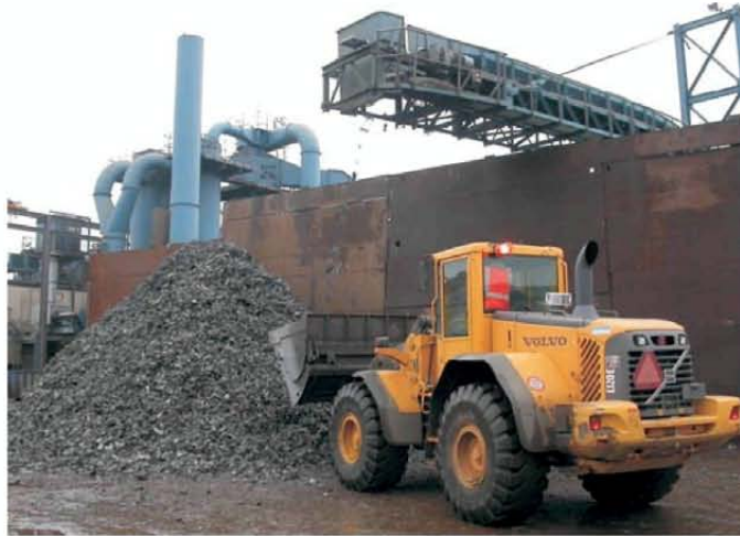
Figure 10.5: Weighing the ferrous sample by Volvo front-end-loader
