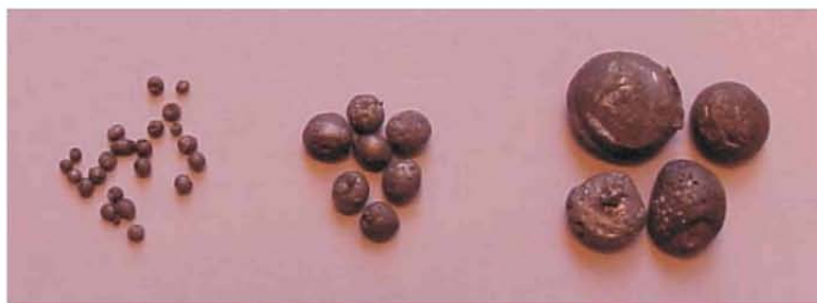
Figure 13.7: Aluminium droplets collected from a salt flux after melting
