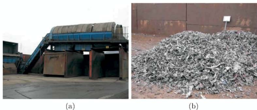
Figure 10.7: (a) Cleaned areas before each trail in this case for the drum screen and (b) labeling of all samples and streams with a consistent code (white sign post at back)
