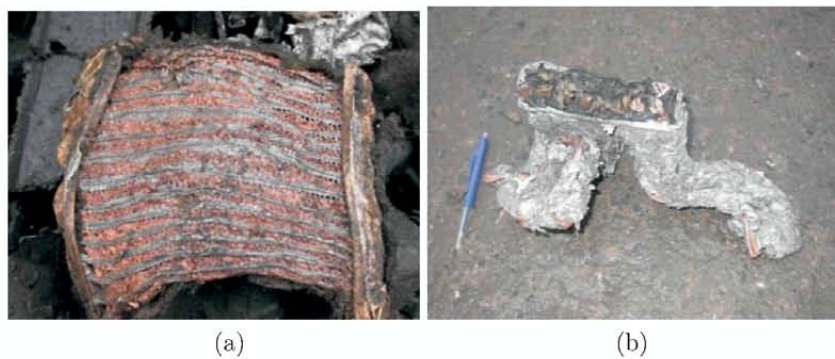
Figure 9.10: (a) Radiator - copper, brass, tin; (b) Radiator - copper, aluminium, plastics
