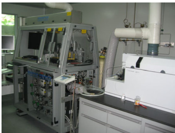
Fig. 2.15 The Agilent 7500a ICP-MS coupled with a Resonetics RESOLUTION M-50 laser ablation system
