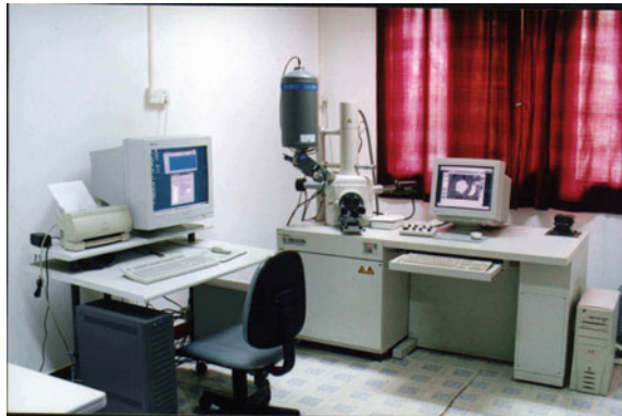
Fig. 2.3 The Hitachi S-3500 N scanning electron microscope with a Link ISIS 300 X-ray energy-dispersive spectrometer
