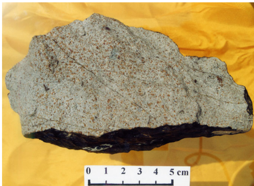
Fig. 1.4 A fragment of the Suizhou meteorite with thin shock melt veins
