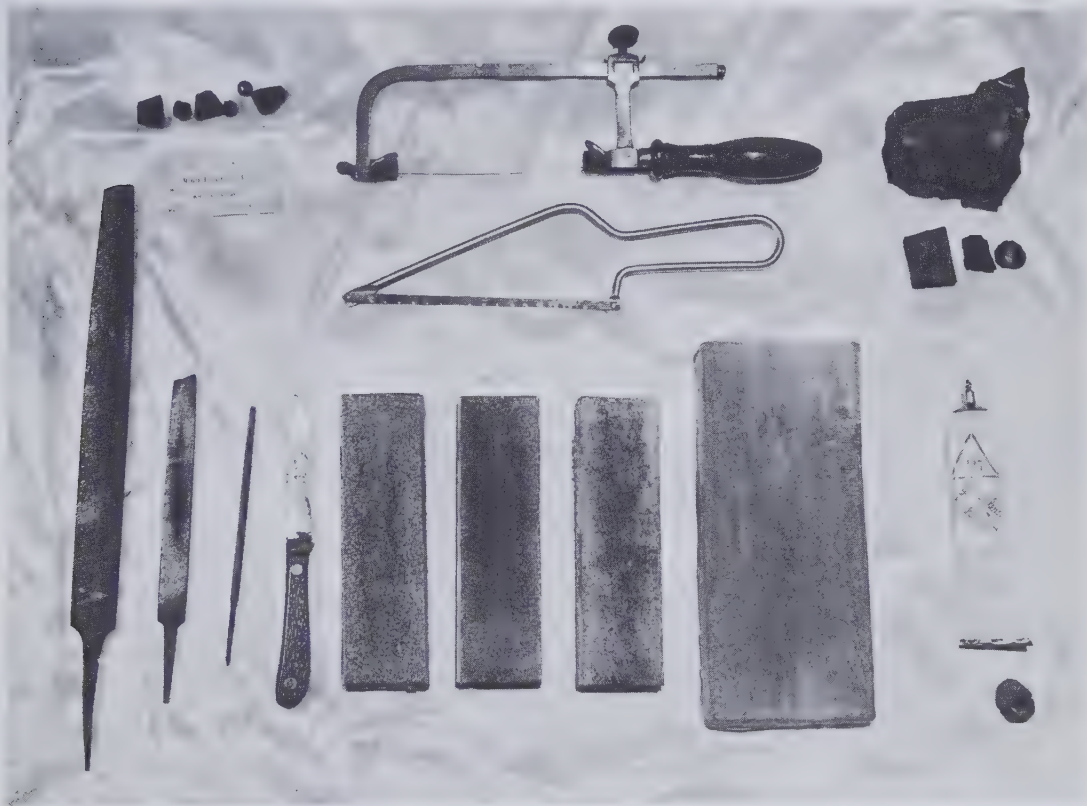
Fig. 182 Simple tools used for carving jet, coral, amber, and other very soft gem materials. Shown are several small saws, files, sanding blocks, and a polishing
