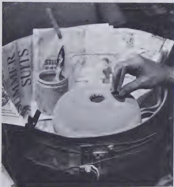
Fig. 91 A cabochon being polished on a felt buff. Note how the fingers support the gem from underneath.
