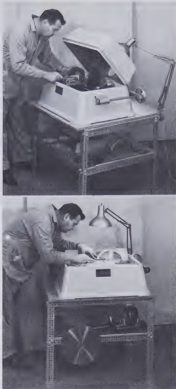
Fig. 15 Top. The Hillquist F10-14 slabbing-trimming saw in operation as a slabbing unit. The agate nodule shown is being adjusted in the clamp prior to engaging the automatic feed device. Bottom. The same unit converted to a trim saw. A slab of agate is now being sawn into smaller sections. Note the accessories on the shelf of the stand which make it possible to convert this unit from one type of saw into another. For slabbing, the saw uses a 14-inch blade; for trimming, a 10-inch blade is used. (Courtesy Lapidary Equipment Company, Inc., Seattle, Washington)
