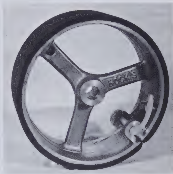
Fig. 48 Drum sander fitted with sponge rubber backing over which strip abrasive cloth is stretched. The ends of the cloth are placed in the slot at the lower right and tightened by the locking lever. (Courtesy Rock's Lapidary Equipment & Supplies, San Antonio, Texas)
