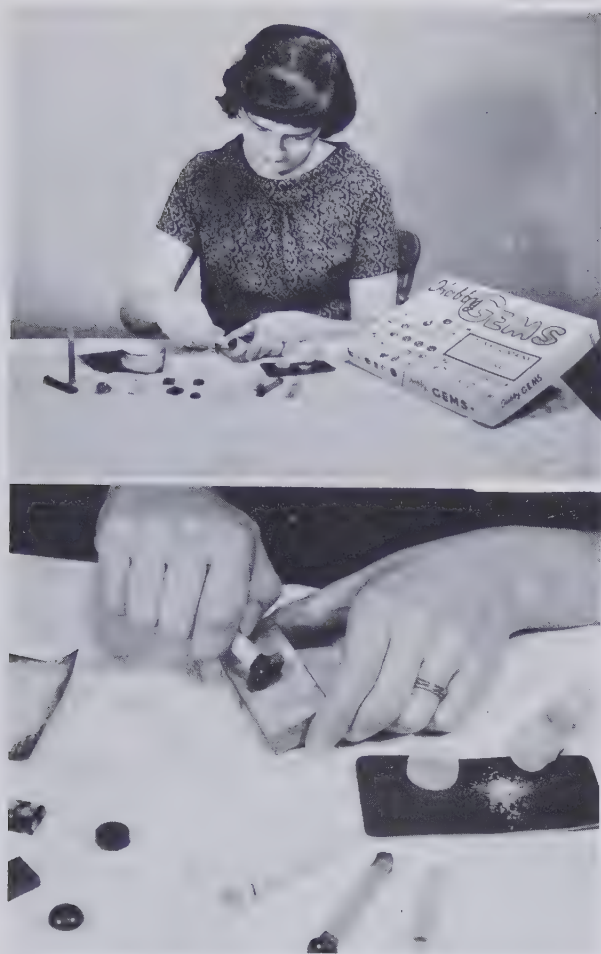
Fig. 93 Top. The Hobby Gems kit for making cabochons without machinery. Bottom. Close-up of grinding operation in which the gemstone is being given its rough shape. This inexpensive kit includes seven gemstone blanks, silicon carbide 80-grit shaping stone, sandpaper, and polishing pad of cowhide with cerium oxide as the polishing agent. Though patience is required, fine gems can be made. (Hobby Gems Co., Omaha, Nebraska)
