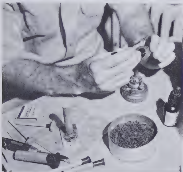
Fig. 87 Top . Shaping warm dopping wax about the base of a cabochon. Bottom . Making last-minute adjustments to be sure that the gem is square on the dopstick. Note dopping equipment, including warming oven at upper right, alcohol lamp, supply of dopping wax in foreground, and dopsticks waxed for attaching cabochons at lower left.
