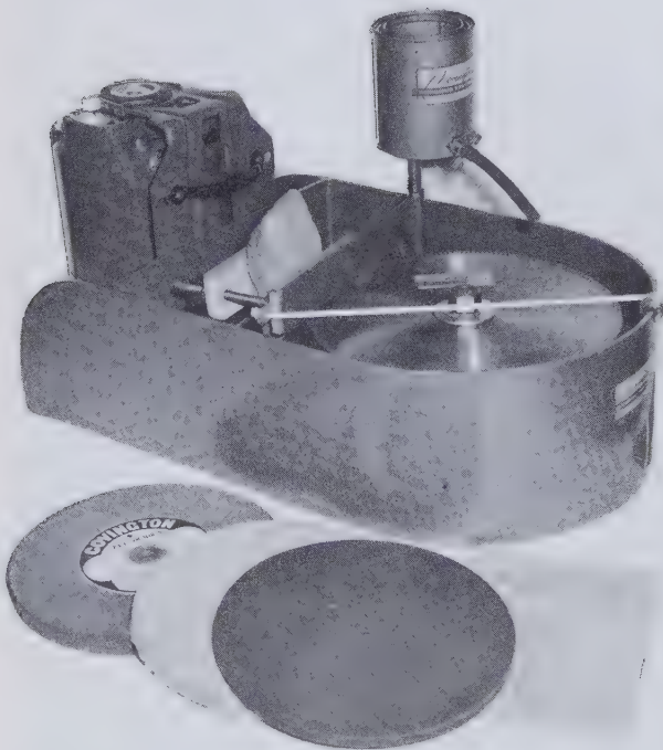
Fig. 63 Covington No. 301 horizontal all-purpose unit. The cord for pulling the rock into the saw blade is shown with a rock already placed in the clamp. As in the unit shown in Figure 62, the saw accessory is removable. (Courtesy Covington Engineering Corporation, Redlands, California)
