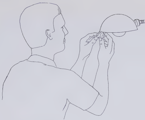
Fig. 99 Examining facet rough. The specimen is held at the edge of the light shade in such a way that the light shows flaws, cracks and inclusions. The eyes of the observer are above the lighted area in the shadow.
