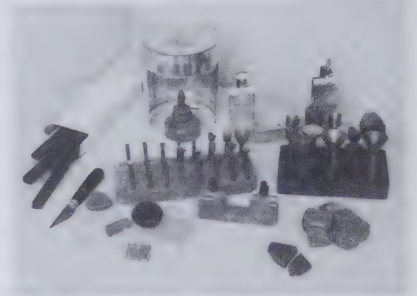
Fig. 143 Dopping accessories. Normal size dops are shown at center while jumbo dops and transfer jigs are shown at right.
