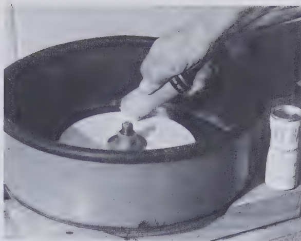
Fig. 53 Polishing agent in bar form. Cerium oxide is shown here being applied to a spinning polishing lap. The binder is water-soluble and allows the mixture to be washed off readily when necessary. (Courtesy Bruce Bars, Bruce Products Corp., Howell, Michigan)
