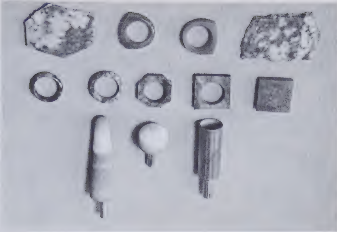
Fig. 169 Making a gemstone ring, showing steps and tools used to do the job. At the top are a hole saw for cutting out the centers, a reamer (right) for sizing the holes, and an abrasive ball point (center) for rounding
