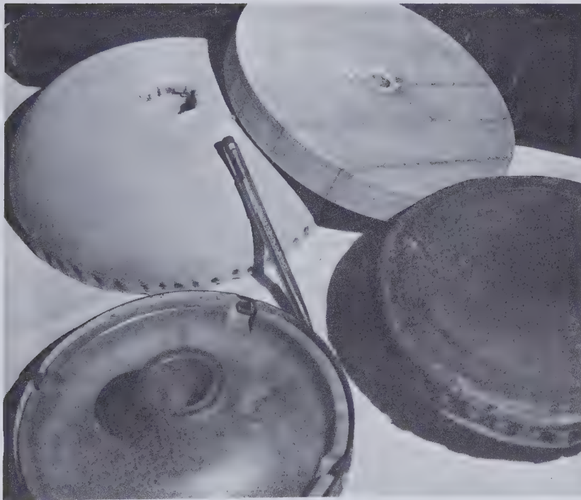
Fig. 65 Accessories for a vertical shaft all-purpose lapidary unit. Top left. Felt-covered polishing buff (see Figure 55). Top right. Poplar wood blank ready to be turned into a polisher for undercutting gems or
