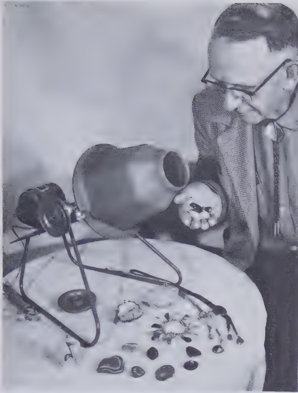
Fig. 154 The 7-lb. capacity Slik midget tumbler. The barrel is made of fiberglass with a liner of polyvinyl. The open-front design permits gases to escape and to inspect progress of work. Some tumbled gems are shown mounted and unmounted in jewelry. (Courtesy S. E. Landon Company, Joshua Tree, California)
