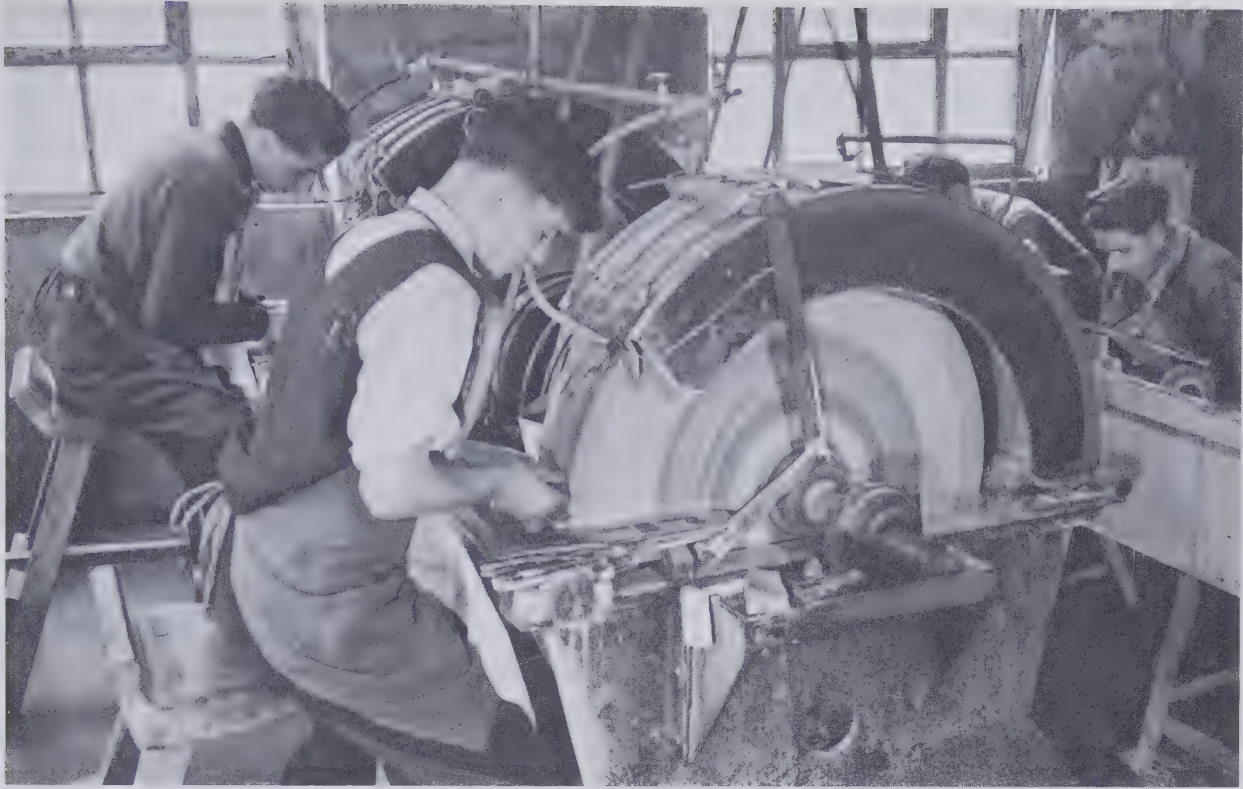
Fig. 38 Extremely large sandstone grinding wheels as used in some professional gem cutting shops in the cutting center of Idar-Oberstein in Germany. Such
