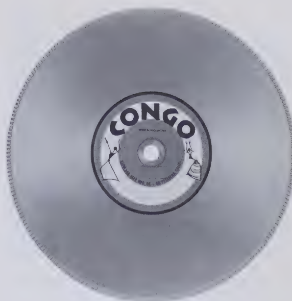
Fig. 10 Typical notched-rim diamond saw blade. In this type the notches are at right angles to the periphery of the blade and therefore this blade can be run in either direction. “Spacer” washers are provided at the arbor hole to accommodate different size shafting. (Courtesy Highland Park Manufacturing Company, South Pasadena, California)
