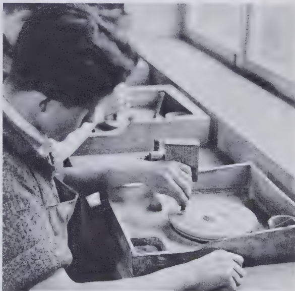
Fig. 102 Traditional "jamb peg" faceting in Idar Oberstein, Germany. The jamb peg board behind the hand is covered with small depressions in which the sharp end of the dop stick fits. The choice of hole, and of elevation angle, is done by eye while rotation angle is also controlled entirely by hand. (Courtesy Dr. Ing. W. Fischer, Rassmann Photo)
