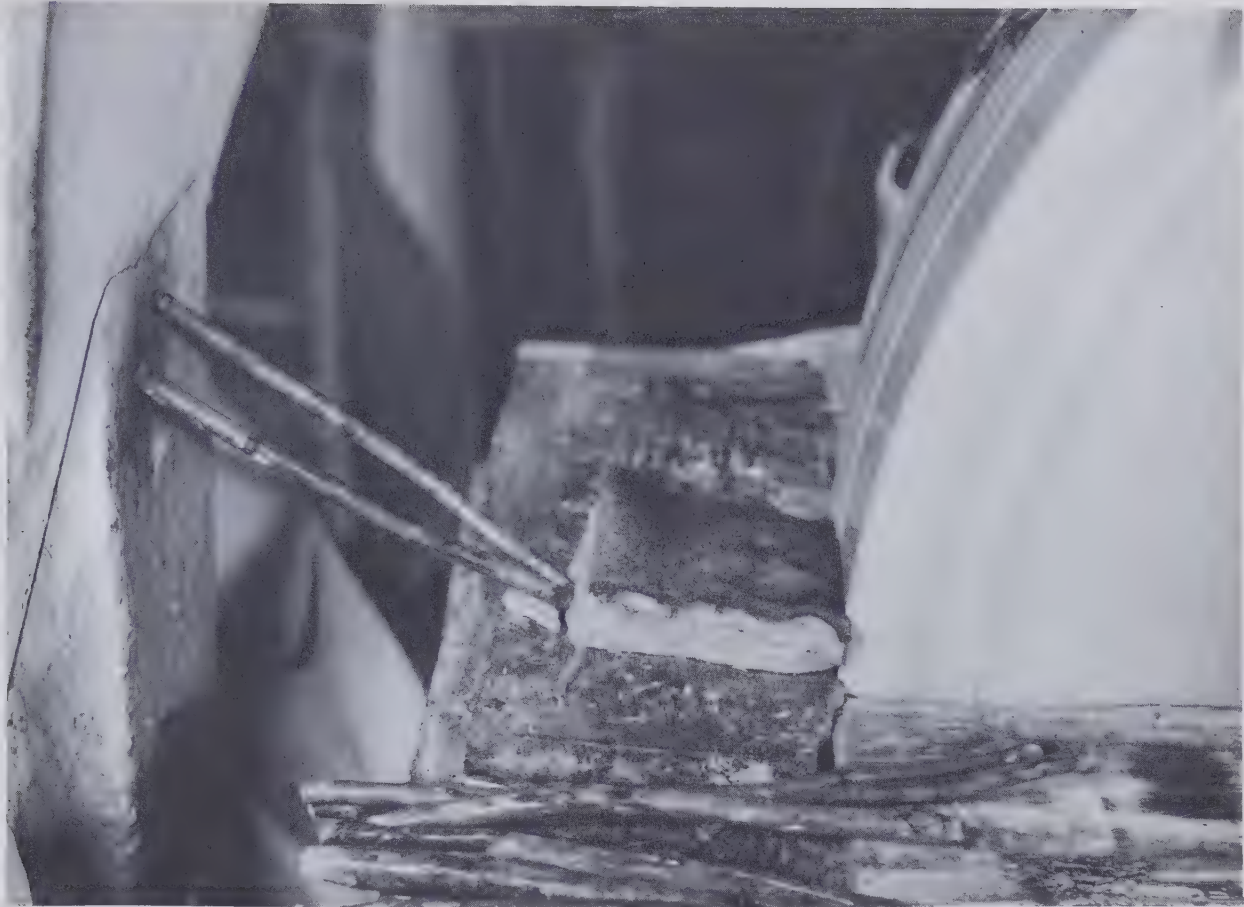
Fig. 35 Method of truing sandstone grinding wheels in Idar-Oberstein, Germany. Springy sticks are used to push a small piece of sandstone into the grinding
