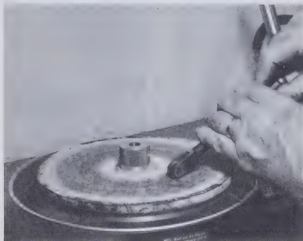
Fig. 115 Scoring a tin polishing lap using the M.D.R. hardened steel roller. (Courtesy M.D.R. Manufacturing Co., Inc., Los Angeles, California)
