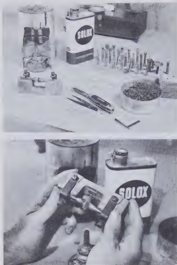
Fig. 127 Dopping equipment for faceted gems. Top. Tin can oven with alcohol lamp at upper left. Various dops in different shapes and sizes at upper right. Transfer block with gem being transferred at lower left. Also shown are preforms in center, dopping wax at lower right, and minor accessories. Bottom. Heating gem and dops to make the transfer.
