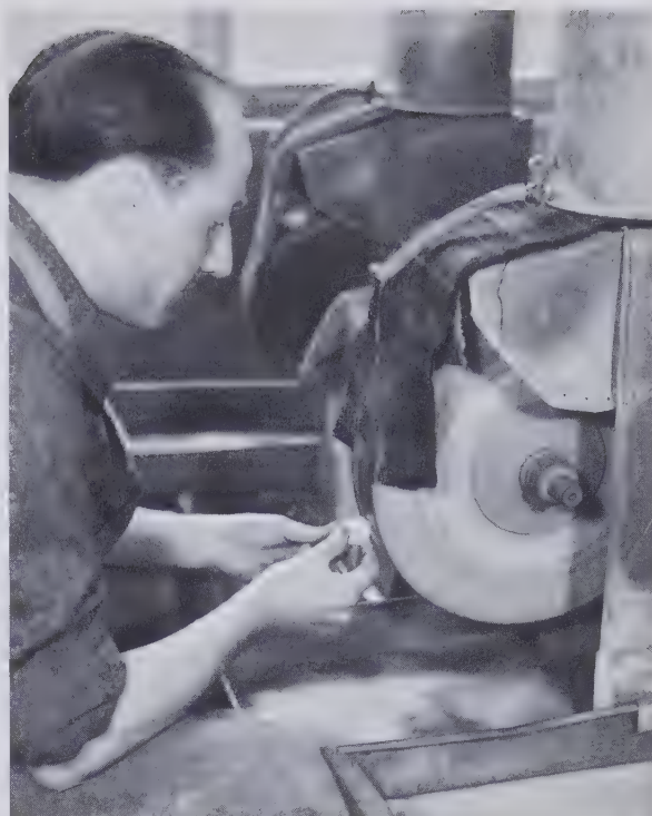
Fig. 31 Roughing out a gemstone using a large silicon carbide wheel. Note the position of the hands. Several folds of cloth above the wheel are used to spread water evenly over the face of the wheel; the water is supplied from a can above the wheel hood. Scene taken in a professional lapidary establishment in the famous German gem cutting center of Idar-Oberstein. (Courtesy W. Fischer; Rassmann Photo, Idar-Oberstein)
