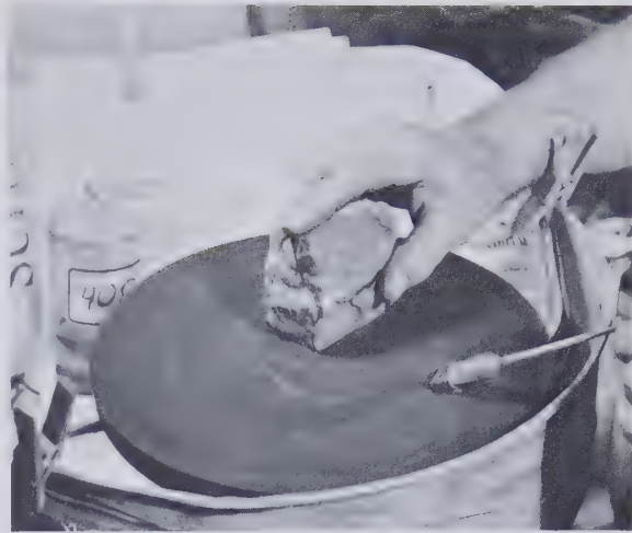
Fig. 41 The lapping process. The essentials are shown: a horizontal steel lap (stopped for clarity), glass jar with grit-water mix, and a brush for applying the mixture to the lap. The tub is lined with newspapers which will be discarded as soon as this stage of lapping is completed.
