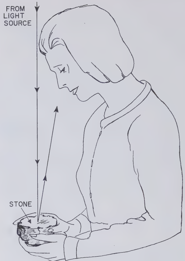
Fig. 78 Orienting feldspar under a light source. The light bulb should be directly overhead and the rays should pass as close to the forehead as possible. The stone is then turned about until the effect appears on top.
