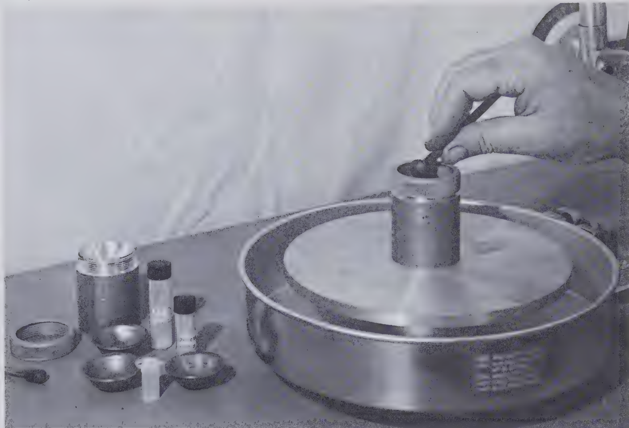
Fig. 92 Shaping hard cabochon star or catseye gems on special diamond-charged M.D.R. cups. An aluminum holder is attached to the lap unit of the M.D.R.
