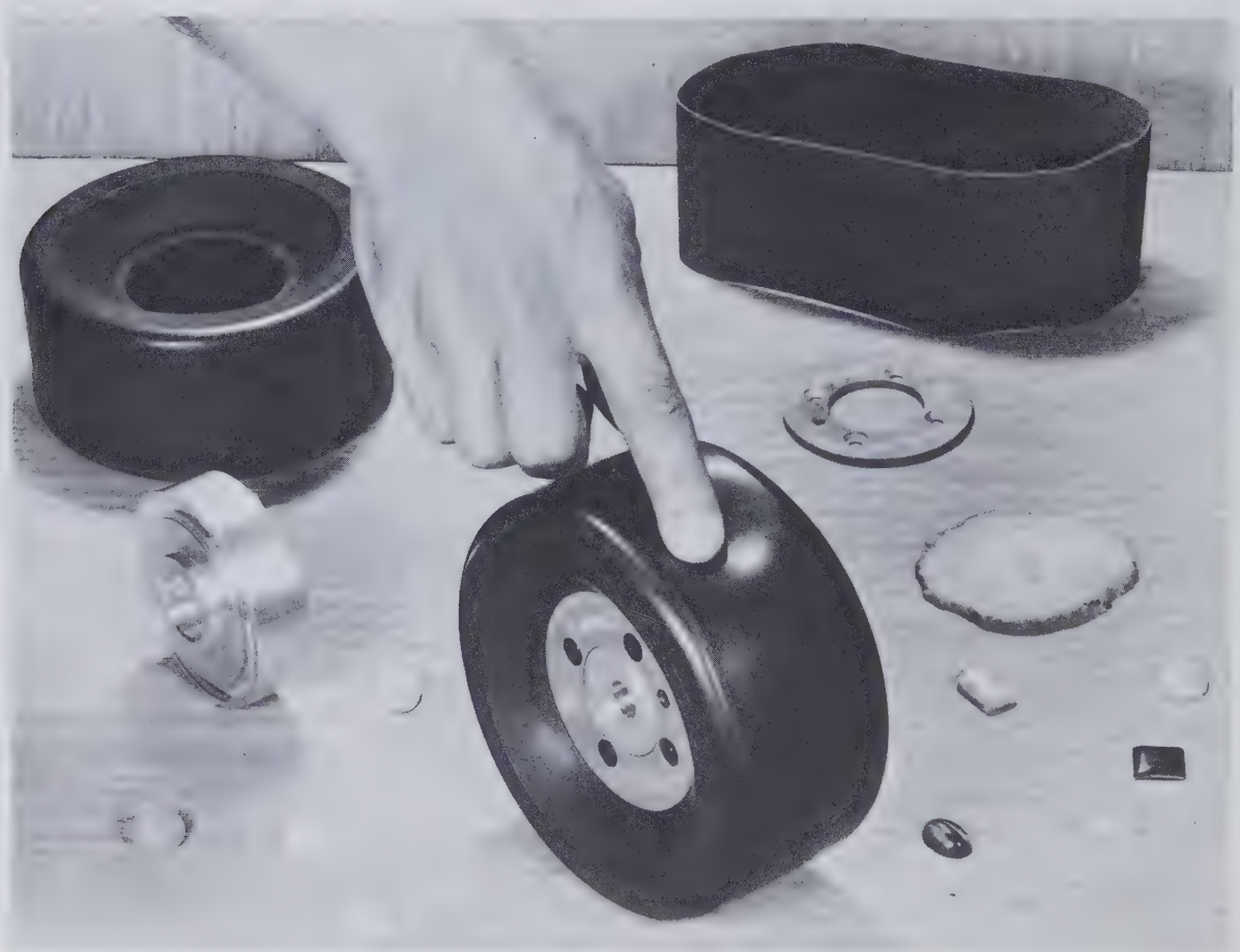
Fig. 49 A unique sanding drum inflated by air to any desired pressure. The endless cloth belt in the background is slipped on the deflated drum and held in place firmly when the latter is inflated. The surface
