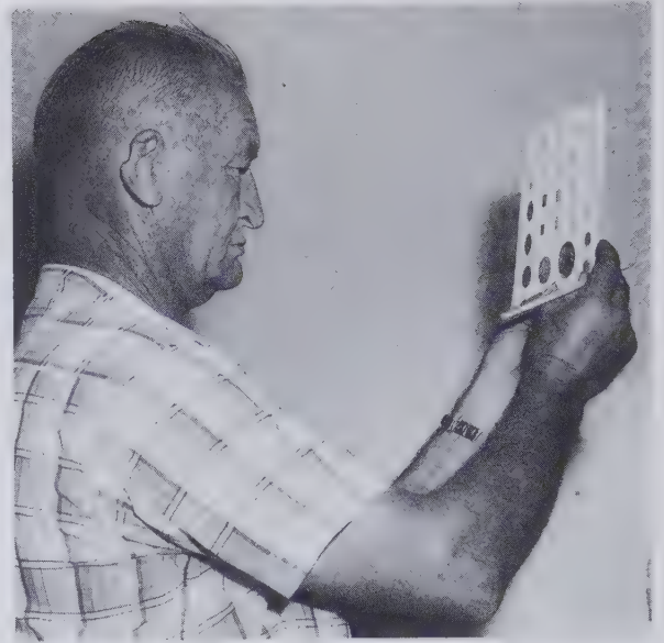
Fig. 81 Nick Potskoff of the Walt Disney Gem & Mineral Society shows how a template and a slab of gem material are held to select the best pattern for marking a cabochon. View in the society's shop on the studio lot. (Courtesy Circle C Walt Disney Productions)
