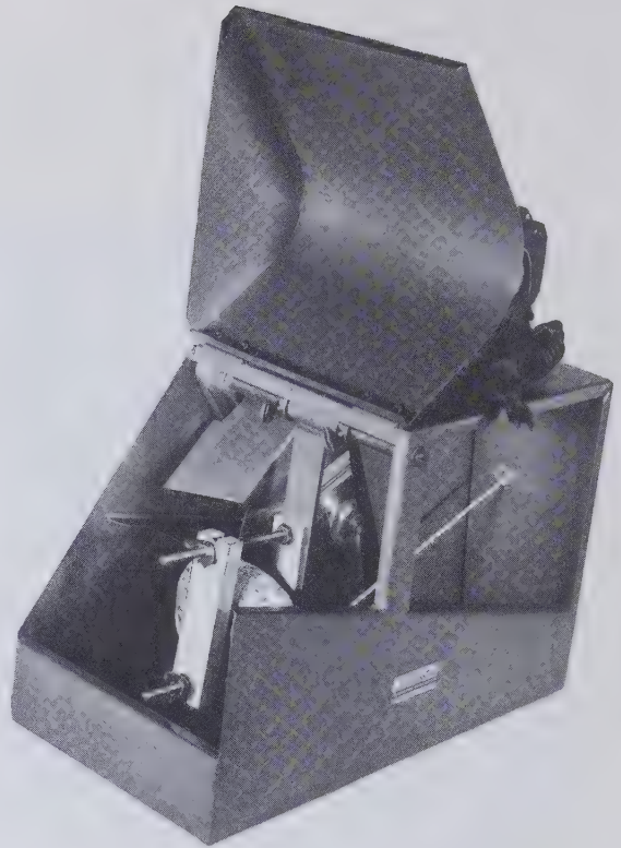
Fig. 14 Covington No. 106 portable combination slabbing and trimming saw. The unit is shown ready to slice a large nodule of rough material. The cord shown at the right leads to a weight which draws the stone into the blade during sawing. A conversion kit changes the saw into a trim saw. (Courtesy Covington Engineering Corporation, Redlands, California)
