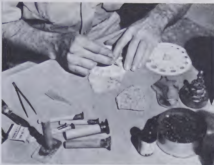
Fig. 82 Marking an oval stone using a plastic template and pointed piece of aluminum wire.
