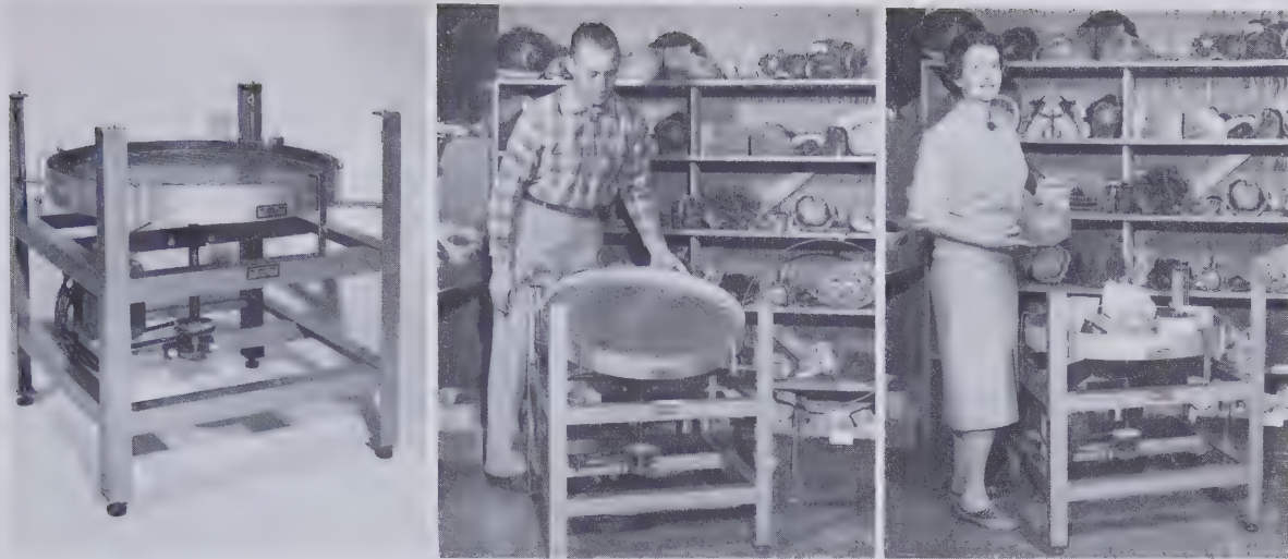
Fig. 43 The Vi-Bro-Lap automatic lapping machine. Left. Details of machine showing scored lap plate on top, drive shaft, supports, and motor. Center. Lap plate tilted up to show ease of removal and details of scored plate. Right. Lap plate loaded with stone sec-
