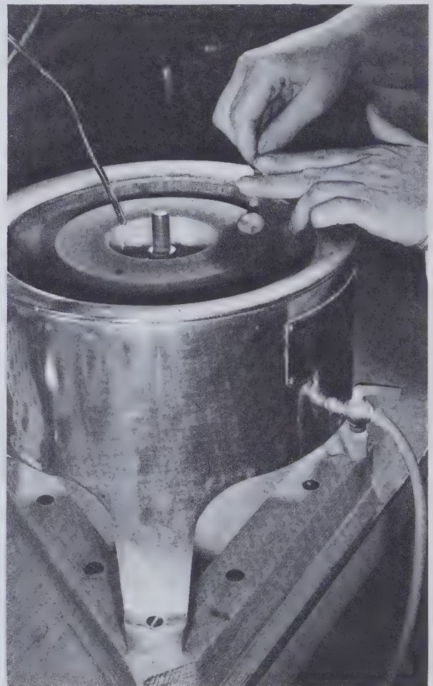
Fig. 64 Gemlap all-purpose unit being used to grind a cabochon. A special hollow-center grinding wheel is mounted upon the spindle. Note water supply. (Courtesy Brad's Rock Shop, Ferndale, Michigan)
