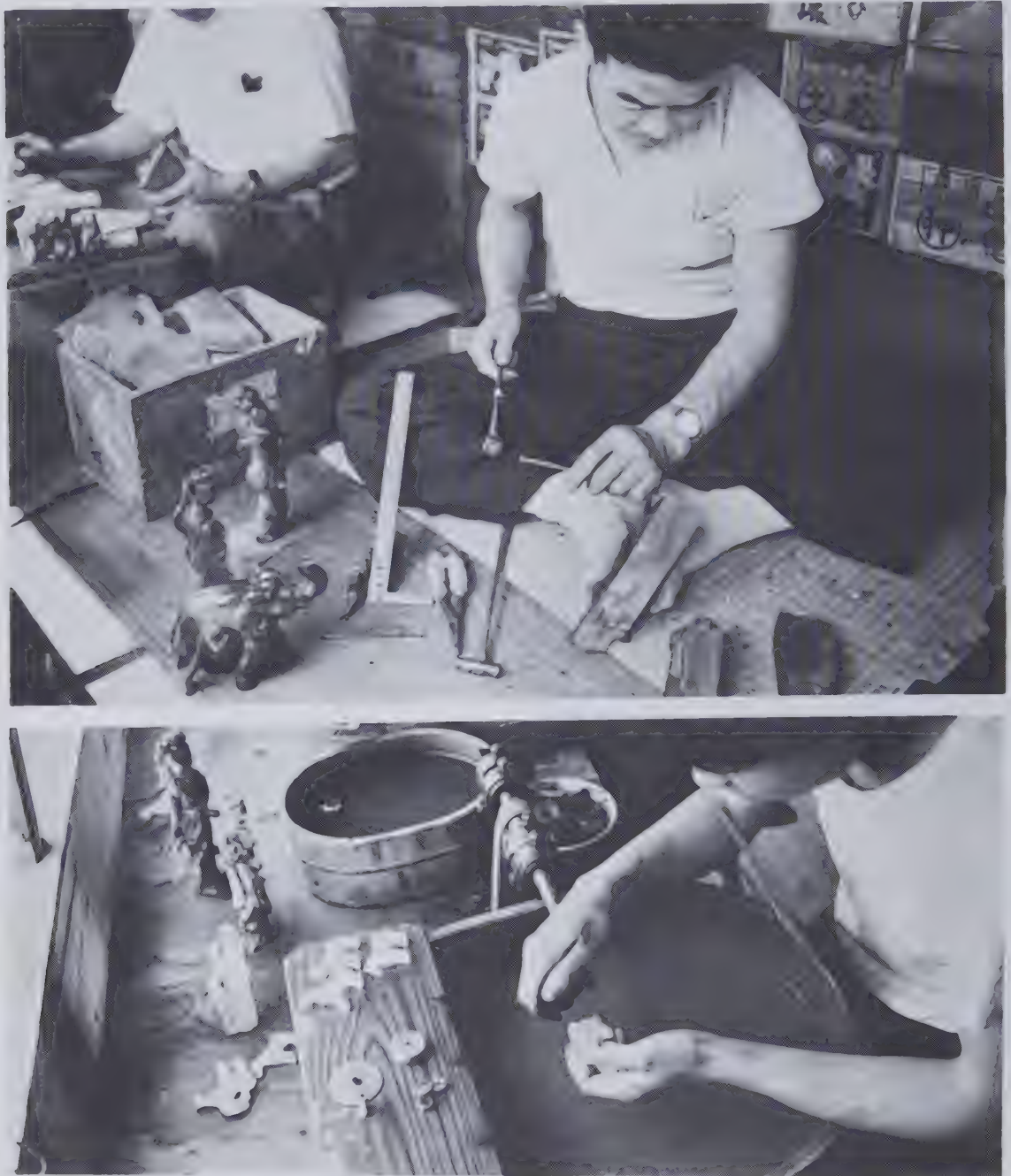
Fig. 164 Carvers at work in a cutting shop in the famous lapidary center of Kofu, Japan. Top. Much of the waste from a large block of agate meant for a carving is removed by carefully administered chiseling. A narrow steel rod is used as a blunt point chisel and is struck by the small hammer held in the right hand of the operator. Bottom. Carving with abrasive
