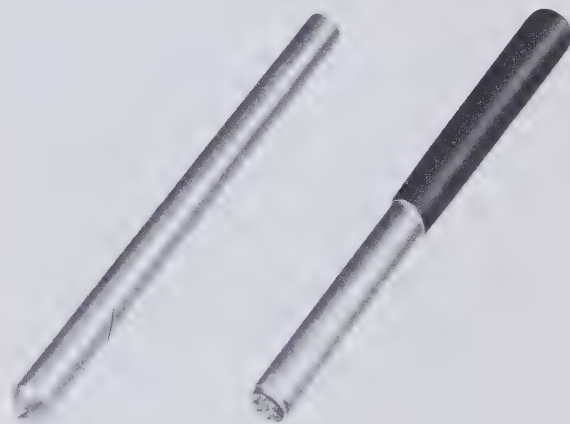
Fig. 33 Two types of diamond grinding wheel dressers. Left. A single point tool with a small industrial diamond protruding from the end. Right. A multiple-point tool containing seven separate diamond crystals. This tool dresses wheels faster and more smoothly but is also more expensive. (Courtesy Highland Park Mfg. Co., South Pasadena, California)
