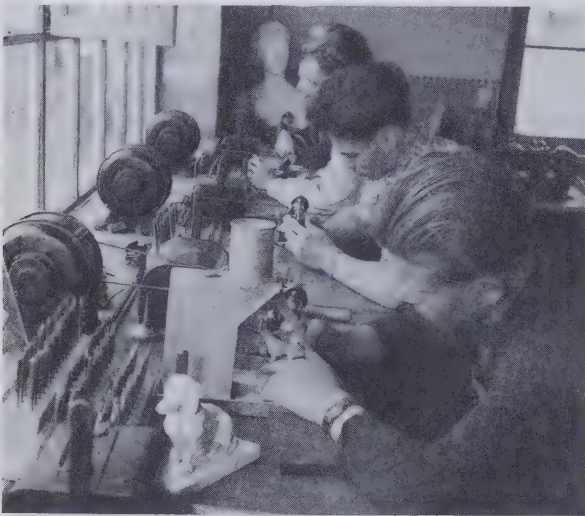
Fig. 159 Carving of gemstone figurines in a cutting establishment in Idar/Oberstein, Germany. Electric motors drive small arbors whose cutting points are interchangeable. Note the small tank over the arbor in the foreground which holds water for cooling and washing the cutting point. The dachshund model in the foreground is being copied in gem material. (Rassmann Photo, Idar/Oberstein, courtesy Walther Fischer)
