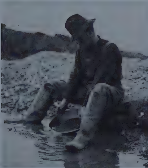
FIGURE 17. A "sourdough" demonstrating the final stages of gold-panning on Boulder Creek, Alaska. Only a handful of small gravel and sand now remains in the pan, plus whatever flakes and nuggets of gold have been concentrated. Courtesy U. S. Geological Survey.
