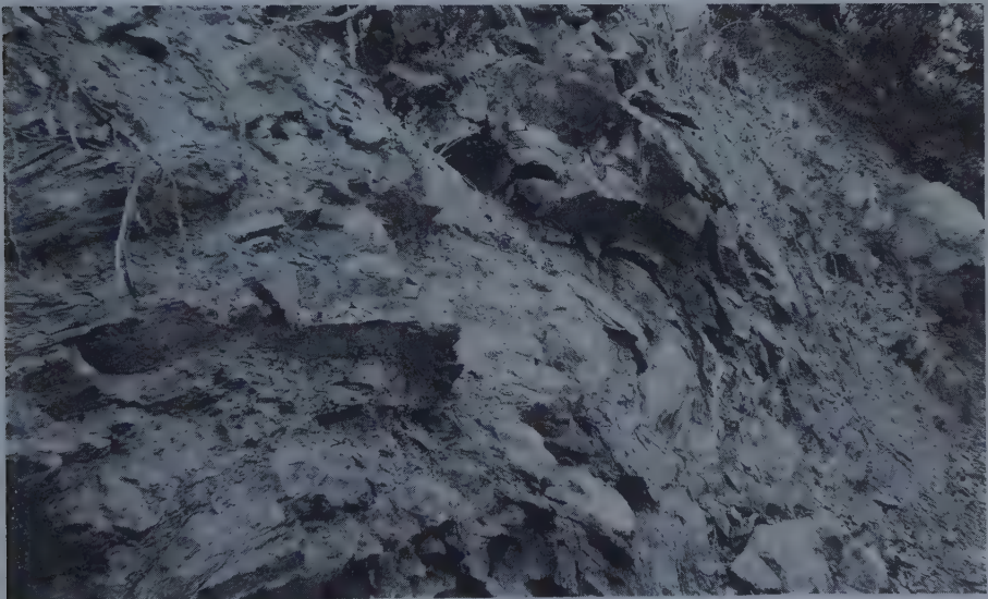
FIGURE 60. The ragged surface left by weathering and disintegration of schist is well illustrated here. In this view, taken along Kenton Road, Allegheny District, Sierra Co., California, a gentle fold is evident in the schist. Layering is also evident but is far more irregular than that noted in sedimentary rocks. Jagged, angular blocks are characteristic of fractured schist. Courtesy U. S. Geological Survey.
