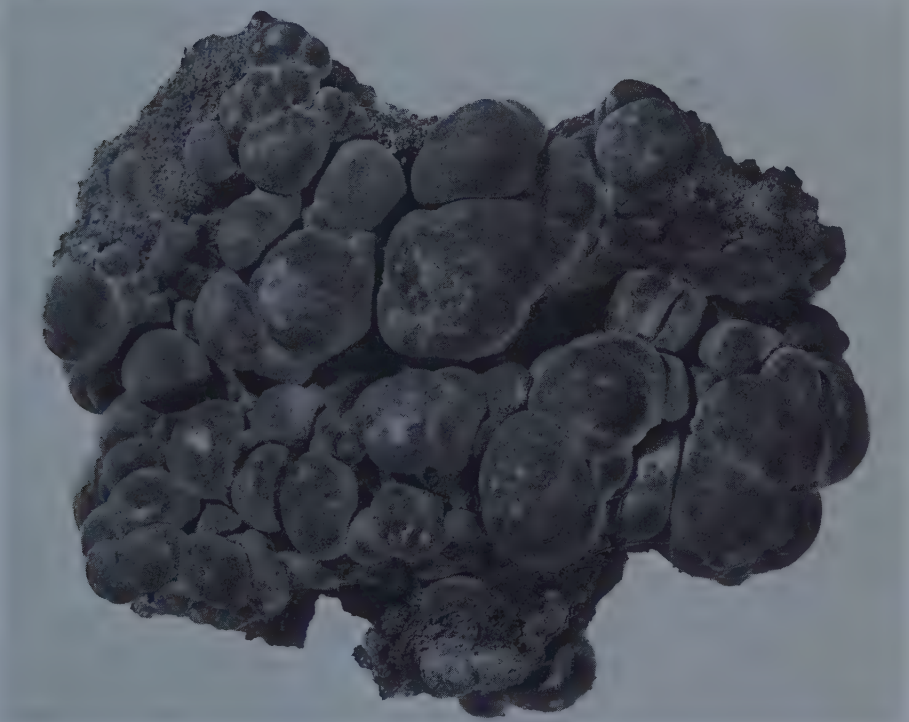
FIGURE 73. Malachite from Bisbee, Arizona. Each spherical growth consists of a multitude of needle-like crystals of malachite radiating outward from points upon the wall of a cavity in the oxidized zone. The featureless material upon which the malachite grew is porous limonite , usually of rich reddish-brown or brownish-yellow color. Specimen size 4 x 3 inches. Courtesy Smithsonian Institution.
