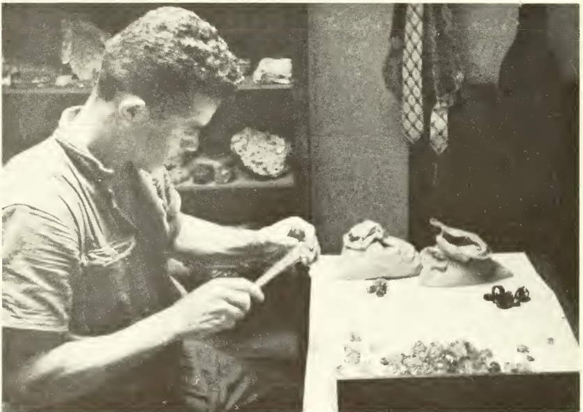
FIG. 2. Cobbing citrine quartz to remove flawed areas.
