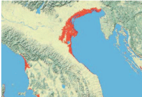
FIGURE 5 (CHAPTER 28) Mapping flood risk by geomorphometry. Inundation of southern European coast (in red), given a potential 3-m rise in sea level, estimated from the 1-km GLOBE DEM ( http://www.cresis.ku.edu/ ). Image credit: Center for Remote Sensing of Ice Sheets. (See page 648 of this volume.)
