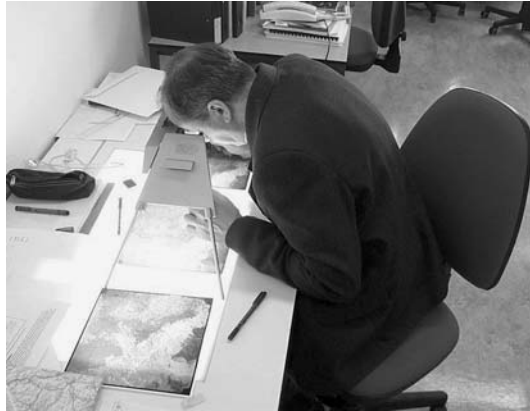
FIGURE 1 Soil surveyor uses a stereophoto and a mylar overlay to delineate (presumable) soil bodies also known as soil mapping units.
