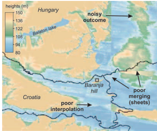
FIGURE 3 (CHAPTER 4) An example of local artefacts in part of the GTOPO DEM (1 km resolution). Such artefacts are only visible after careful inspection. (See page 91 of this volume.)
