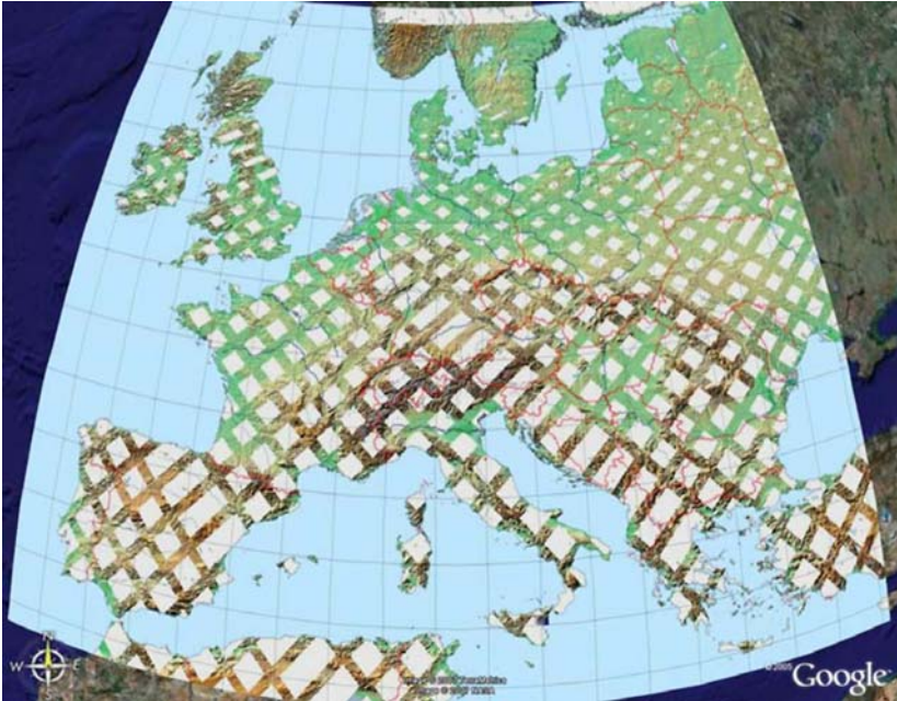
FIGURE 7 Availability of the 1 arcsec SRTM DEMs (C-Band Radar) over the European continent. Missing areas were not acquired due to an energy shortage at the end of the mission (Rabus et al. , 2003). To load the Google Earth map, visit geomorphometry.org . (See page 711 in Colour Plate Section at the back of the book.)
