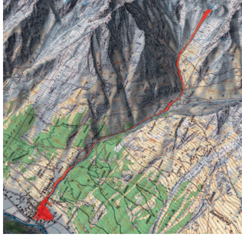
FIGURE 1 (CHAPTER 23) The track and deposits left by the June 2001 flow of debris that overwhelmed the Swiss village of Täsch. Reproduced by permission of SWISSTOPO (BA081244). (See page 535 of this volume.)
