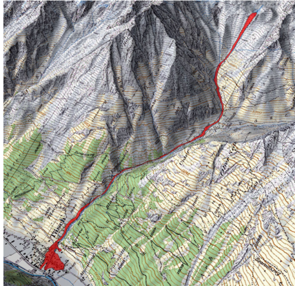
FIGURE 1 The track and deposits left by the June 2001 flow of debris that overwhelmed the Swiss village of Täsch. Reproduced by permission of SWISSTOPO (BA081244). (See page 750 in Colour Plate Section at the back of the book.)
