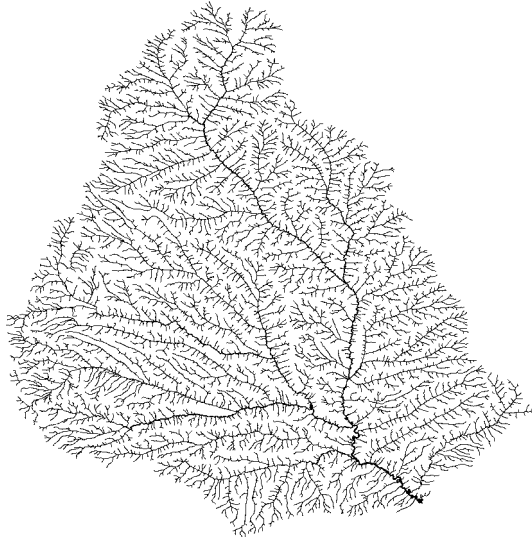
FIGURE 4 Jing River in the Loess Plateau of China, extracted from SRTM data with 3-arcsec grid cells.
