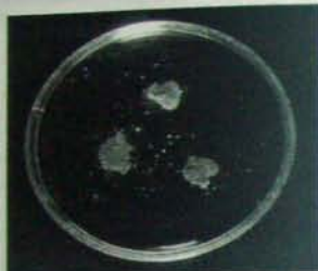
Figure 1. Structural breakdown of aggregates after two hours. The crumbs of fine sandy loam have not dispersed but the one on the left of fine sandy loam has 'slaked'. The crumbs of medium clay have all dispersed, and slaked.
