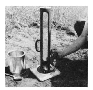
Figure 15–2 Rubber-Balloon Apparatus for Determining Density/Unit Weight of Soil in Place (Courtesy of Soiltest, Inc.)
