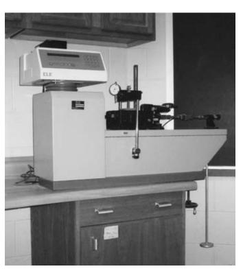
**Figure 23–4** Direct Shear Apparatus
