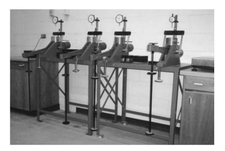
Figure 20–2 Consolidation Device (Courtesy of Cheng Liu)
