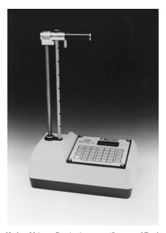
**Figure 16–1** Nuclear Moisture-Density Apparatus (Courtesy of Troxler Electronic Laboratories, Inc., North Carolina).
