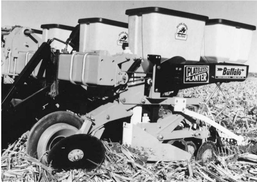
Figure 9-17 A no-till row crop planter. The planter is equipped to open the furrow, push crop residue to the side, fertilize, and apply herbicides. This type of implement will work equally well in untilled wheat stubble or in clean-tilled land. (Courtesy Fleischer Manufacturing, Inc., Columbus, Nebraska.)
