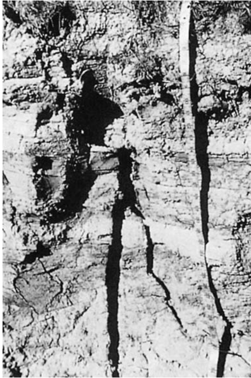
Figure 3–9 Varved clay deposit in Michigan. Each varve is about 1 mm thick and is composed of a thin, sandy layer deposited during the summer thaw and a coating of silt and clay deposited while the glacial lake was frozen. The scale is in centimeters. (Courtesy Roy L. Donahue.)
