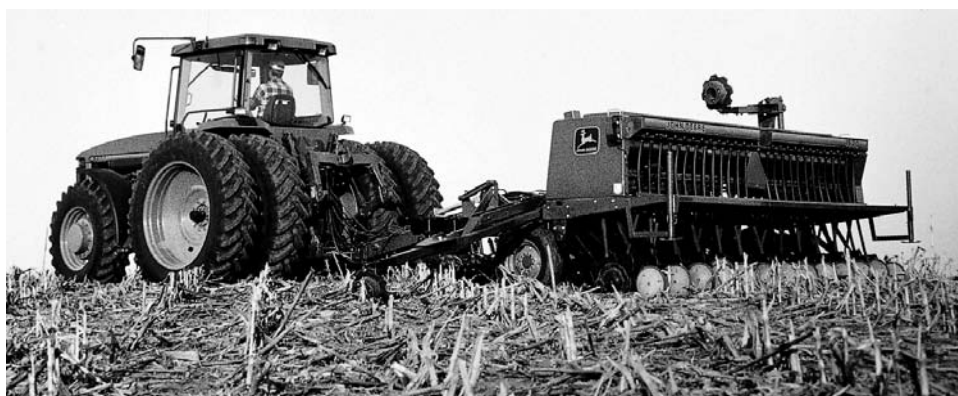
Figure 9–15 A heavy double-disk grain drill designed to seed small grain through reasonable quantities of crop residue. It can be purchased with a variety of furrow openers. (Courtesy Deere and Company, Moline, Illinois.)
