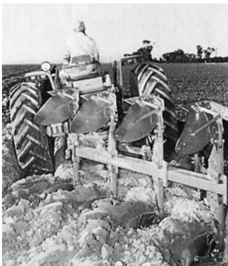
Figure 9-3 A four-bottom rollover (two-way) moldboard plow. The plowshare or cutting edge, the curved moldboard, and the landside are visible on the units in the air. The “two-way” feature makes it possible to turn all furrows in one direction, an excellent feature in a soil conservation program. The soil behind the plow has been inverted and crumbled. (Courtesy Massey Ferguson, Inc., Des Moines, Iowa.)
