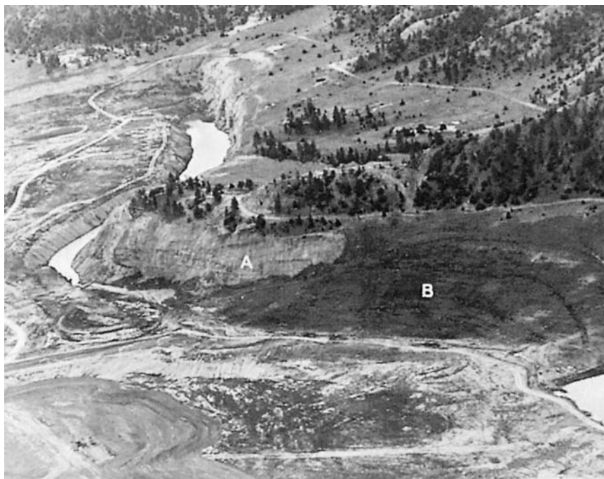
Figure 11-8 The highwall labelled A in this photo of a mine in Montana resulted from strip mining that was done before Montana law required that ponds be filled and slopes be smoothed. The area labelled B was mined later and reduced to a 3:1 (33%) gradient to meet state and federal requirements. (Courtesy USDI Bureau of Mines.)
