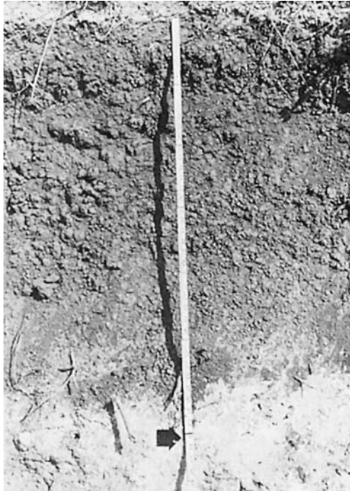
Figure 7-5 A soil profile of the Abilene series (Pachic Argiustoll) in the 25-in. (640-mm) precipitation belt in Texas. This soil supports a good growth of nutritious range grasses. The depth to the whitish calcium carbonate zone at the bottom of the photo is about 3 ft (nearly a meter). ( Note: the arrow is at 1 meter.) (Courtesy Texas Agricultural Experiment Station.)
