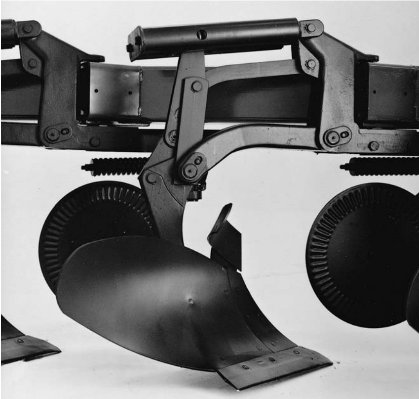
Figure 9–2 A single moldboard plow unit. The sharpened plowshare on the bottom cuts the furrow slice free from the soil. The curved moldboard, above the share, slides the furrow slice into an inverted position. The small, curved trash board guides the standing stubble and other trash beneath the furrow slice as it is inverted. The flat disk in front of the share is a coulter that cuts through crop residue and trash and partially cuts the side of the furrow slice. Not shown, because it is hidden behind the moldboard, is the landside—a flat, vertical plate—that presses against the side of the furrow and prevents the plow from sliding sidewise as it is drawn through the soil. These units can be joined together along a heavy beam to make anything from a two-bottom plow to a 10-bottom plow (or even larger). (Courtesy Deere and Company, Moline, Illinois.)
