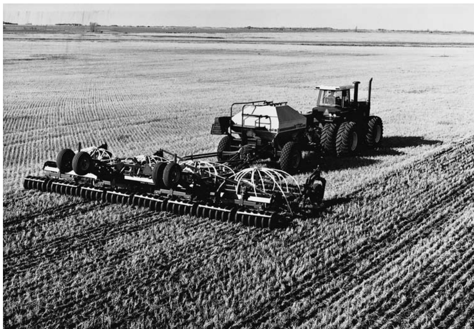
Figure 9-18 A no-till grain drill with rugged, high-clearance furrow openers and a combined air seeder/fertilizer applicator. This unit comes in widths from 27 to 57 ft (8.2 to 17.4 m) and is capable of seeding through dense residues on untilled small grain or row crop fields. An herbicide application attachment is available. (Courtesy CNH Global N.V., Saskatoon, Saskatchewan, Canada.)
