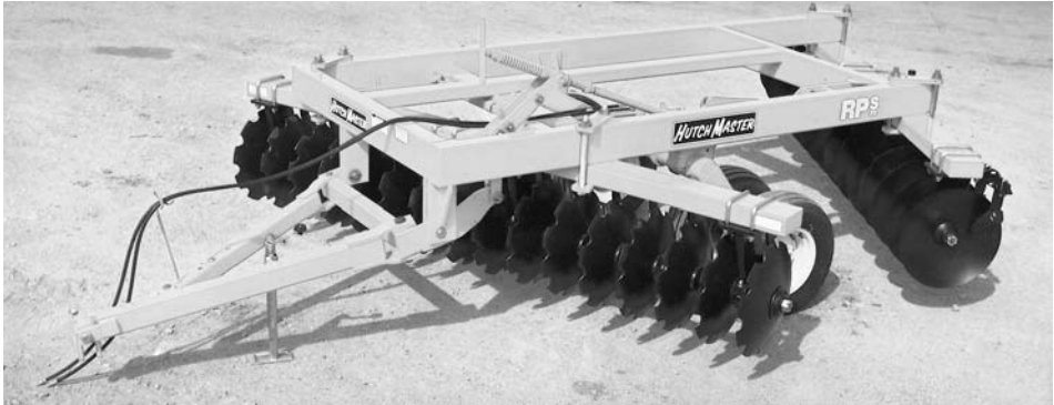
Figure 9-5 An offset disk. This heavy-framed, large implement has replaced the moldboard plow and disk plow as an initial tillage tool on many farms. (Courtesy Wil-Rich Manufacturing Co., Wahpeton, North Dakota.)
