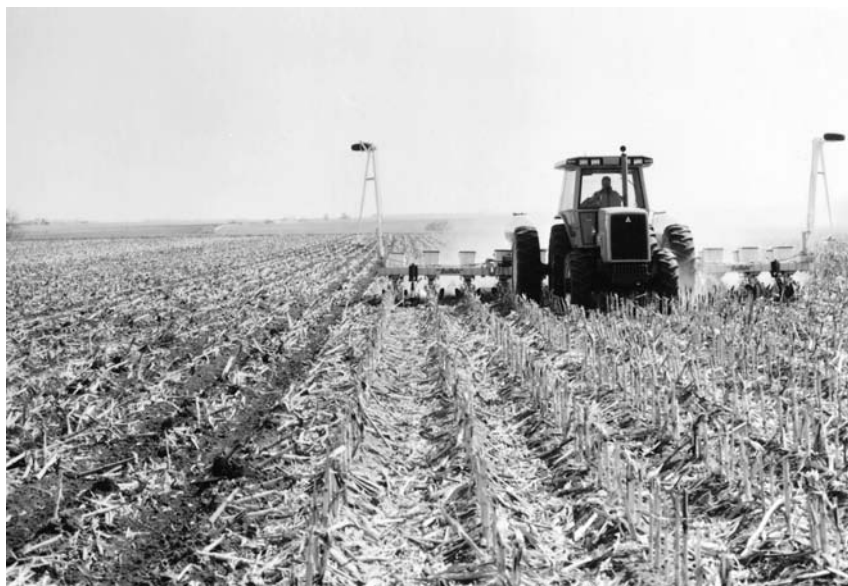
Figure 9–14 Row crops can be seeded in untilled soil with a no-till planter. This machine is adapted to plant on former crop ridges in order to maintain a ridged condition for erosion control. Attachments for this and other makes and models are available to apply either dry or liquid herbicides in addition to dry fertilizer. (Courtesy Fleischer Manufacturing Co., Columbus, Nebraska.)
