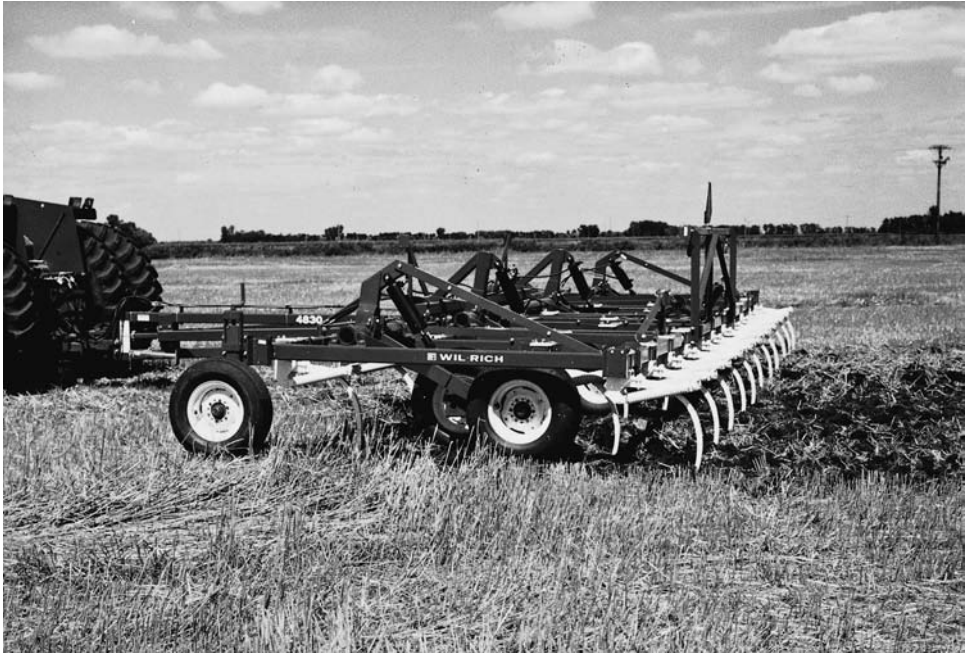
Figure 9–7 A chisel plow equipped with narrow points. Shanks are mounted on the frame in tiers so that any bunched crop residue will flow through the machine easily. (Courtesy Wil-Rich Manufacturing Co., Wahpeton, North Dakota.)
