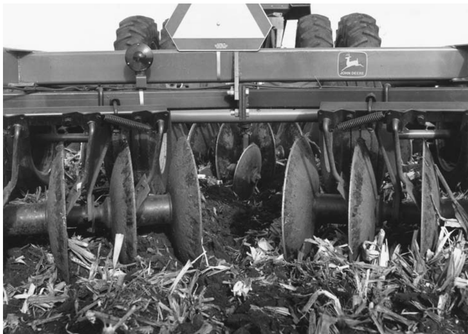
Figure 9-4 A tandem disk. The front disks turn the furrows out from the center, the rear disks toward the center. Such implements produce a relatively smooth surface and cover part of the crop residues. This unit is equipped with a “floating” central small disk that cuts the ridge left by the front disk gangs. (Courtesy Deere and Company, Moline, Illinois.)
