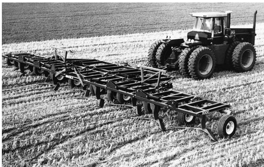
Figure 9-9 A Noble™ blade implement with rugged construction and large clearance between adjacent shanks and between blades and frame. This model has nine 6-ft (1.8-m) “V” blades for a total working width of 49.5 ft (15.0 m). The frame is flexible so that each blade will conform to the land surface and work at a uniform depth. (Courtesy Cereal Implements [Vicon], Portage la Prairie, Manitoba.)
