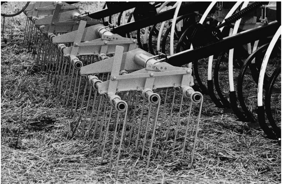
Figure 9-6 A spring harrow mounted behind a planter. The spring tines can be set at different angles to accommodate the purpose for which the implement is to be used—smoothing the soil surface, spreading straw, etc. (Courtesy Bourgault Industries Inc., Minot, North Dakota.)
