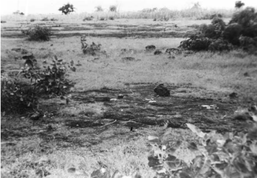
Figure 2–10 Ironstone (hardened plinthite) in a tropical soil in Ghana exposed by the erosion of about 6 in. (15 cm) of overlying soil. (Courtesy Henry Obeng.)
