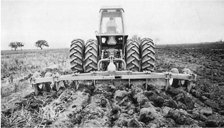
Figure 9–19 Deep chiseling a field leaves clods on the surface and deep chisel marks in the soil. (Courtesy Allis-Chalmers Corporation, Milwaukee, Wisconsin.)
