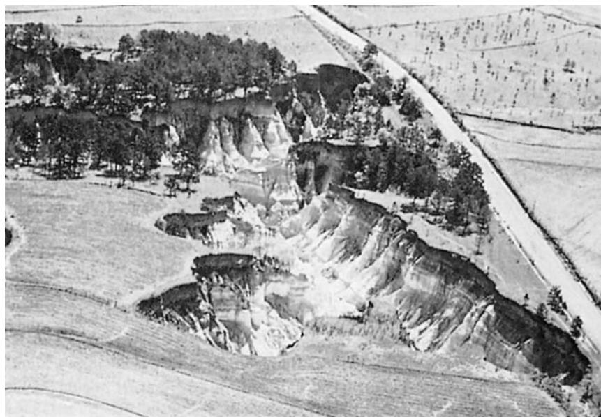
Figure 11-10 Part of a gully near Lumpkin, Georgia. Gullying in this area was neglected for more than 100 years. The gully became several miles long and 50- to 200-ft (15- to 60-m) deep, affecting an area of about 100,000 ac (40,000 ha). (Courtesy USDA Natural Resources Conservation Service.)
