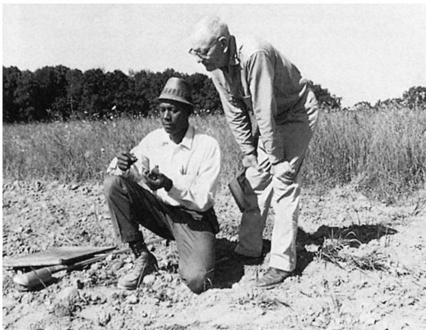
Figure 7-1 This soil surveyor is showing the farmer how he uses 10% HCl solution to detect the presence of calcium carbonate in soils and rocks. This information helps him classify the soil and make a map that will help natural resource managers make efficient long-term use of the land. (Courtesy USDA Natural Resources Conservation Service.)
