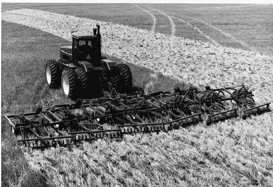
Figure 9-11 Skew treaders attached behind a gang of chisel plows. The treaders help to smooth the seedbed and to anchor the loose straw in the soil. A large amount of residue remains on the ground surface after this combined operation. (Courtesy Sunflower Manufacturing, Beloit, Kansas.)
