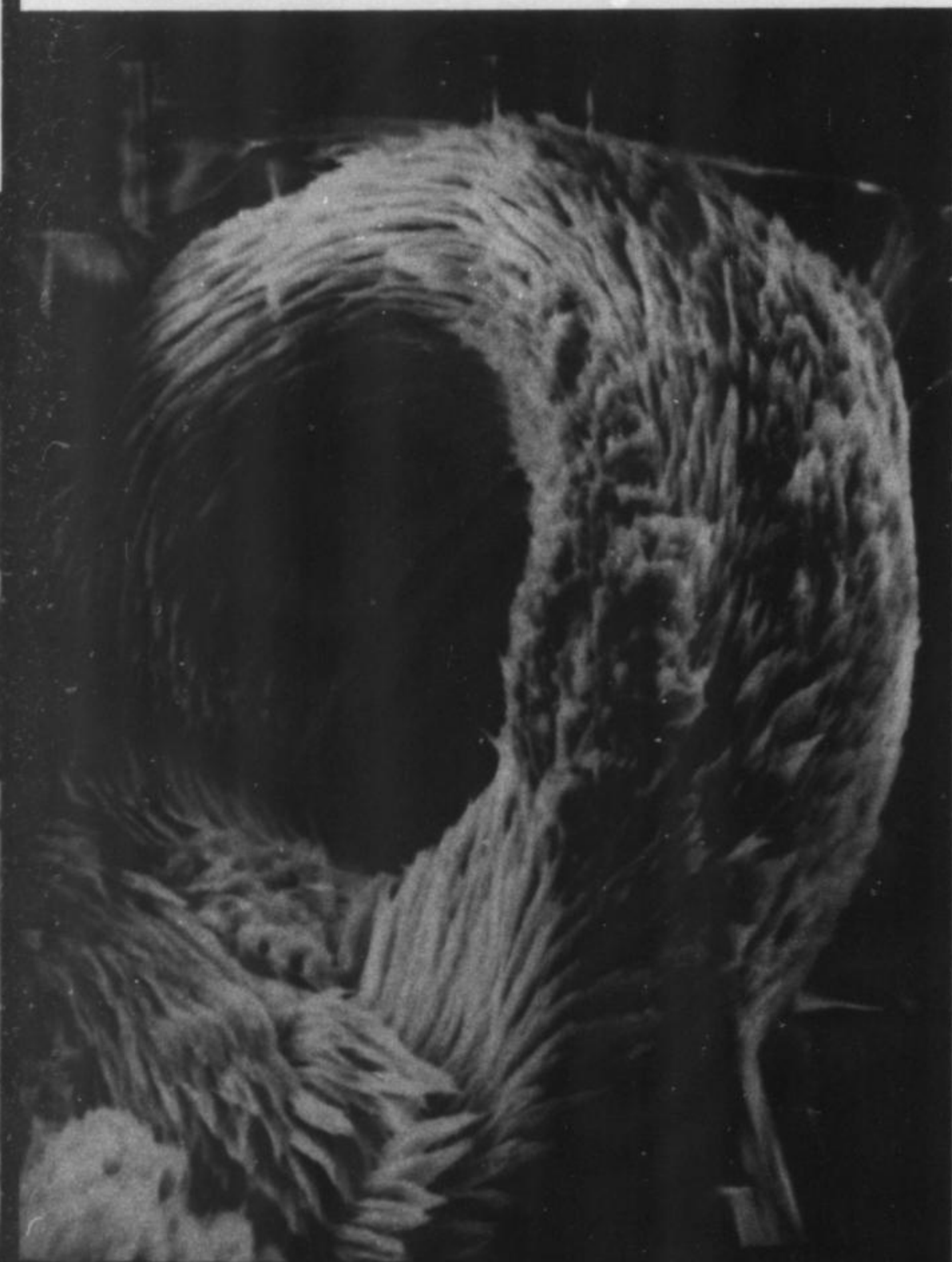
Fig. 7 (above) Pyrite, Hall's Gap, Kentucky. 800X (SEM). Specimen, Douglas Berndt, Eastman Kodak.
