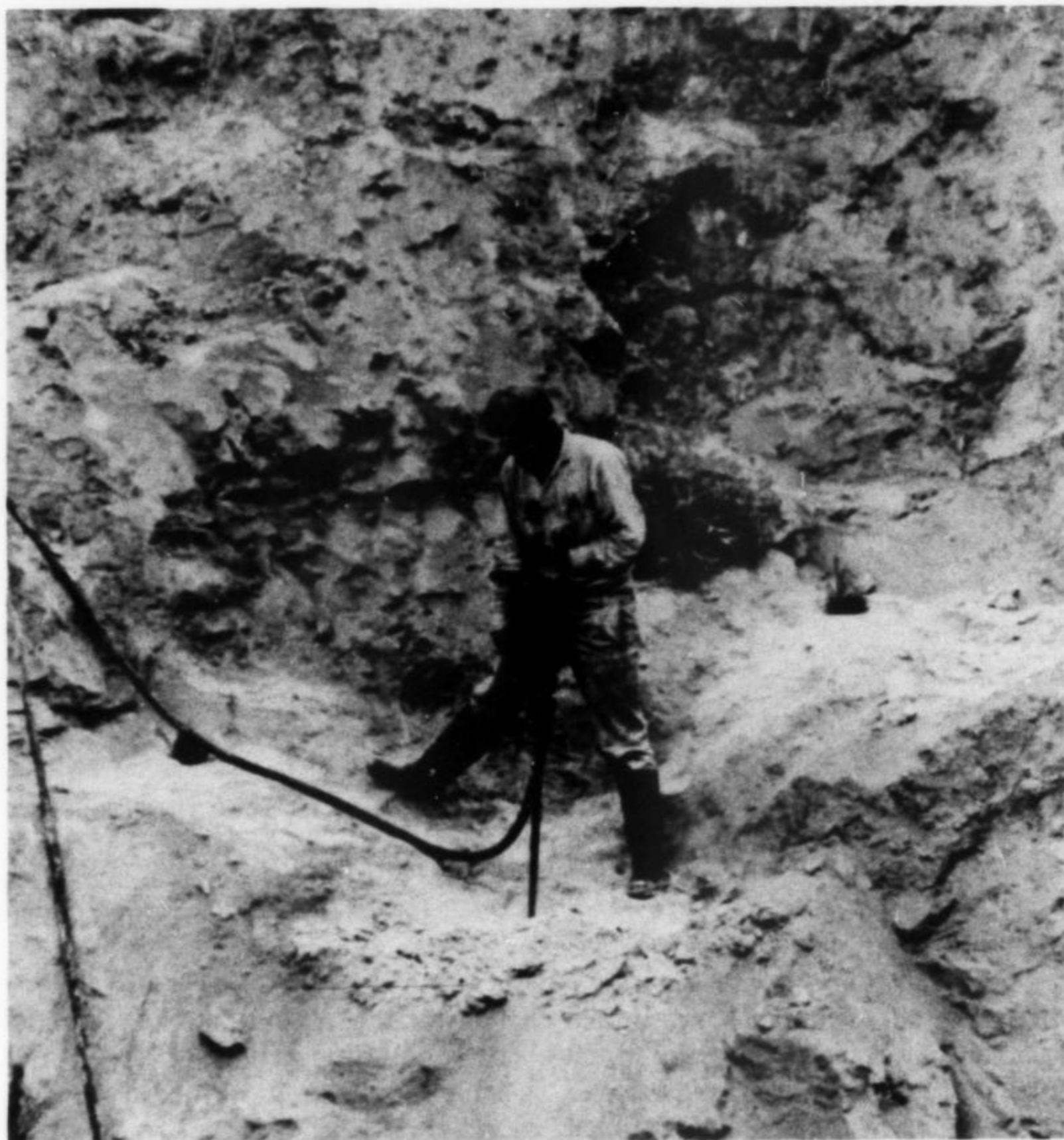
Most mining at Chivor is by hand, because of the fragile nature of the emeralds. When necessary a limited amount of drilling and light blasting is done.
