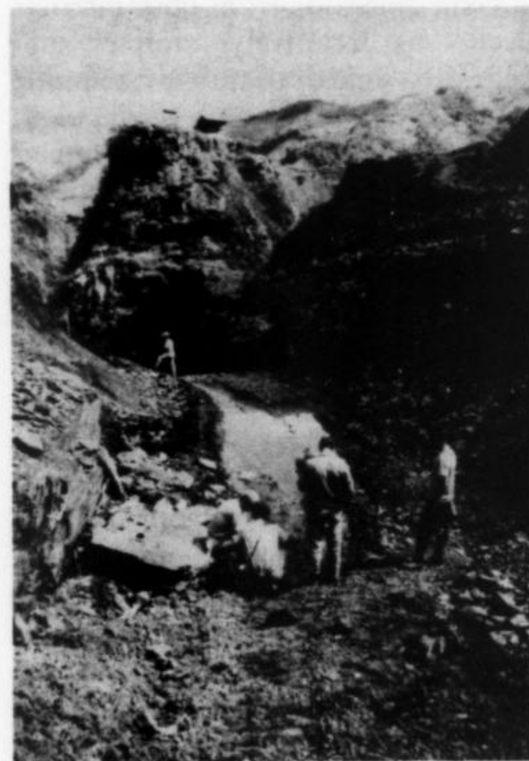
The working face at the Muzo mine lies at the foot of a large, steep open cut. Emerald veins occur very sparsely in the soft, black shale.
