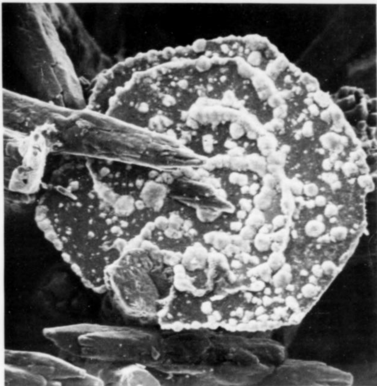
Figure 8. A second zincite crystal showing spiral growth and the associated acicular calcite. (SEM photo at 270 \times ).
