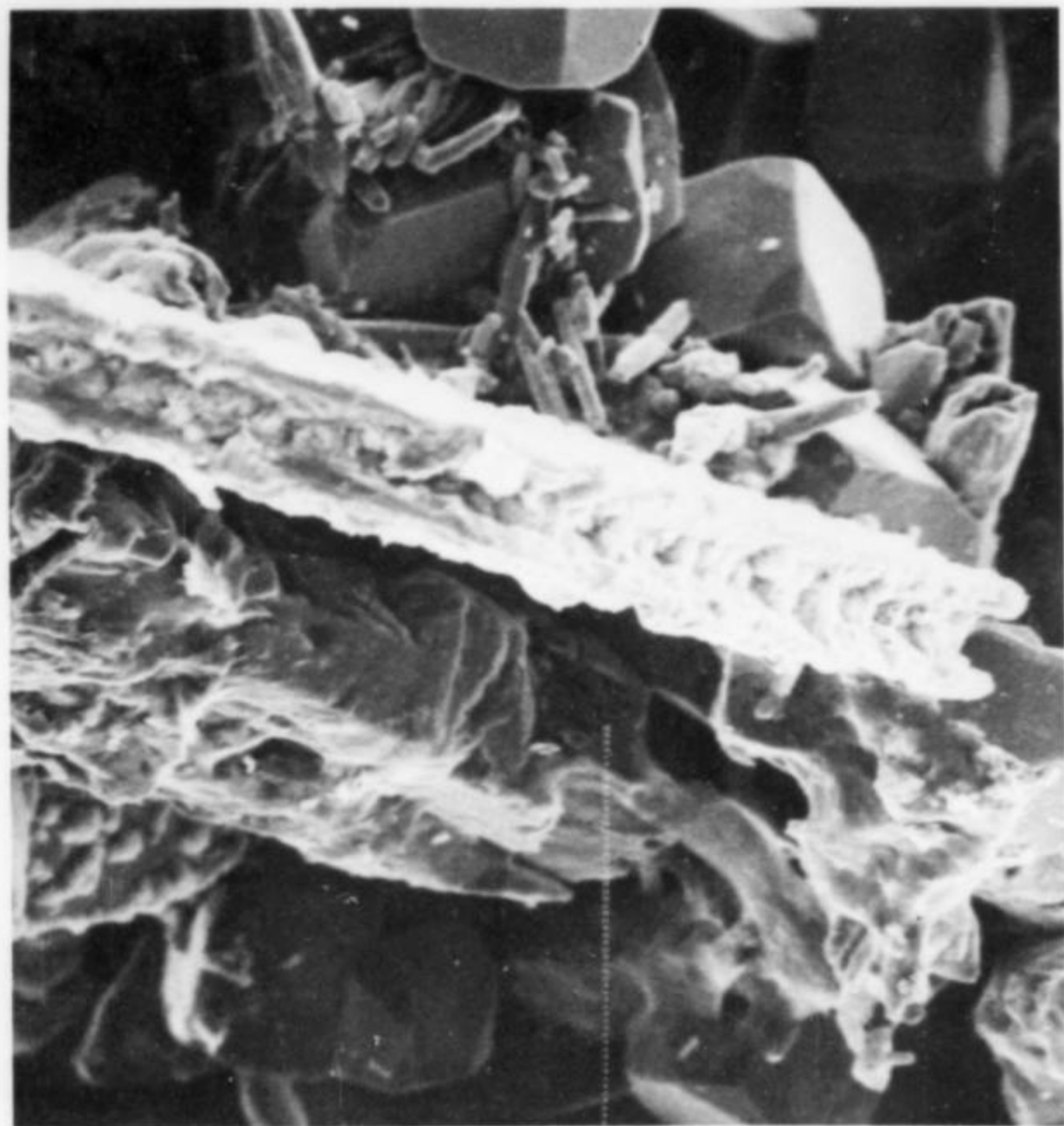
Figure 4. View along apparent a -axis of the zincite crystals shown in Figure 2, showing the apparently twinned nature of these zincite crystals. (SEM photo at 260 \times ). Note the trisectahedron form on franklinite.
