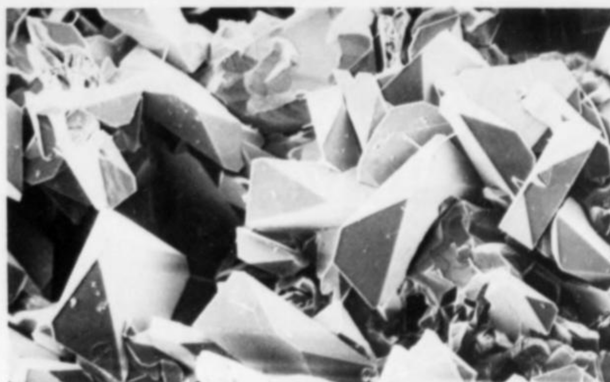
Figure 3. Bright yellow crystals of jarosite from Graves Mountain, Georgia (X540, SEM photograph).
