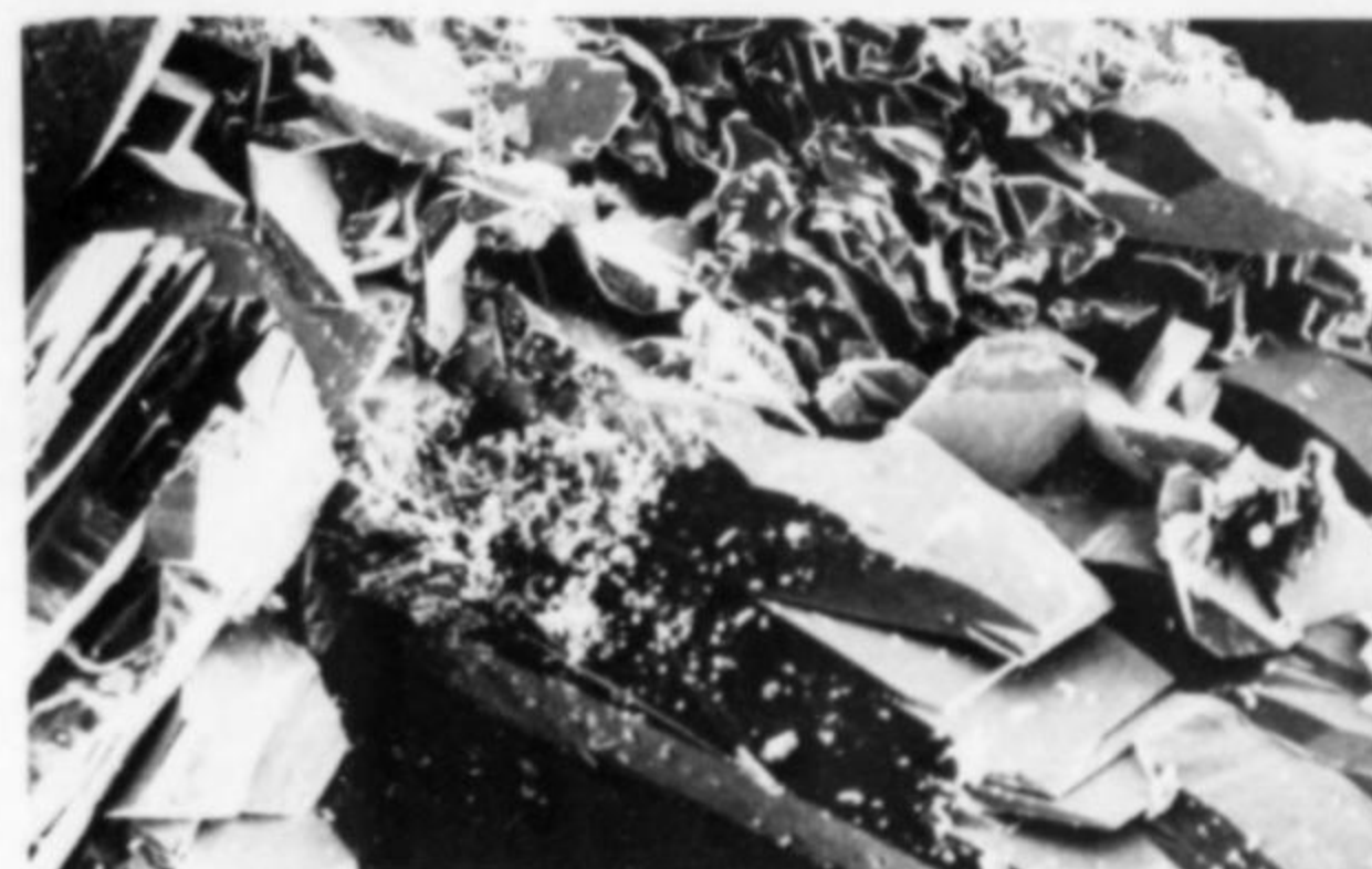
Figure 4. Pink phosphosiderite crystals with jarosite from Graves Mountain, Georgia (X54, SEM photograph).
