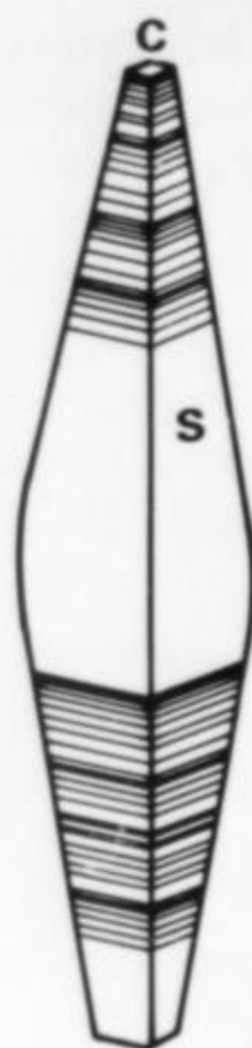
Figure 11. Sketch of a doubly terminated prehnite crystal (NMNS #32675). Crystal forms are the rhombic pyramid s\{111\} and the pinacoid c\{001\} . The other \{\bar{1}11\} pyramid is behind the crystal.
