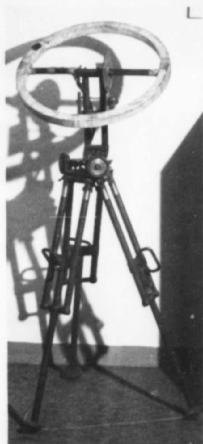
Figure 13. An old plane table (surveyor's device) in the Tsumeb Museum.
