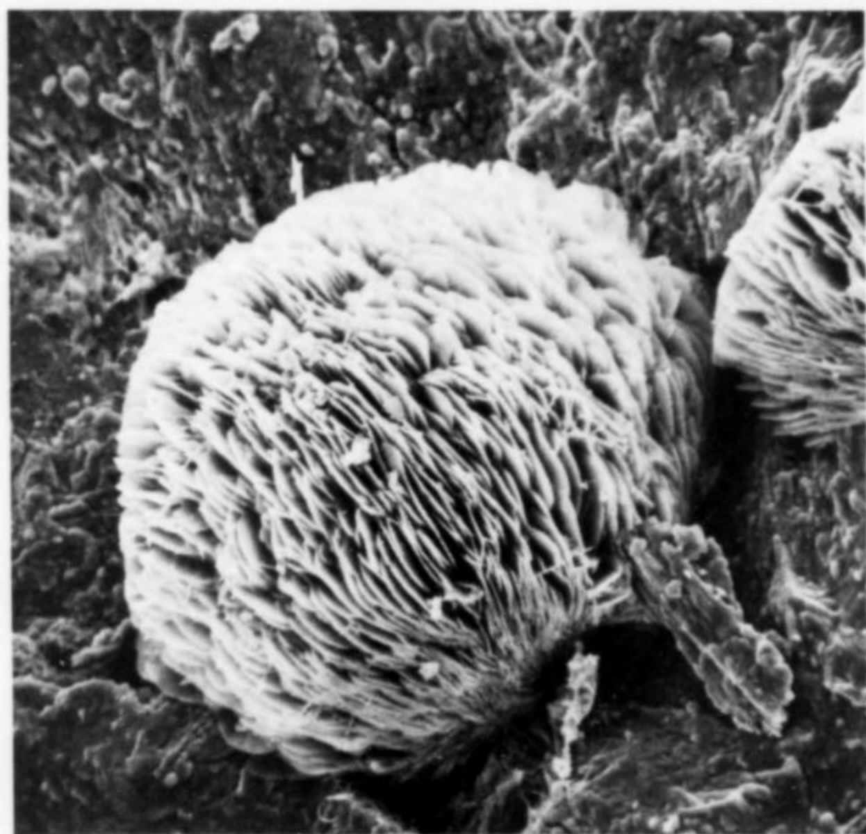
Figure 11. Scanning electron photo-micrograph of a spherical aggregate of dypingite from Sterling Hill (425X).
