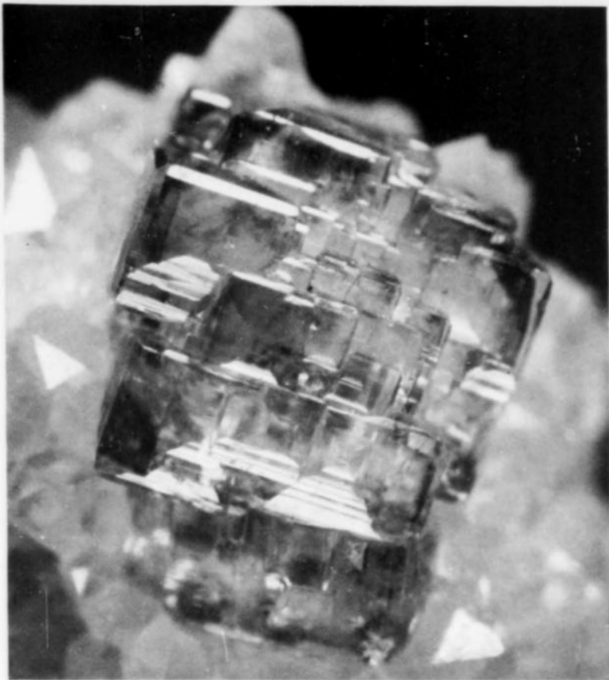
Figure 6. Pale blue, slightly zoned fluorite crystals in parallel growth, showing major cube plus dodecahedron (brilliant highlights) and tetra-hexahedron (lesser highlights). The size of the group is 5 mm.
