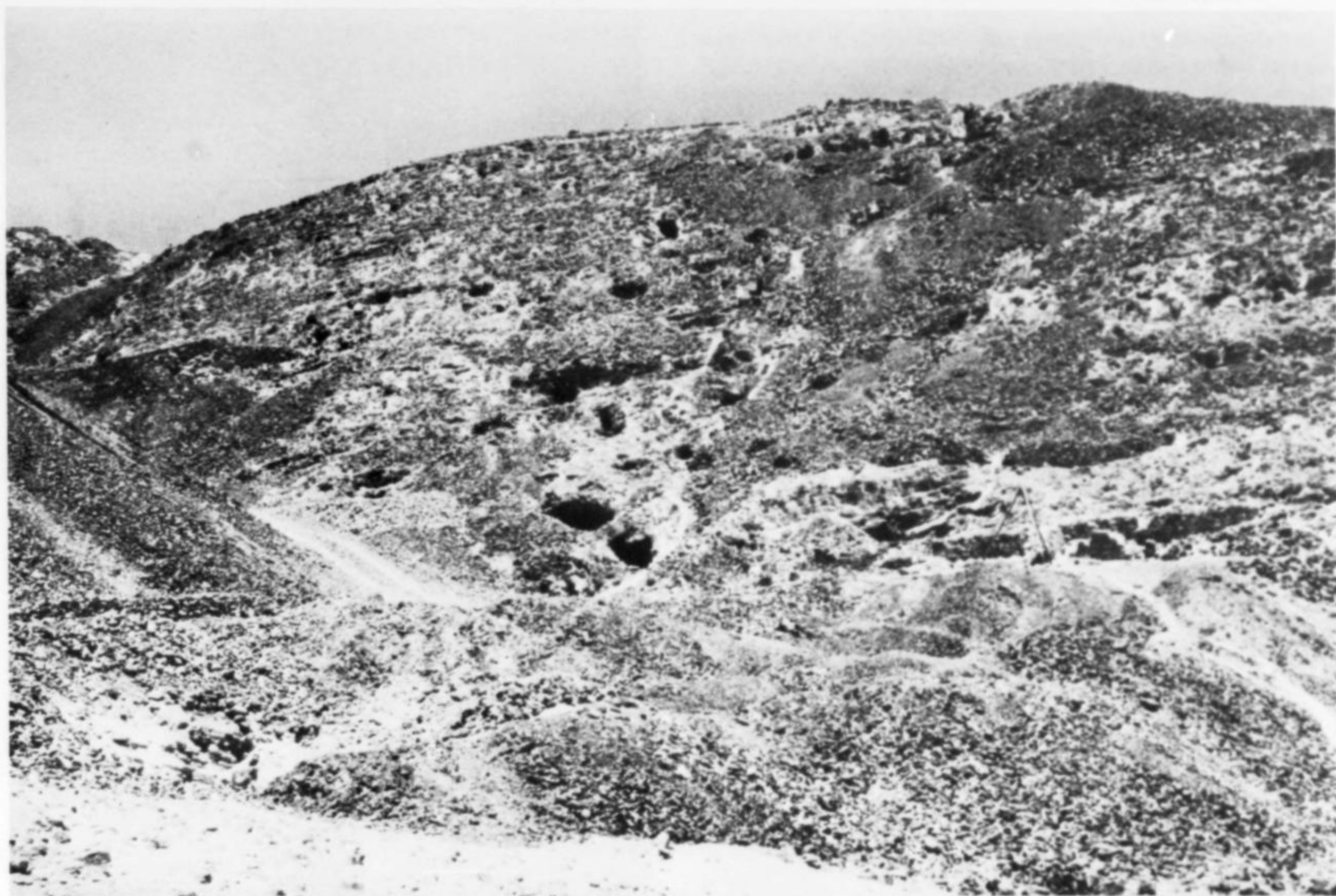
Figure 4. Recent photograph (1976) of open stopes and dumps along one of the major Chañarcillo vein systems.
