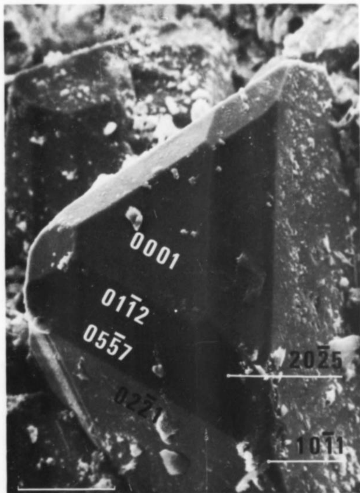
Figure 8. SEM photograph of paratacamite crystal showing the rare form \{05\bar{5}7\} and others. Length of the bar is 50 \mu\text{m} .
