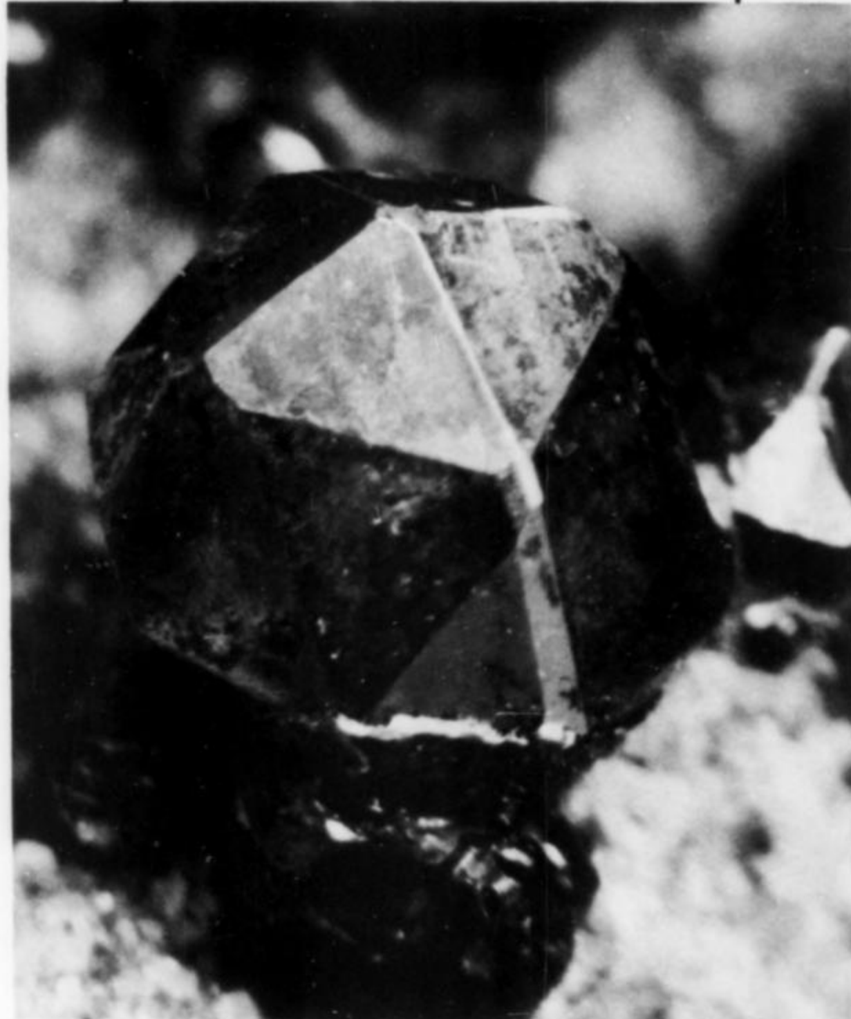
Figure 5. ROM #M35608. Photomicrograph and sketch of the combination of the trapezohedron {112} and the octahedron o\{111\} , in almost equal development. The other faces shown are the dodecahedron, pyritohedron, and trisoctahedron. The crystal is about 3 mm in diameter. Compare with the ideal drawing of this combination to the upper right.
