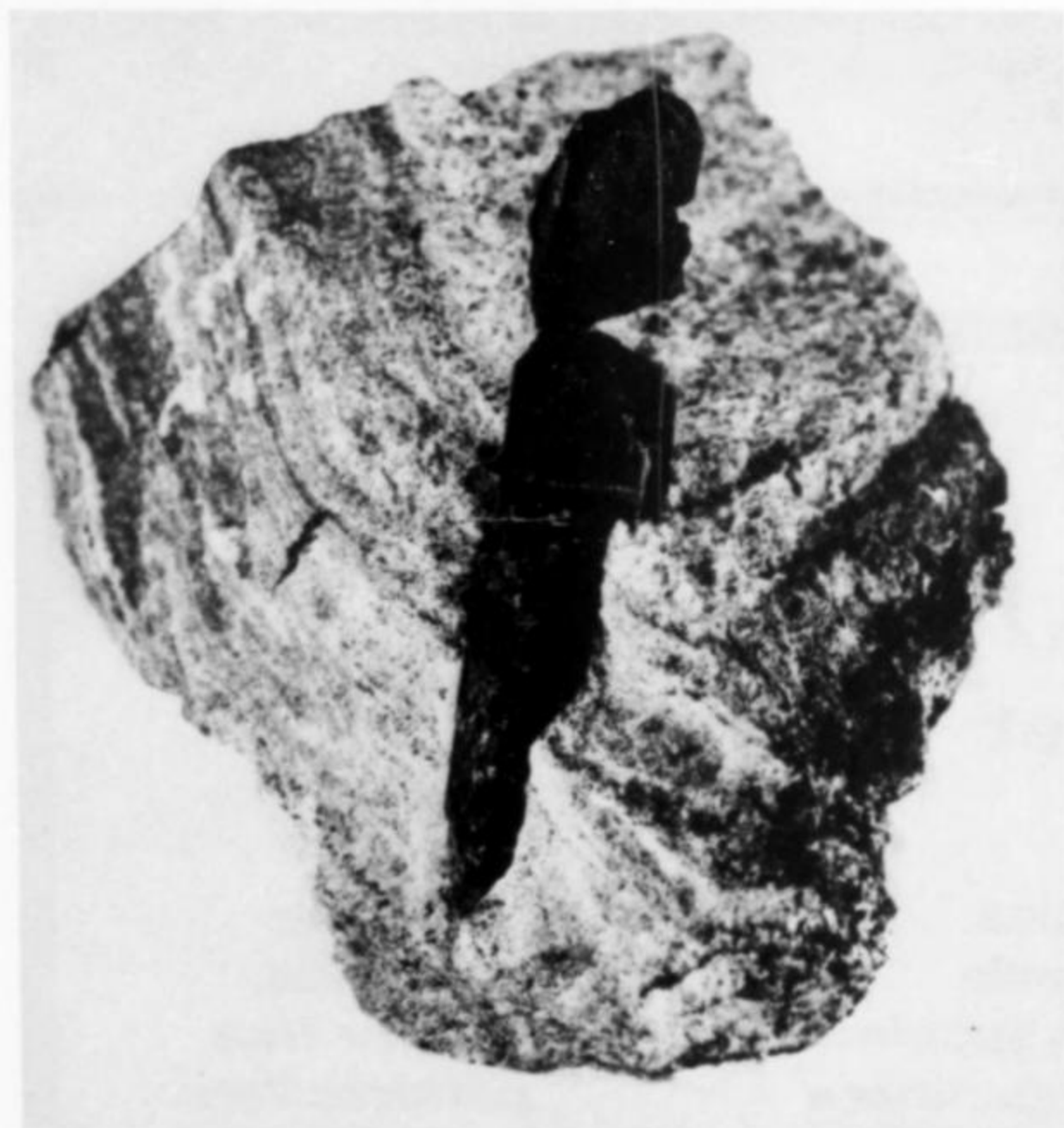
Figure 3. The largest crystal found, 23 cm long, showing \{110\} , \{100\} and \{021\} . The crystal is not shown in the correct crystallographic orientation.
