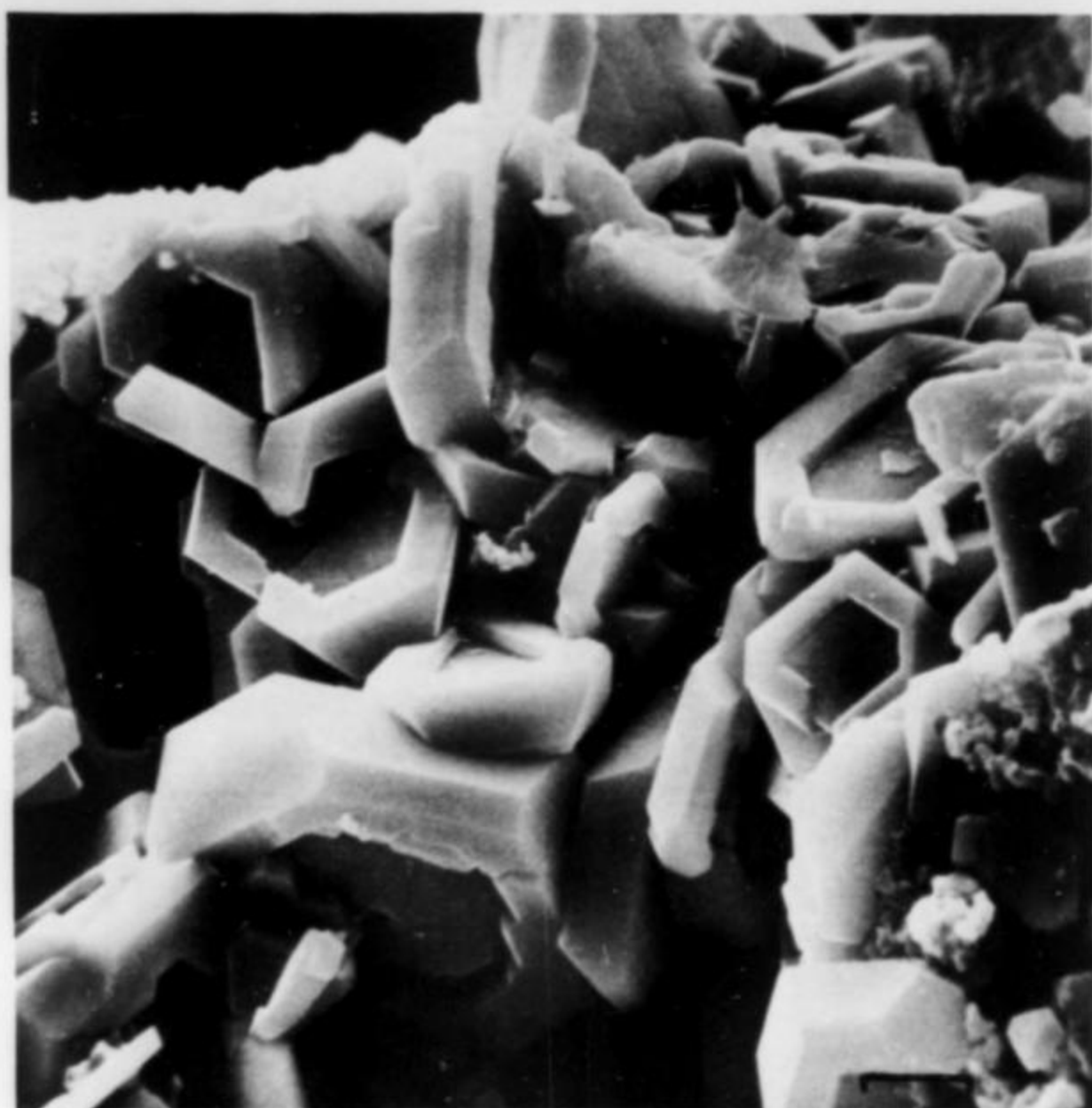
Figure 4. SEM photograph of osarizawaite-beaverite intergrowths. Length of the bar is 1.5 \mu\text{m} .
