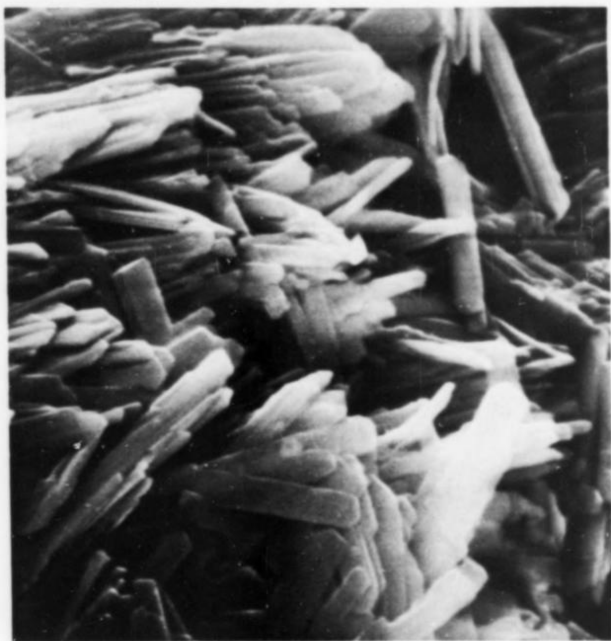
Figure 7. Lath-shaped crystals of gearsutite as seen at high magnification. (SEM photo at 12,200x).
