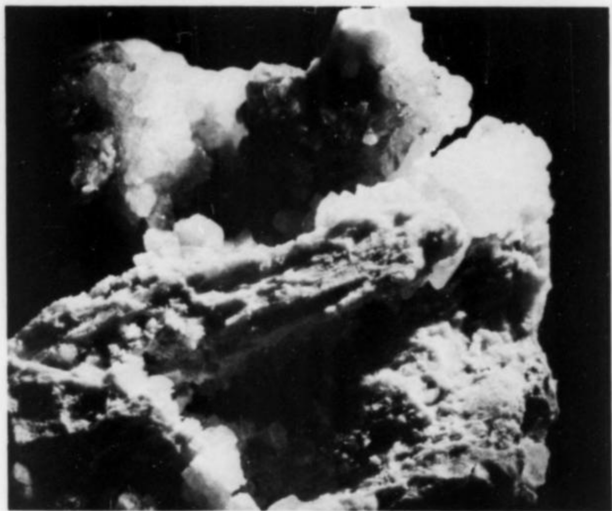
Figure 5. An almost totally replaced lanarkite prism, showing an additional coating of cerussite (specimen width is 2 cm).
