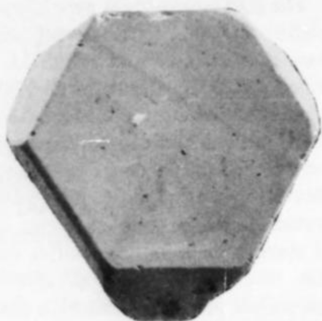
Figure 4. Sperrylite crystal, platy parallel to an octahedron face. Crystal size 0.5 mm. Scanning electron micrograph.
