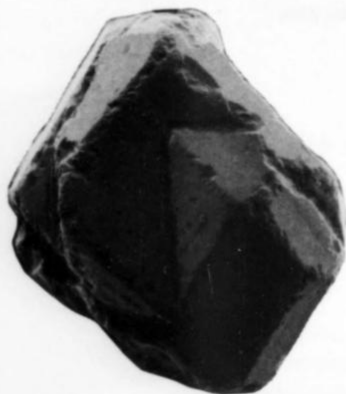
Figure 6. Octahedral sperrylite twinned on (011). Crystal size 0.4 mm. Scanning electron micrograph.
