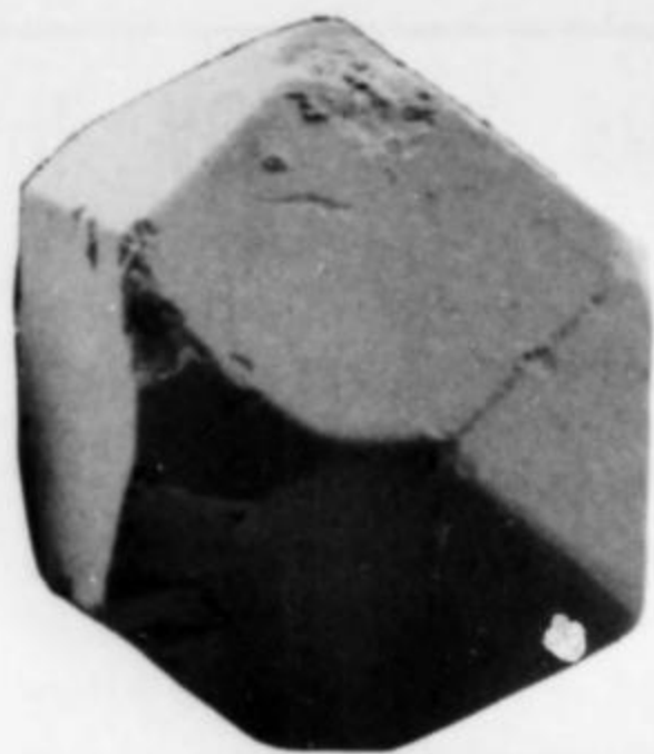
Figure 3. Sperrylite crystal, a combination of a cube {100} and an octahedron {111} with traces of some dodecahedron {110} faces. Crystal size 0.3 mm. Scanning electron micrograph.
