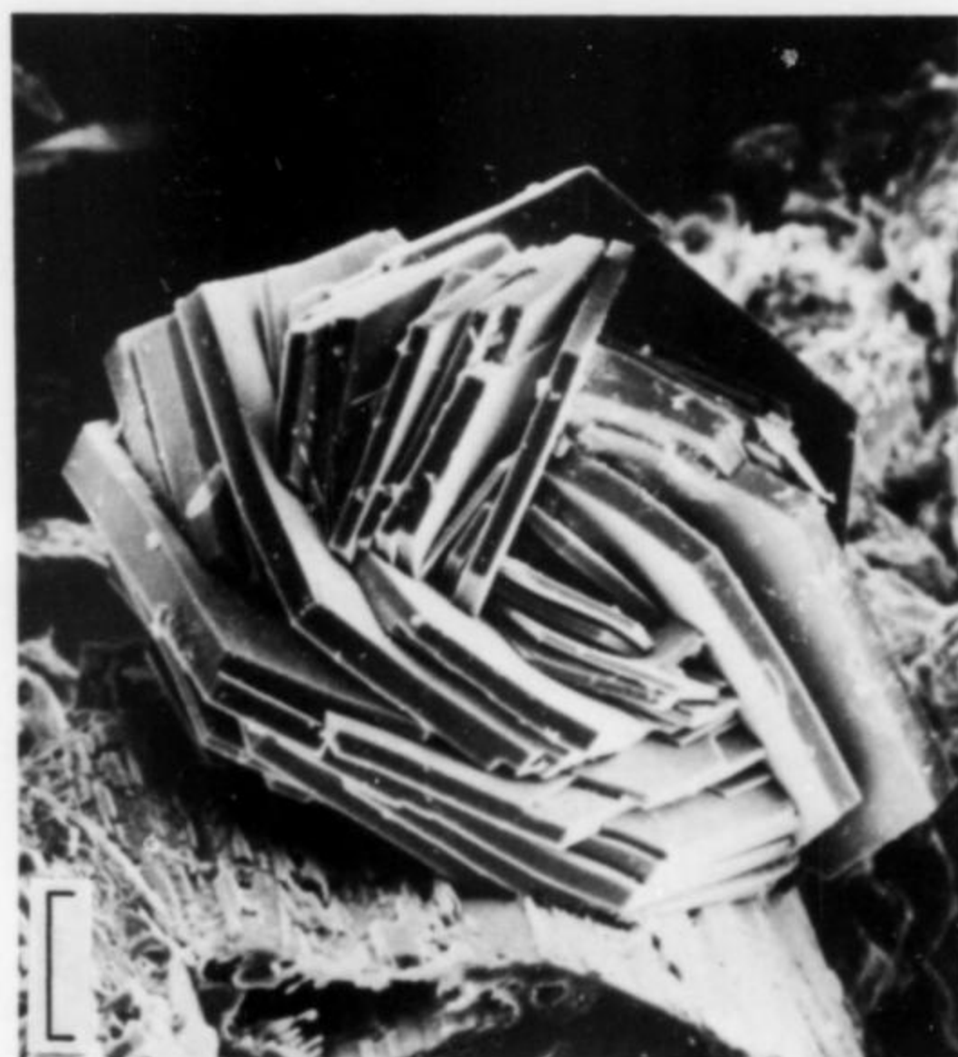
Figure 26. Scanning electron micrograph of a rosette of tabular truscottite on leached potassium-feldspar from ~120 m in drill hole Y-13. Scale bar is 20 microns.
