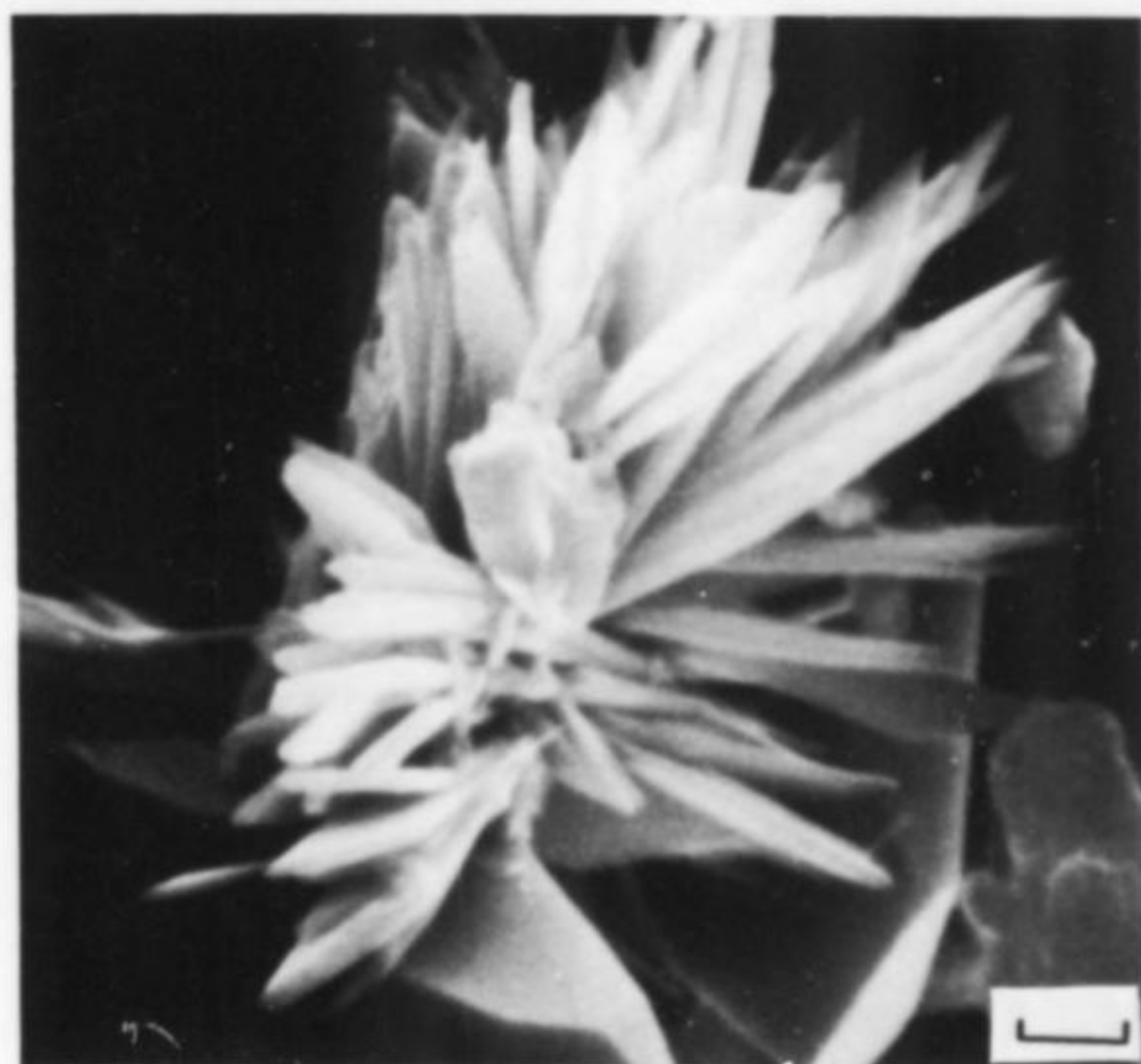
Figure 30. Scanning electron micrograph showing a radiating cluster of bladed pectolite crystals on hydrothermal quartz prisms from ~28 m in drill hole Y-3. Scale bar is 1 micron.
