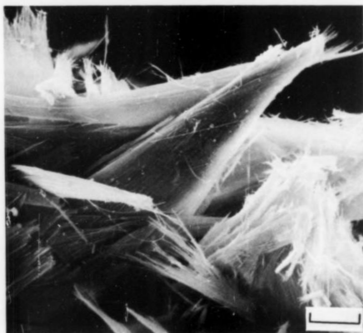
Figure 28. Scanning electron micrograph of fibrous gyrolite from ~28 m in drill hole C-1. Scale bar is 10 microns.
