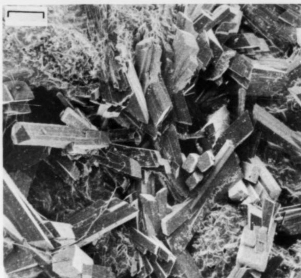
Figure 17. Scanning electron micrograph of laumontite crystals from ~ 86 m in drill hole Y-3. Fine particles on crystals are mixed-layer illite-montmorillonite. Scale bar is 300 microns.
