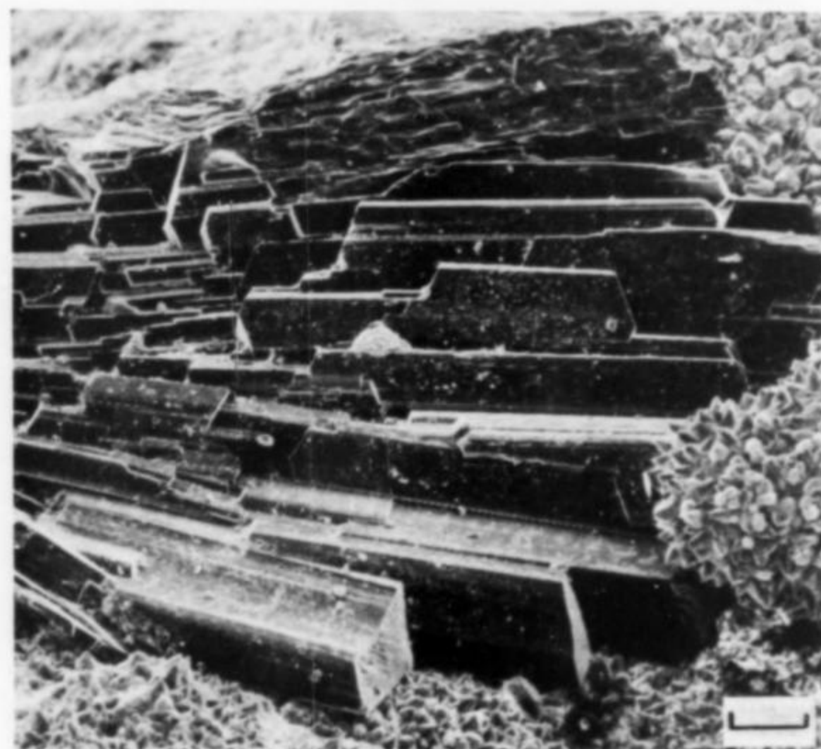
Figure 20. Scanning electron micrograph of a large radiating cluster of dachiardite crystals deposited on hydrothermal quartz crystals in a cavity at ~60 m in drill hole Y-3. Scale bar is 200 microns.
