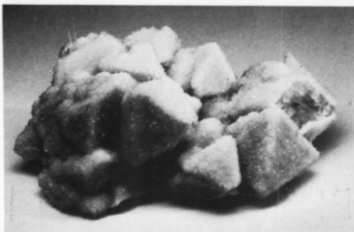
Figure 7. White drusy quartz encrusting fluorite octahedra. The specimen is 5.5 inches across (U.B.C. #S-4852).
