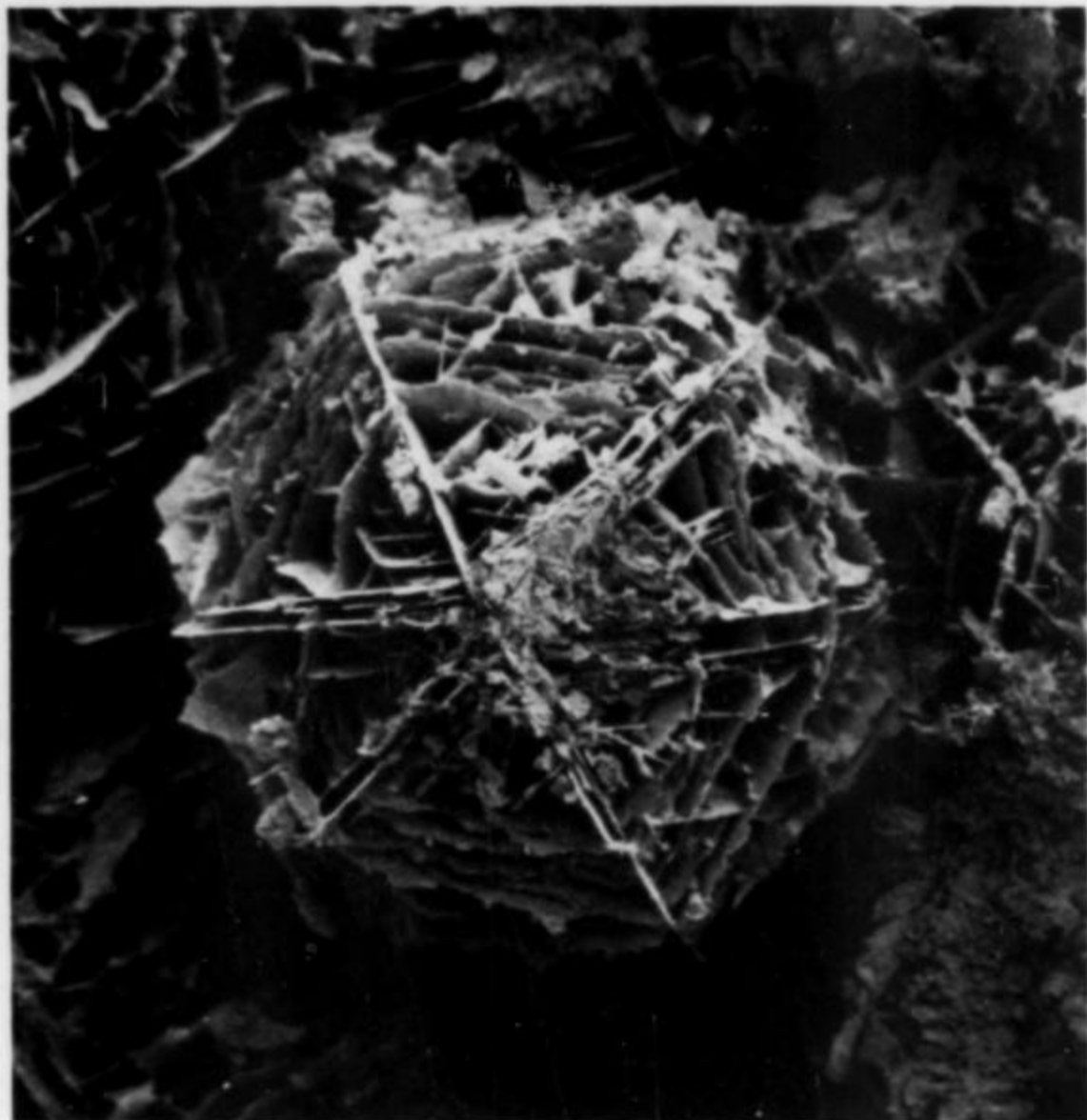
Figure 7. Complicated rosette of ferritungstite. Borralha mine, Minho, Portugal. Diameter of rosette: 70 microns. Scanning electron micrograph.
