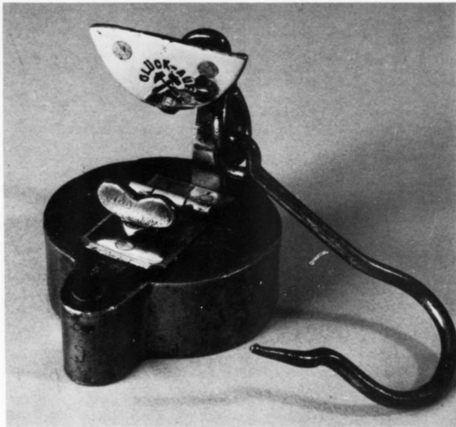
Figure 1. A German miner's lamp, known as a frog lamp, dated around 1880. Note the "GLÜCK AUF" and the Schlägel und Eisen (crossed mallet and gad) on the shield. Wendell Wilson collection.
