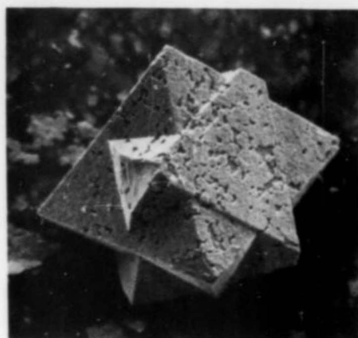
Figure 11. Penetration twin of almotungstite with a semi-loose skin. Nyamulilo mine, Uganda. Size of crystal: 70 microns. Scanning electron micrograph.
