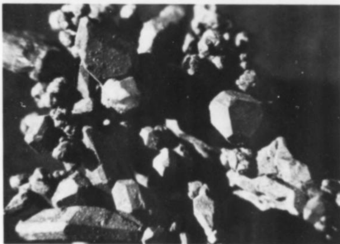
Figure 15. Native copper group 13 mm across, dark red-brown crystals showing cube and octahedron; Broken Hill, New South Wales. Photo by Bill Henderson.
