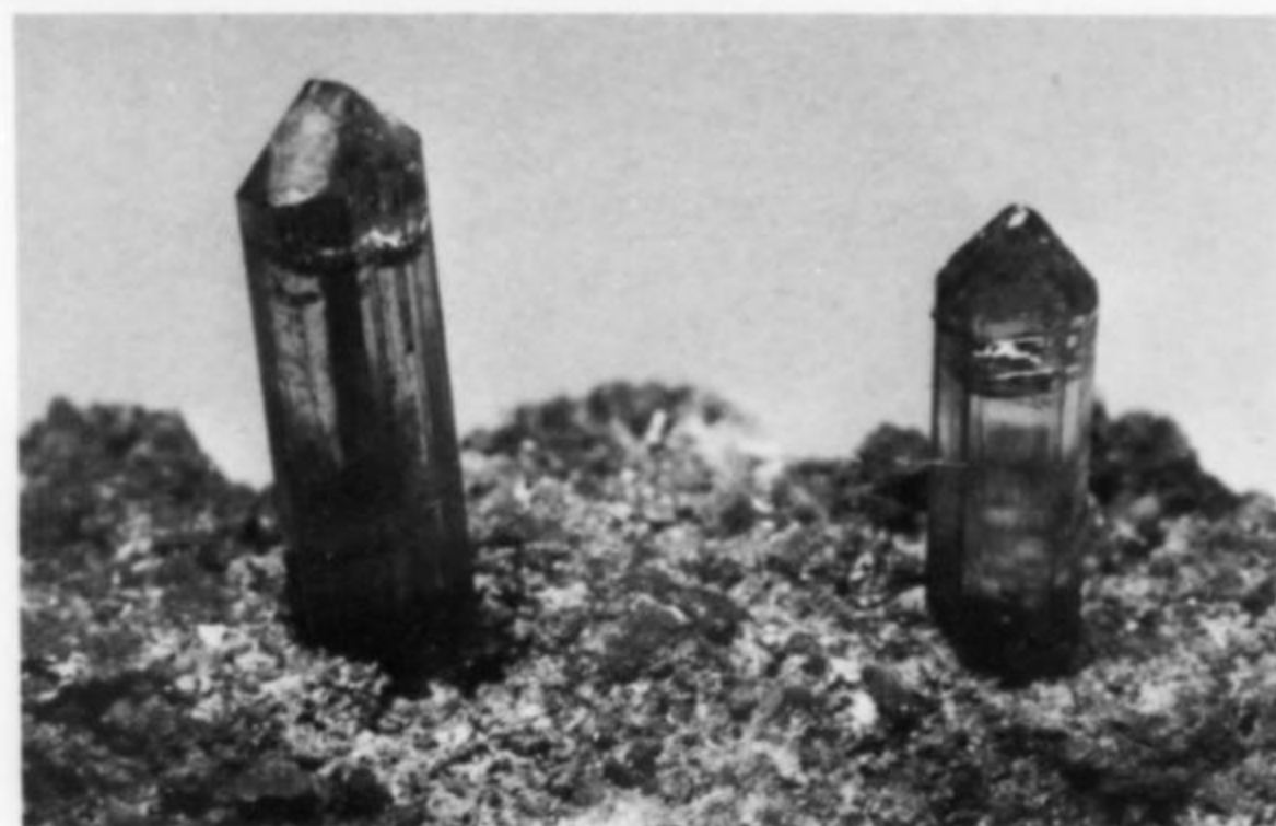
Figure 4. Pink and green elbaite crystals (left crystal is 1.5 cm) imbedded in reconstituted matrix. Purported locality: Minas Gerais, Brazil. The "matrix" around the crystals is crushed lepidolite made into a paste with glue. (Bentley collection.)
