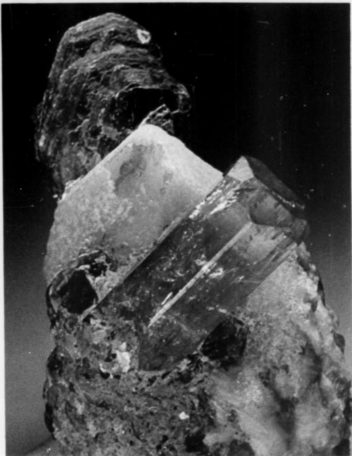
Figure 12. Beryl (aquamarine) crystal glued on matrix. Purported locality: Klein Spitzkopje, Southwest Africa. The crystal is about 2.5 cm tall. Note rock powder paste used as glue. (Harvard specimen #98382.)
