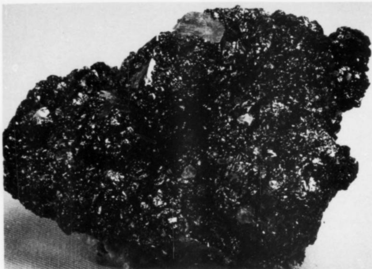
Figure 18. Black, highly lustrous, tetrahedral crystals of sphalerite with rounded faces and contact twinning, on galena. The three pale purple fluorite crystals show strong development of the tetrahexahedron \{210\} . Size: 4 x 5 inches; no. 475.
