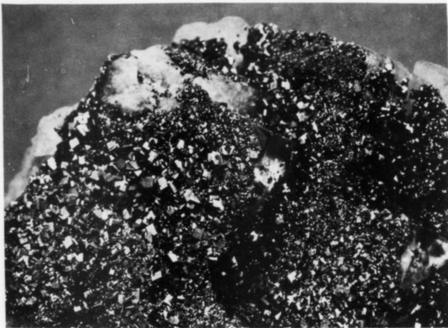
Figure 19. Cubic crystals of pyrite encrusting pale yellow fluorite. Size: 3 x 4 inches; No. 5542, collected in 1917.
