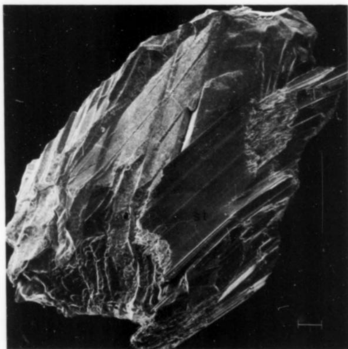
Figure 7. Platy sterryite (st) on massive guettardite. Bar represents 100 \mu\text{m} (M 35891).
