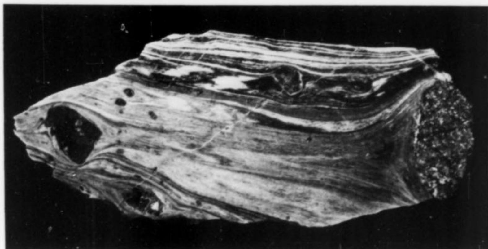
Figure 7. Flow texture in specimen from calcite-fluorite vein-dike, Fission mine. Aligned, dark mineral is antozonite , the deep purple variety of fluorite. Speckled mass at right is an entrapped rock fragment. Black mass at left is magnetite. Specimen is 13½ inches (34 cm) long (GSC 61244).
