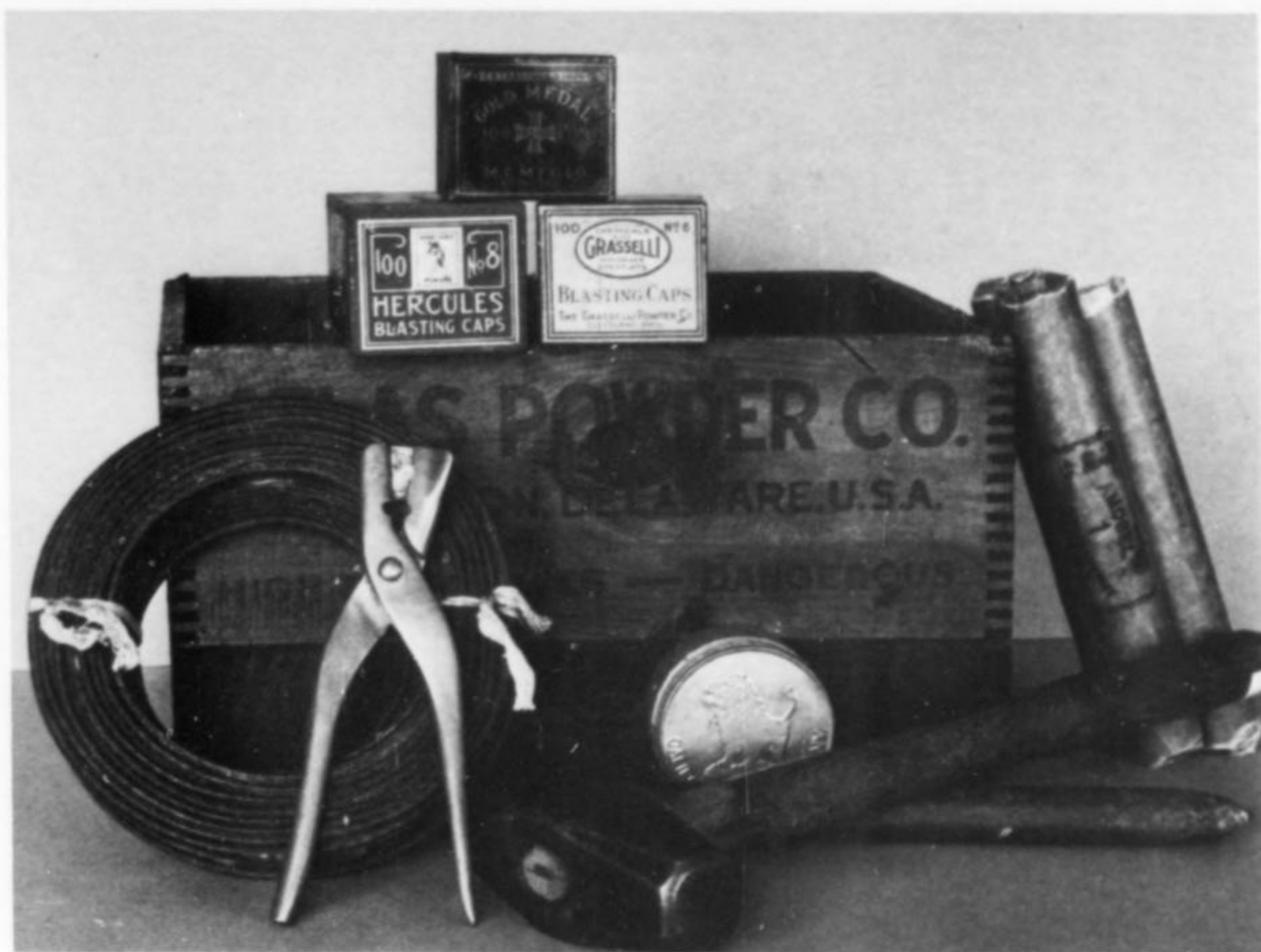
Figure 3. Blasting paraphernalia (left to right): electric blasting wire; brass fuse cutter-crimper (Don Olson collection); rectangular blasting cap tins; hand sledge and hand steel for drilling blast holes; round blasting cap tin; dynamite tubes (with wooden dowels inside); and (behind) Atlas powder box.
