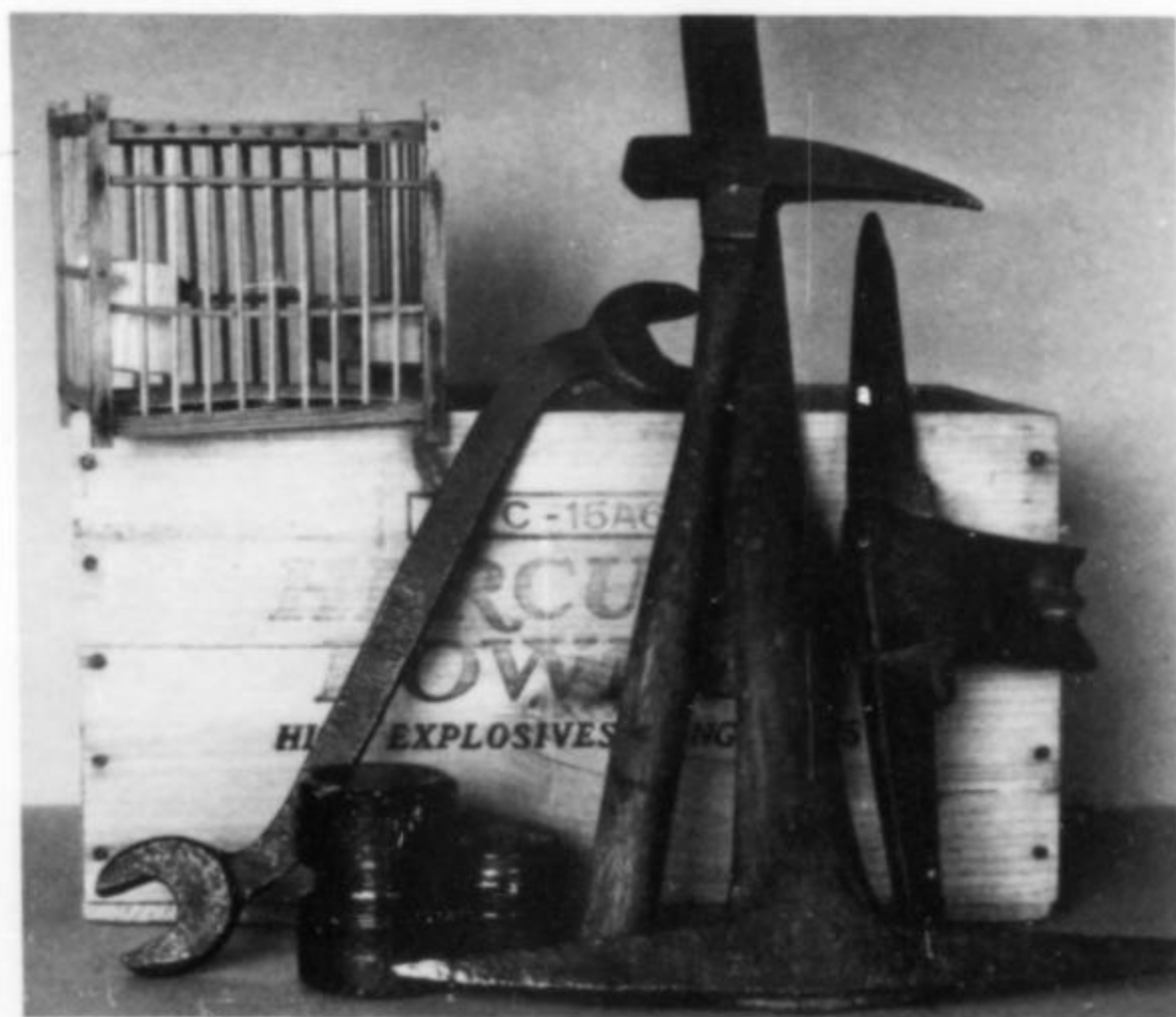
Figure 2. (left to right) Miner's canary cage (canaries were used for gas testing); heavy spanner for adjusting pneumatic rock drills (marked "COPPER QUEEN," used in Bisbee, Arizona); glass insulators for underground wiring (left one, green, is marked "JEFFREY MINE INSULATOR"; right one, purple, is marked "CALIFORNIA"); geologist's rock hammer, miner's picks, and (behind) Hercules powder box.
