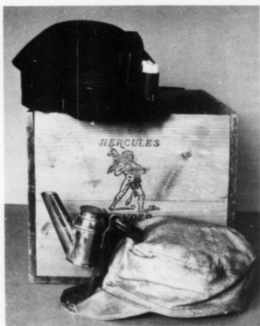
Figure 4. Miners' caps: hard rubber and leather cap with candleholder attached; soft canvas cap with "Sunshine" lamp attached; and (behind) Hercules powder box.
