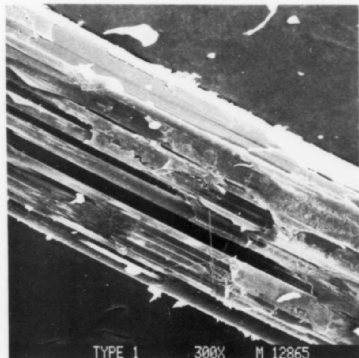
Figure 7. Detail of Fig. 6, showing the lamellar structure of the graphite crystal.
