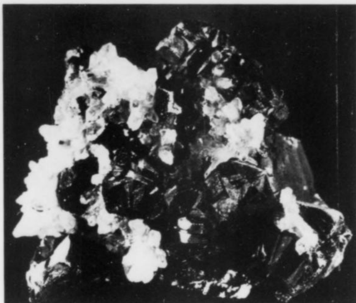
Figure 12. Black sphalerite crystals with quartz and chalcopyrite, from the 'A' bed, 2610 level. Wayne and Sara Foster collection; J. Scovil photo.
