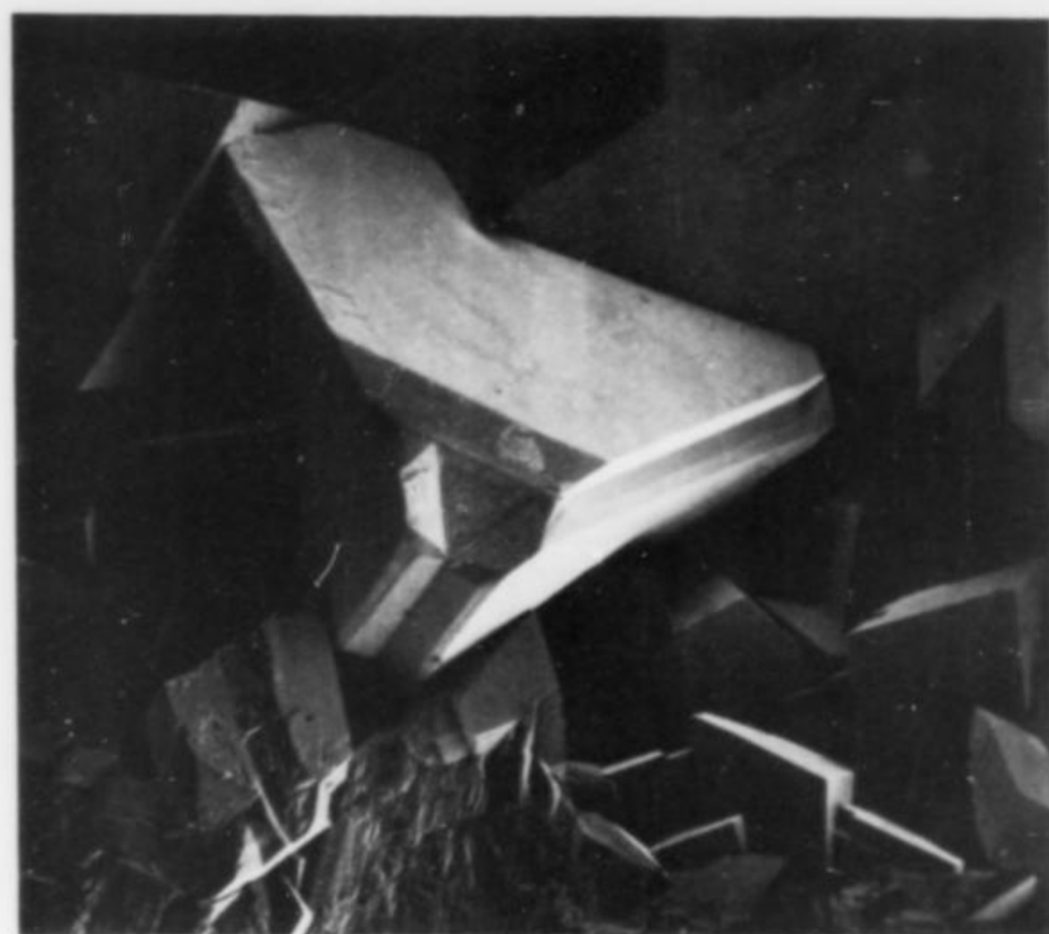
Figure 34. Sphalerite—a complex, multiply twinned fanning of sphalerite crystals, twinned by the spinel law. The largest plate is 2 mm wide.
