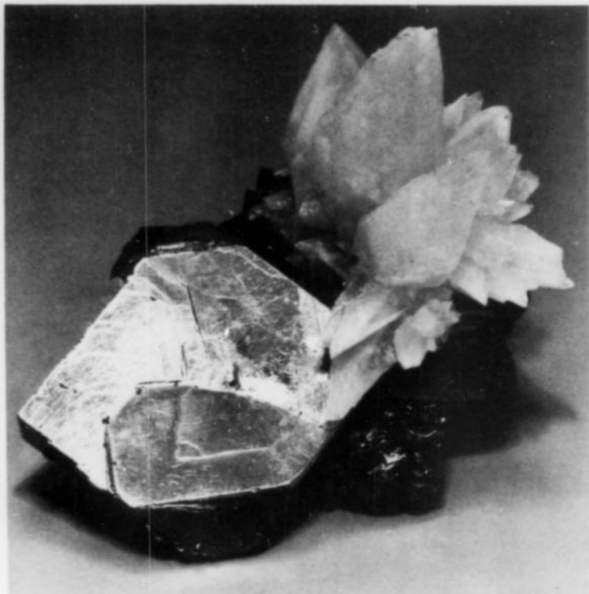
Figure 9. Cuboctahedral galena crystal 2.5 cm on edge with white calcite and black sphalerite crystals from the Gordon #2 orebody, Camp Bird mine. Collected in 1976 by T. Rosemeyer. Kosnar specimen and photo.
