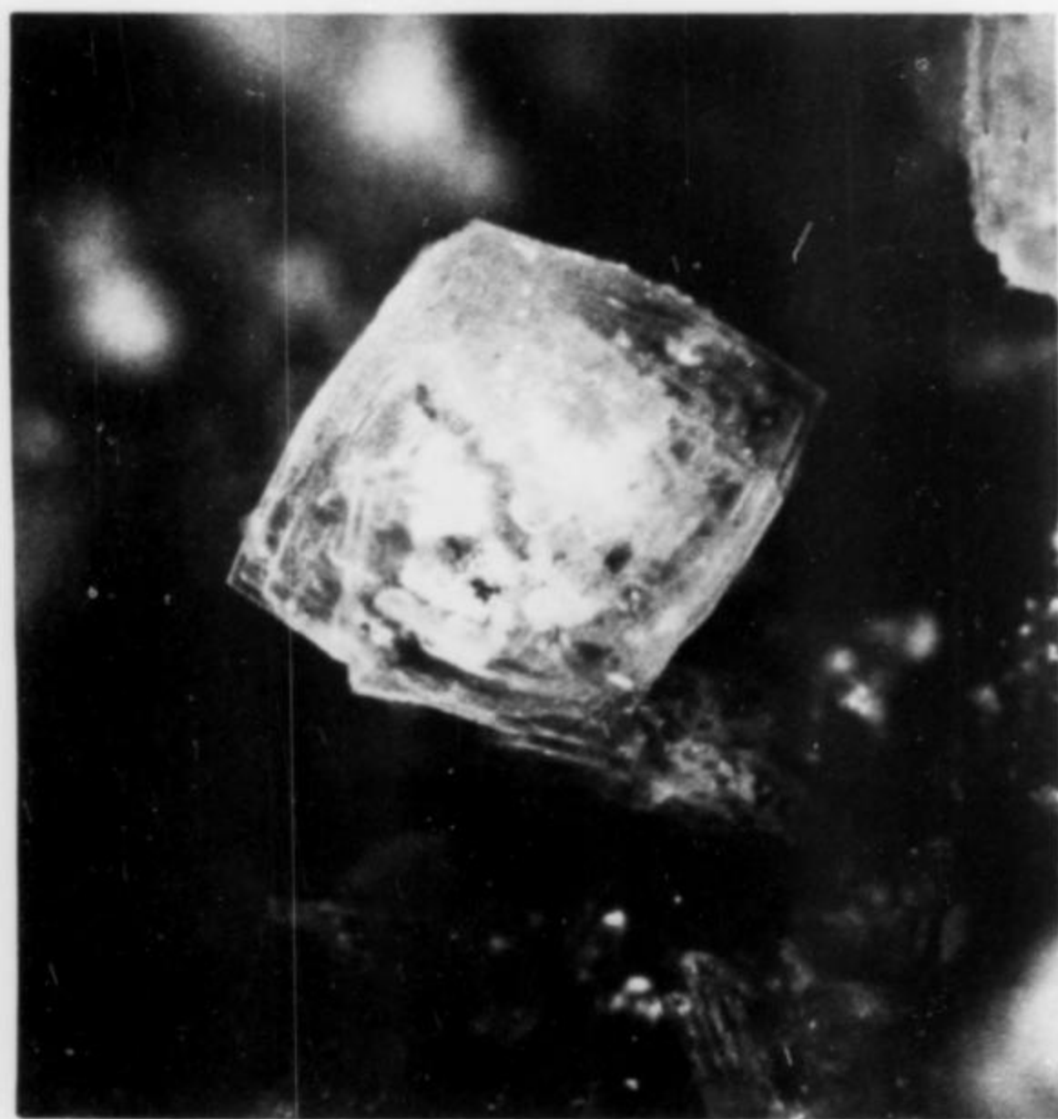
Figure 14. A whitish rosette of prehnite 0.69 mm across, with inclusions of bright copper, from the Clark mine.
