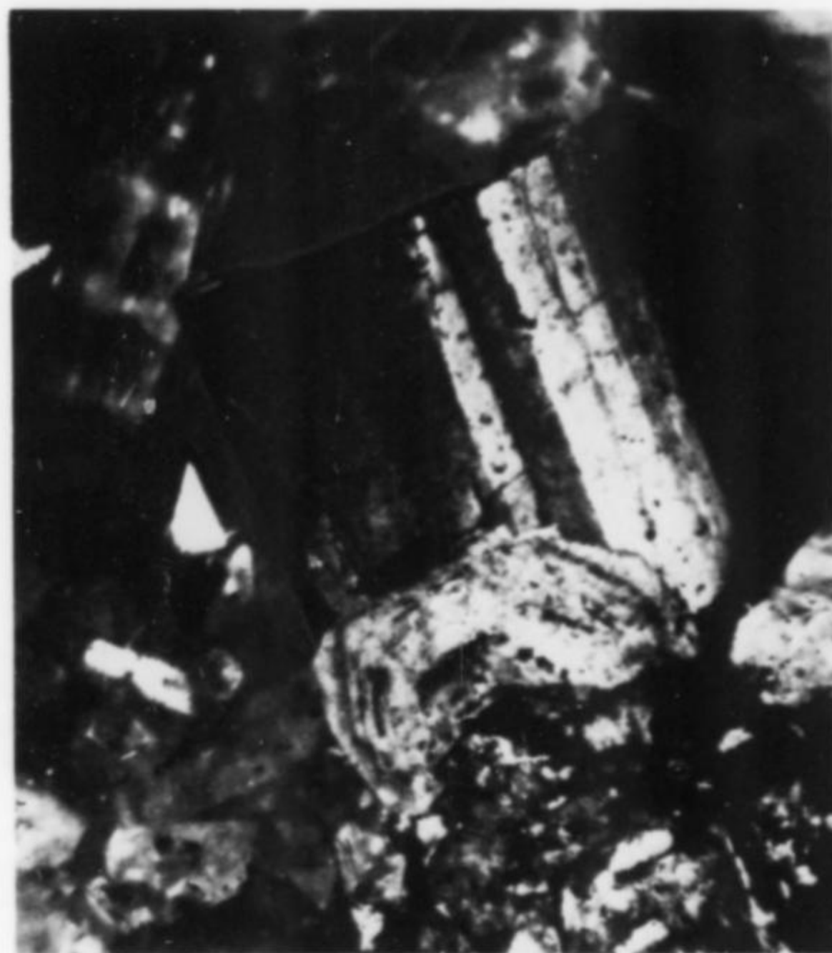
Figure 1. Bastnaesite showing re-entrant angle on complete crystal and lamellar structure of broken crystal. Height of complete crystal equals 7 mm.
