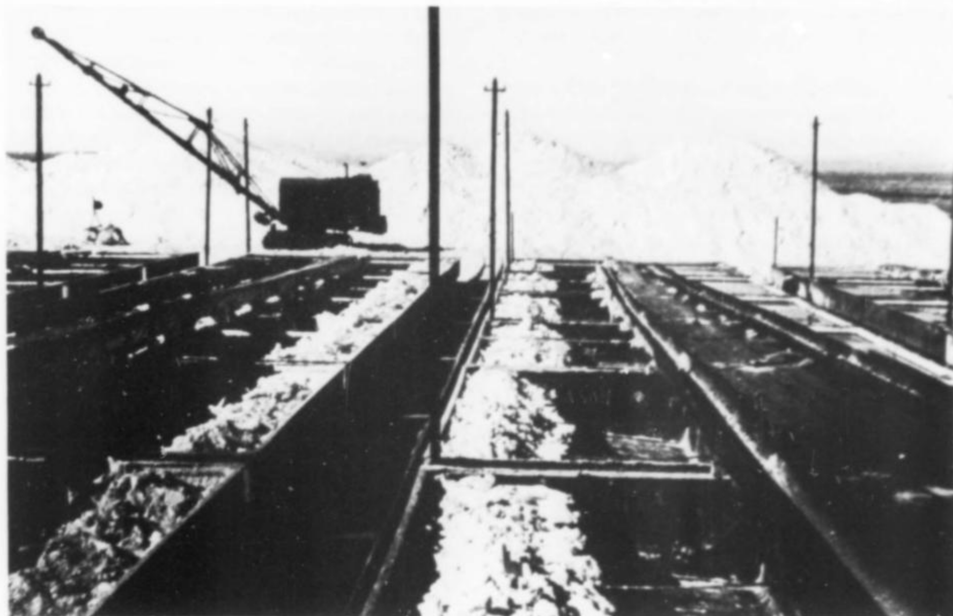
Figure 5. Evaporating tanks at Chacabuco, Chile, 1935. Crystallized nitrate is shoveled to one side, and subsequently loaded into cars for transport to the stockpile.
