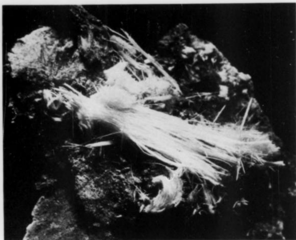
Figure 5. A specimen (6 cm across) exhibiting a sheaf of white epsomite fibers. Photo by G. Brizzi.
