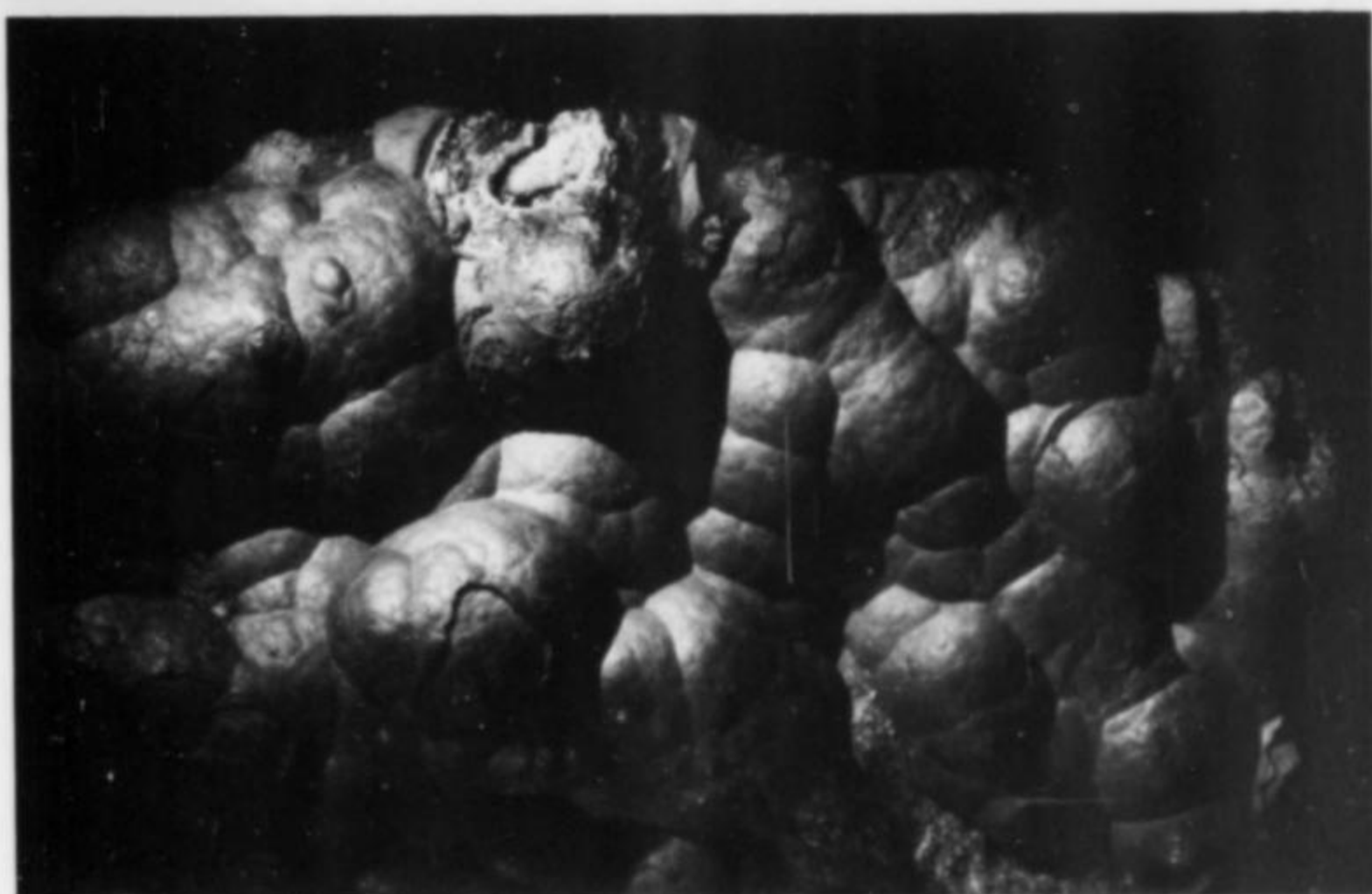
Figure 10. Red botryoidal hematite with minor quartz and specular hematite. The specular hematite has been reduced to magnetite, the botryoidal form remains hematite. The specimen is 20 cm in length; #H269, Oren Root collection, Hamilton College, Clinton, New York. Photo by S. Chamberlain.
