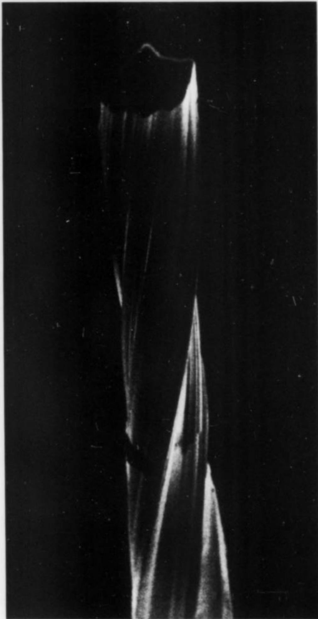
Figure 18. Millerite crystal showing spiral growth. The magnification of the SEM photomicrograph is about 2000x. Photo by G. Robinson.
