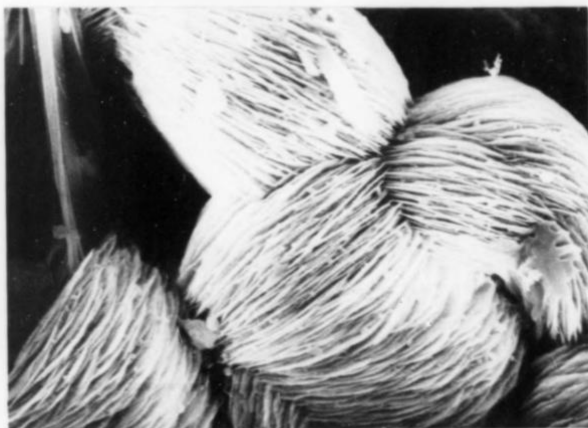
Figure 7. Ferrostrunzite with aluminian strengite on shale. (SEM photo; width of view is 46 \mu\text{m} .)
