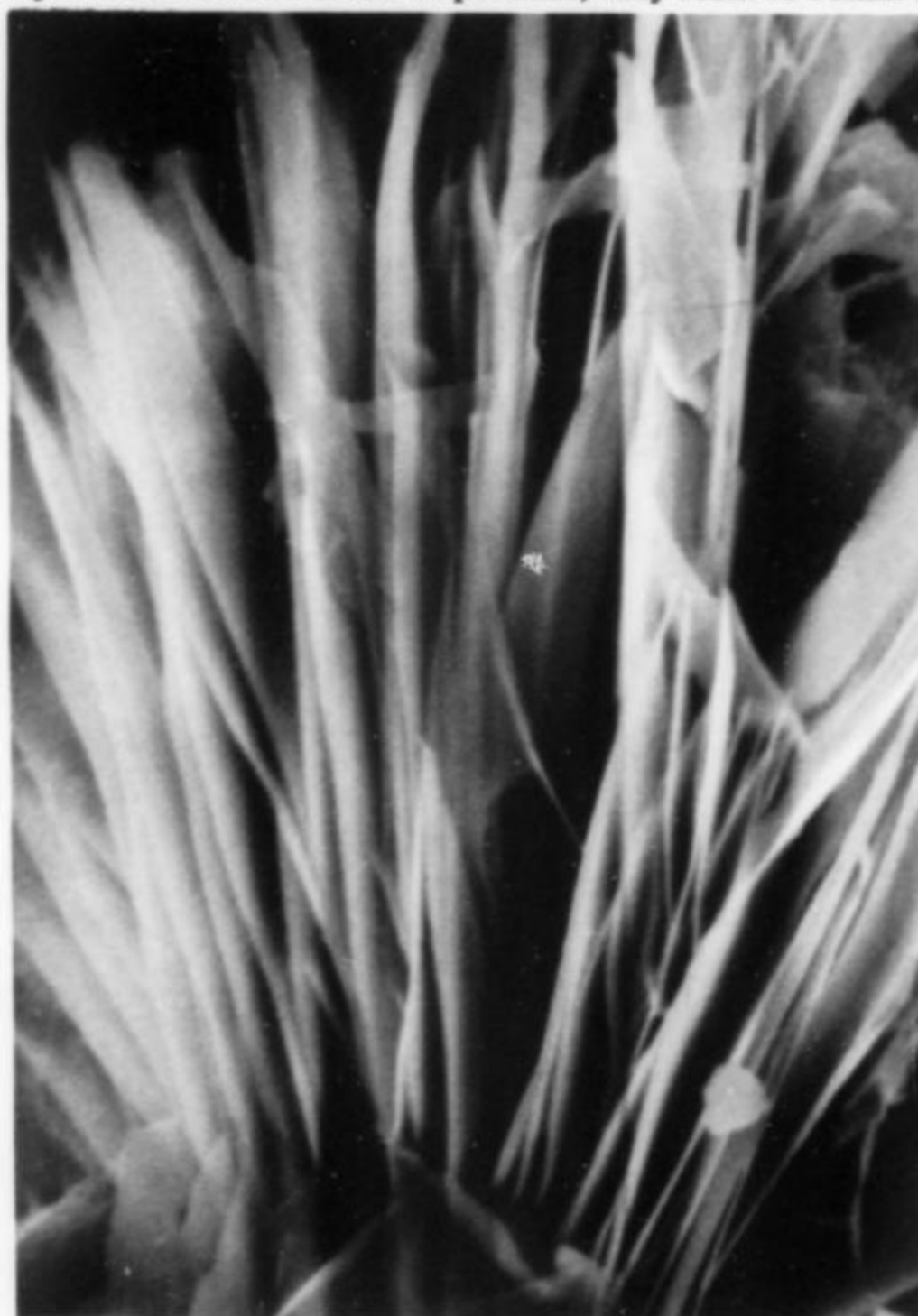
Figure 21. SEM photograph of leafy strashimirite; the view is 20 \mu\text{m} across. B. Runner photo.
