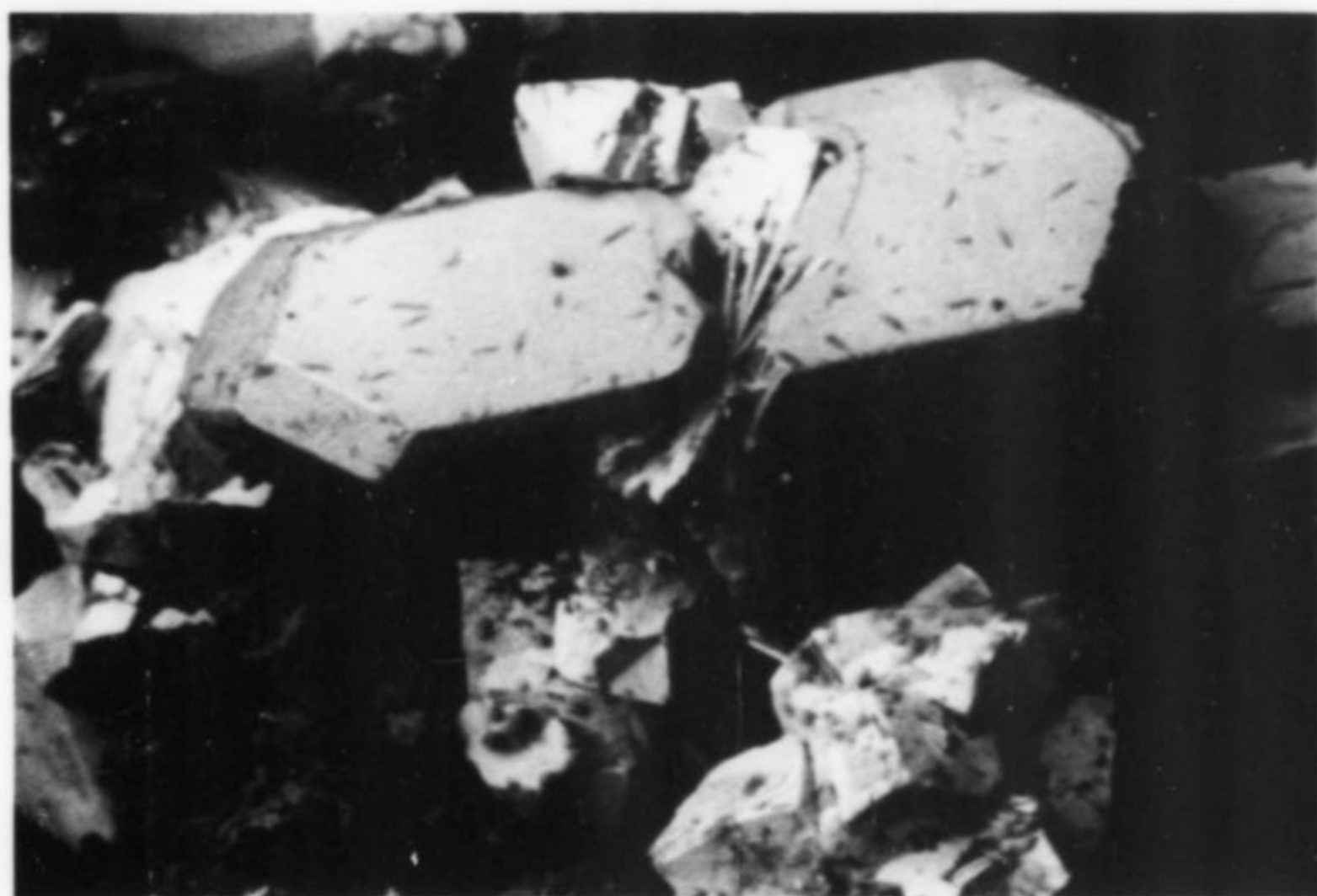
Figure 14. Bright red realgar crystal, 0.1 x 0.3 mm, containing radiating groups of stibnite and 0.1 mm rhombohedral cinnabar crystals; Dunning SEM photo, R. W. Thomssen specimen.
