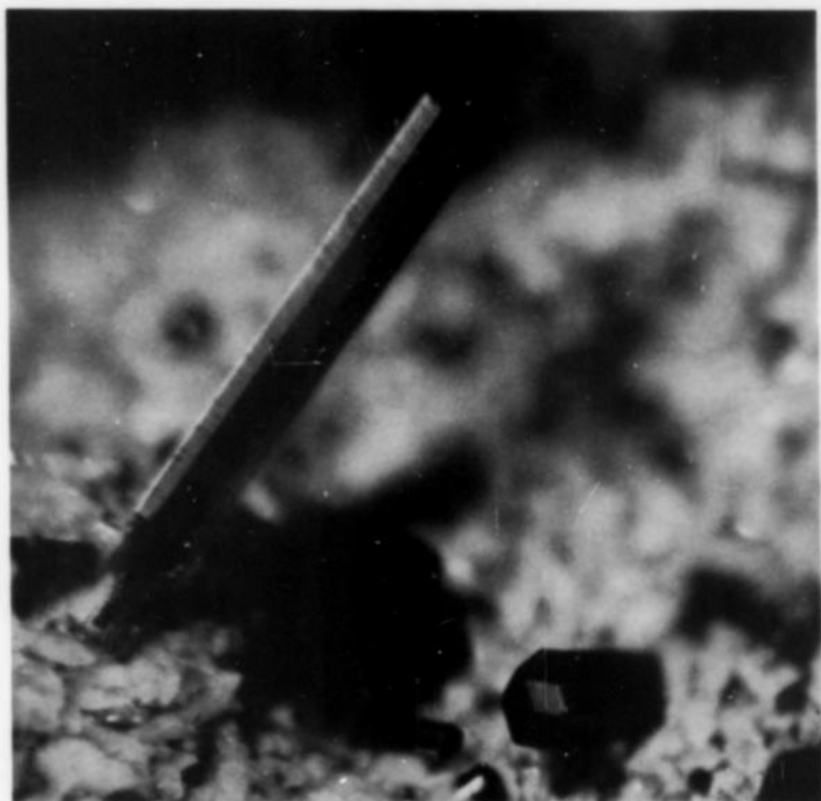
Figure 16. A 1.8 mm, greenish brown, long columnar crystal of hornblende with short columnar crystals of hypersthene of the same color, from Summit Rock, Oregon.
