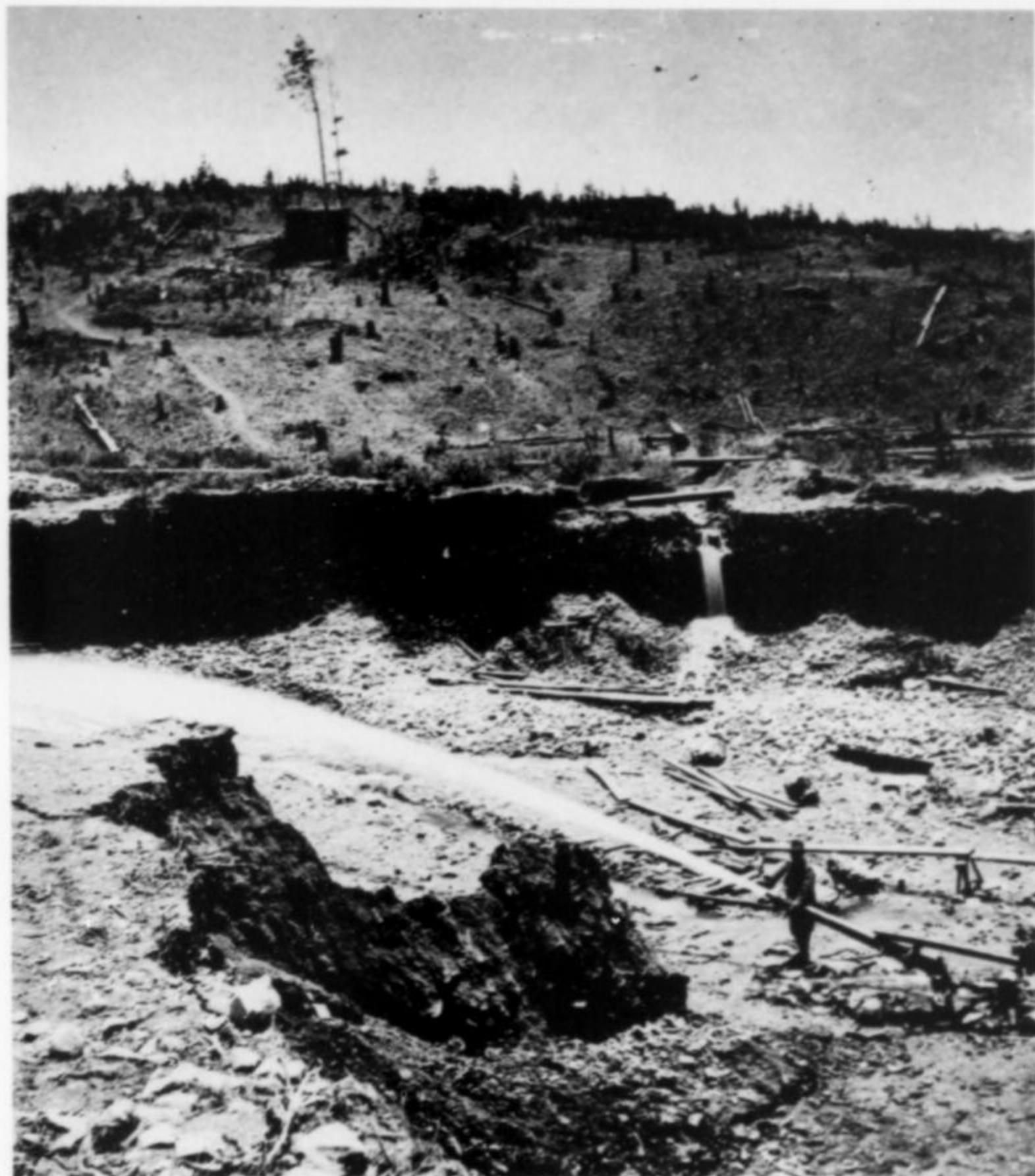
Figure 3. Hydraulic mining at Leadville. W. Prosser collection, now in the collection of the authors.
