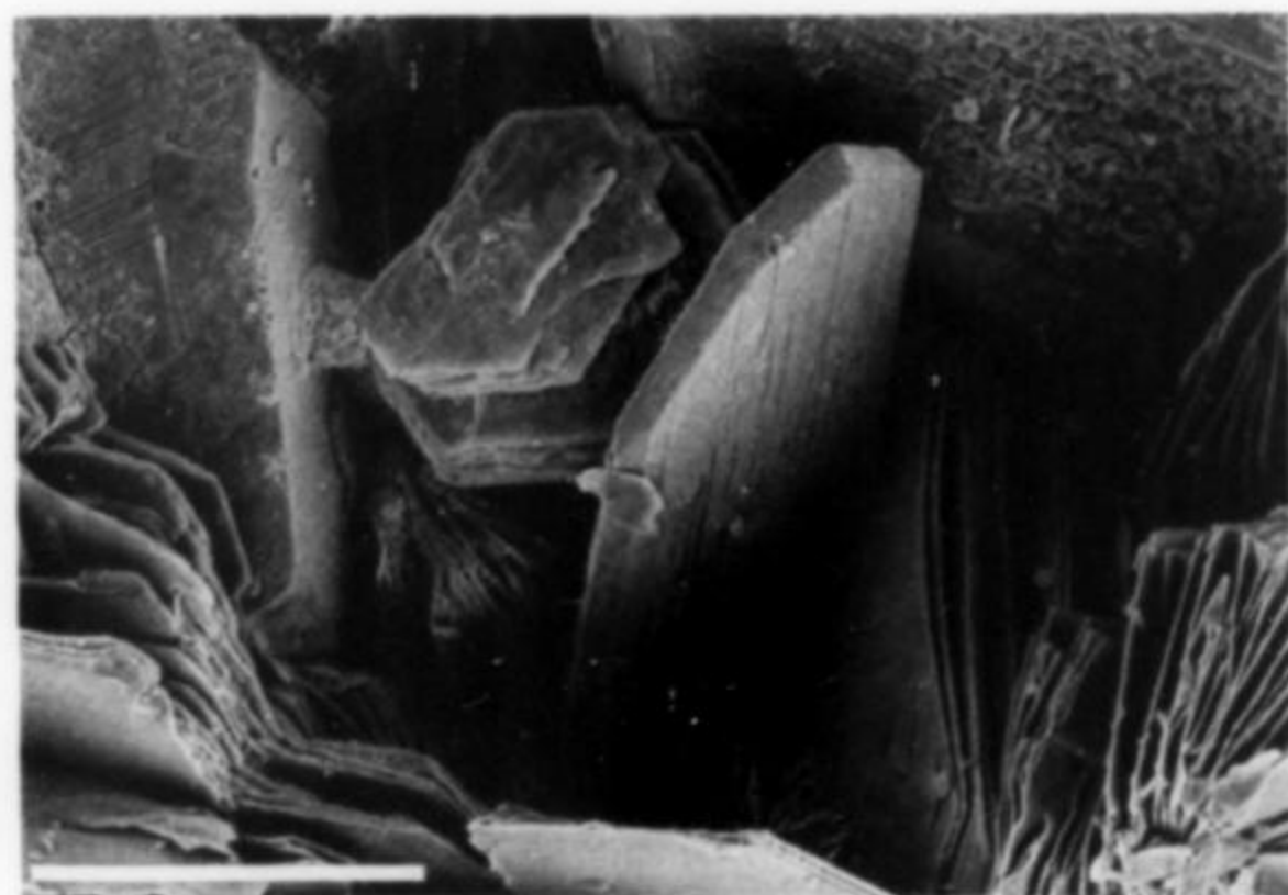
Figure 25. Brookite crystals associated with muscovite and quartz. 25 North pipe dumps, Kingsgate. Scanning electron micrograph. Scale bar is 0.1 mm. Author's specimen and photograph.
