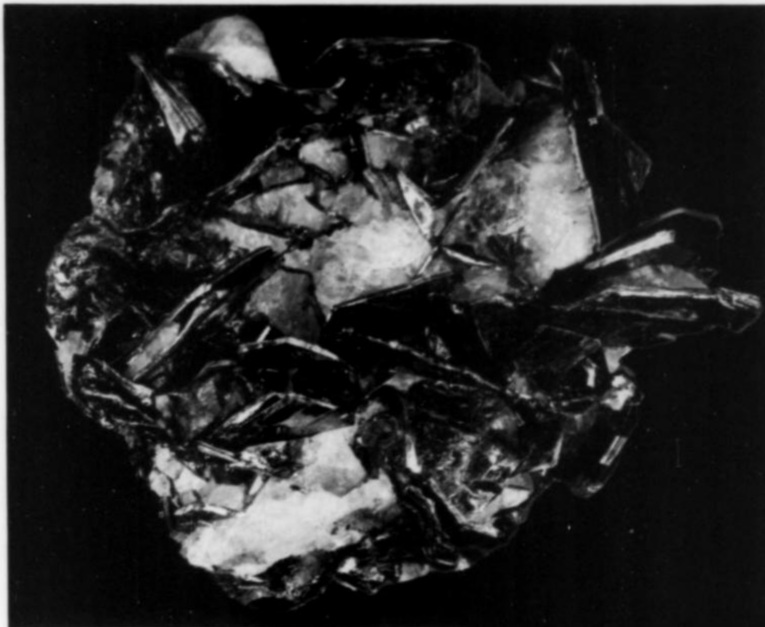
Figure 29. Tabular hexagonal molybdenite crystals encased in white quartz. Road shaft, Kingsgate, N.S.W. Australian Museum specimen D/40828, presented by Professor David Brown in 1961. 5 cm in diameter. Photograph by the author. (This specimen appeared as Plate 9 in Contributions to the mineralogy of N.S.W., Mineral Resources No. 34 , Geological Survey of N.S.W., 1926.)
