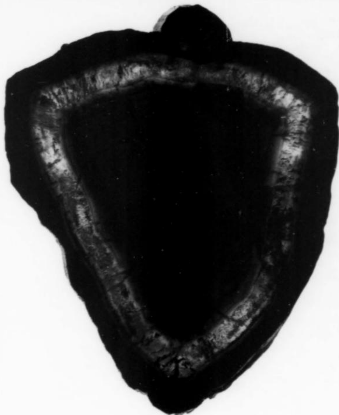
Figure 19. Crystal slab cut parallel to c showing color zoning; 7 cm across, from Brazil. B. Wöhrmann collection, photo by Karl Hartmann.
