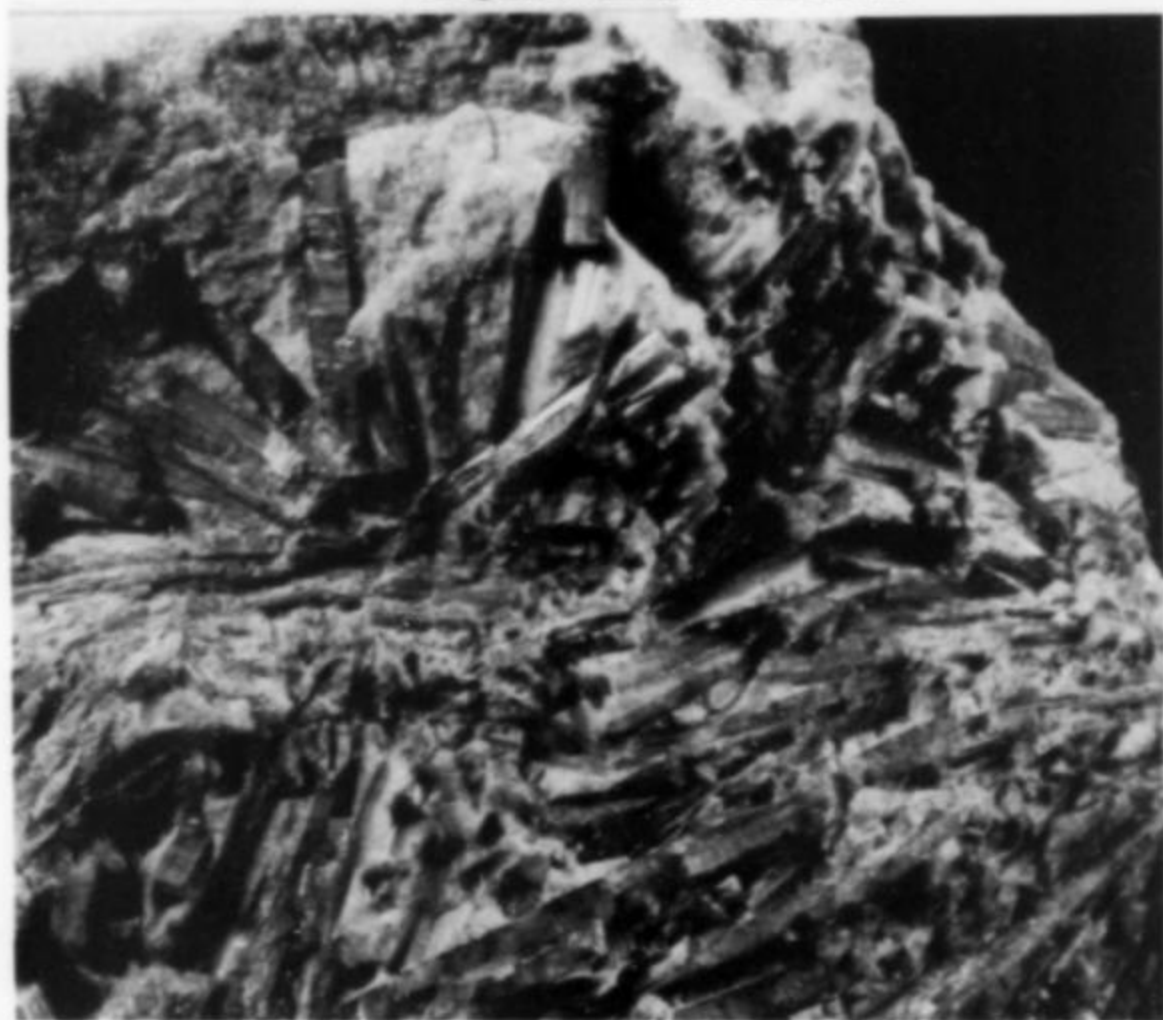
Figure 5. Pale gray, asbestiform tourmaline growing from a black single-crystal substrate. The view is about 4 cm across. Harvard Mineralogical Museum collection.
