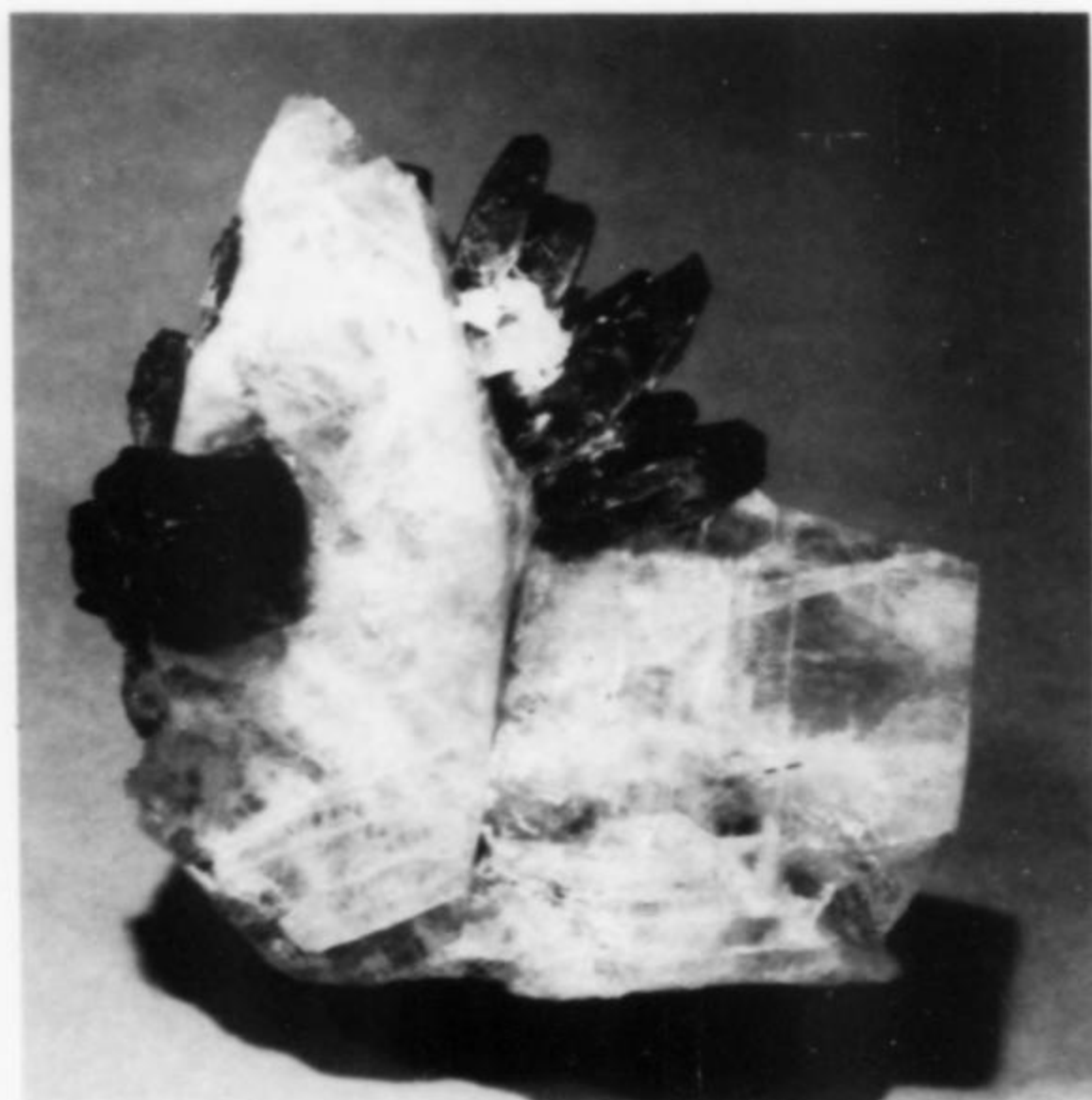
Figure 32. Yellowish green, sub-parallel aggregate of zircon crystals (average 1.5 cm) on a matrix of buff-colored albite crystals. Individual crystals exhibit tetragonal prism {110} and dipyramid {111} faces; from near Stak Nala, Gilgit division, Pakistan. AMNH 97490; photo by Olivia Bauer and Jackie Beckett.
