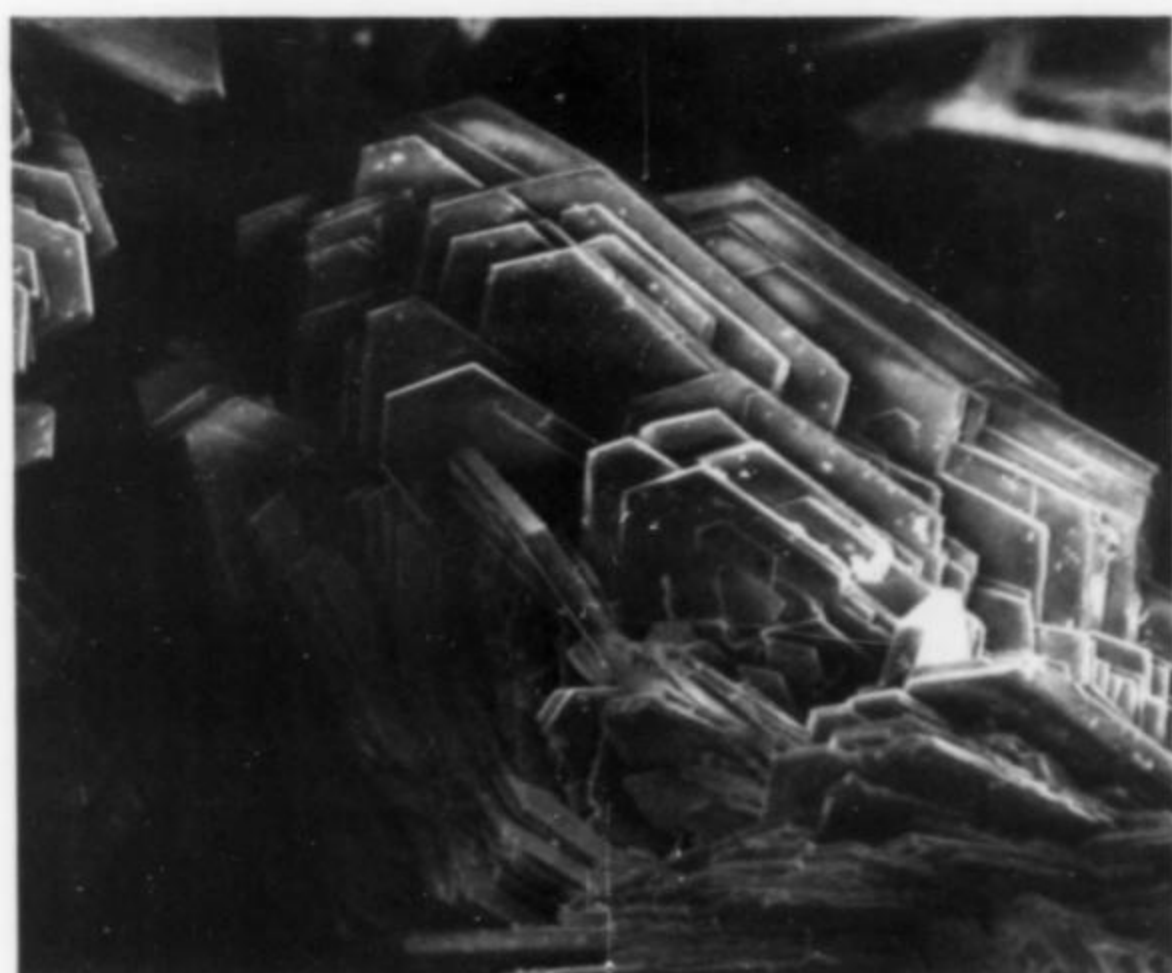
Figure 5. SEM photograph of a cluster of calcioferrite crystals up to 0.2 mm in size.
