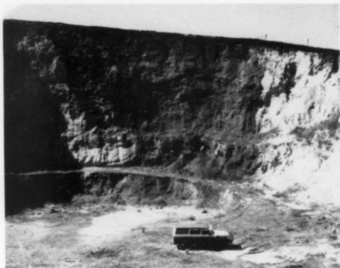
Figure 2. North wall of the Moculta quarry. The dark area behind the truck is the main phosphate orebody. Immediately to the right and at the junction with the lighter colored rock is the jarosite body in which the calcioferrite was found.
