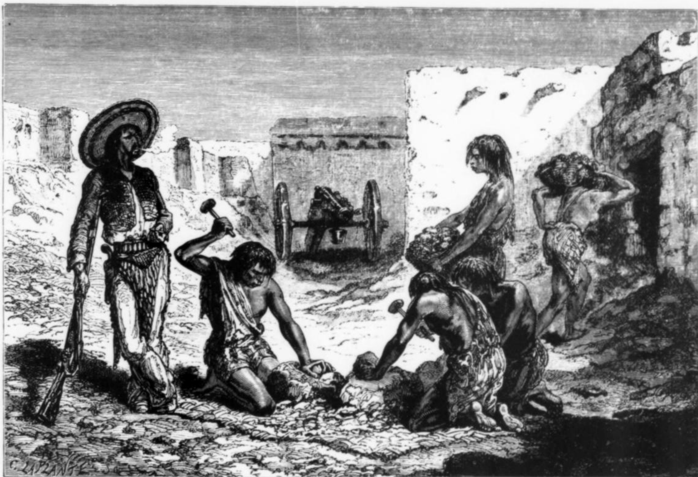
Figure 2. Indian prisoners employed as forced labor under the Spanish, cobbing out silver ore at a mine in Chihuahua (Simonin, 1869).
