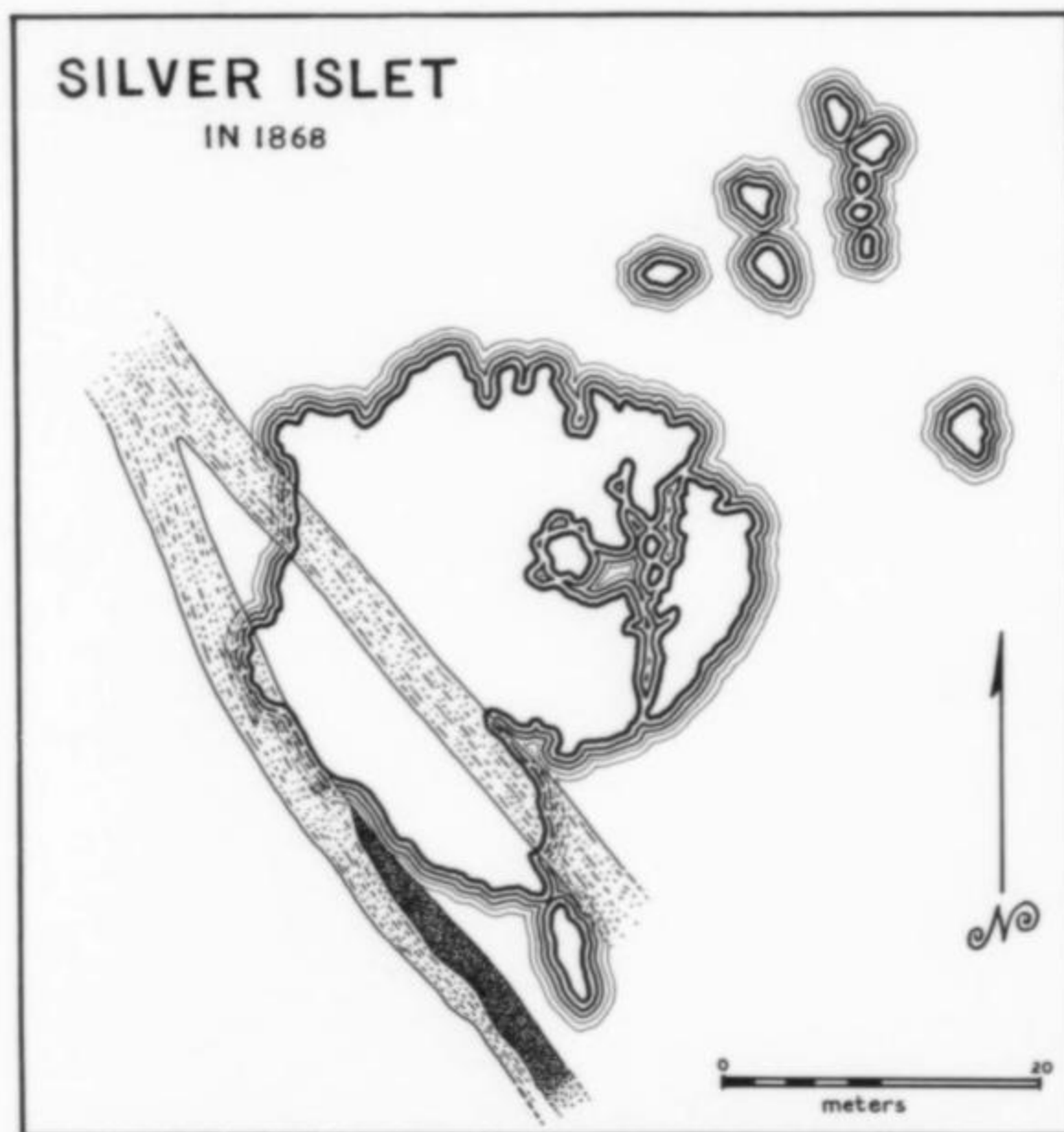
Figure 2. Silver Islet as it was when first discovered. Note how the vein splits in two, surrounding a "horse" of country rock. The rich part of the outcrop (shown dark) was visible under shallow water (after Macfarlane, 1879).
