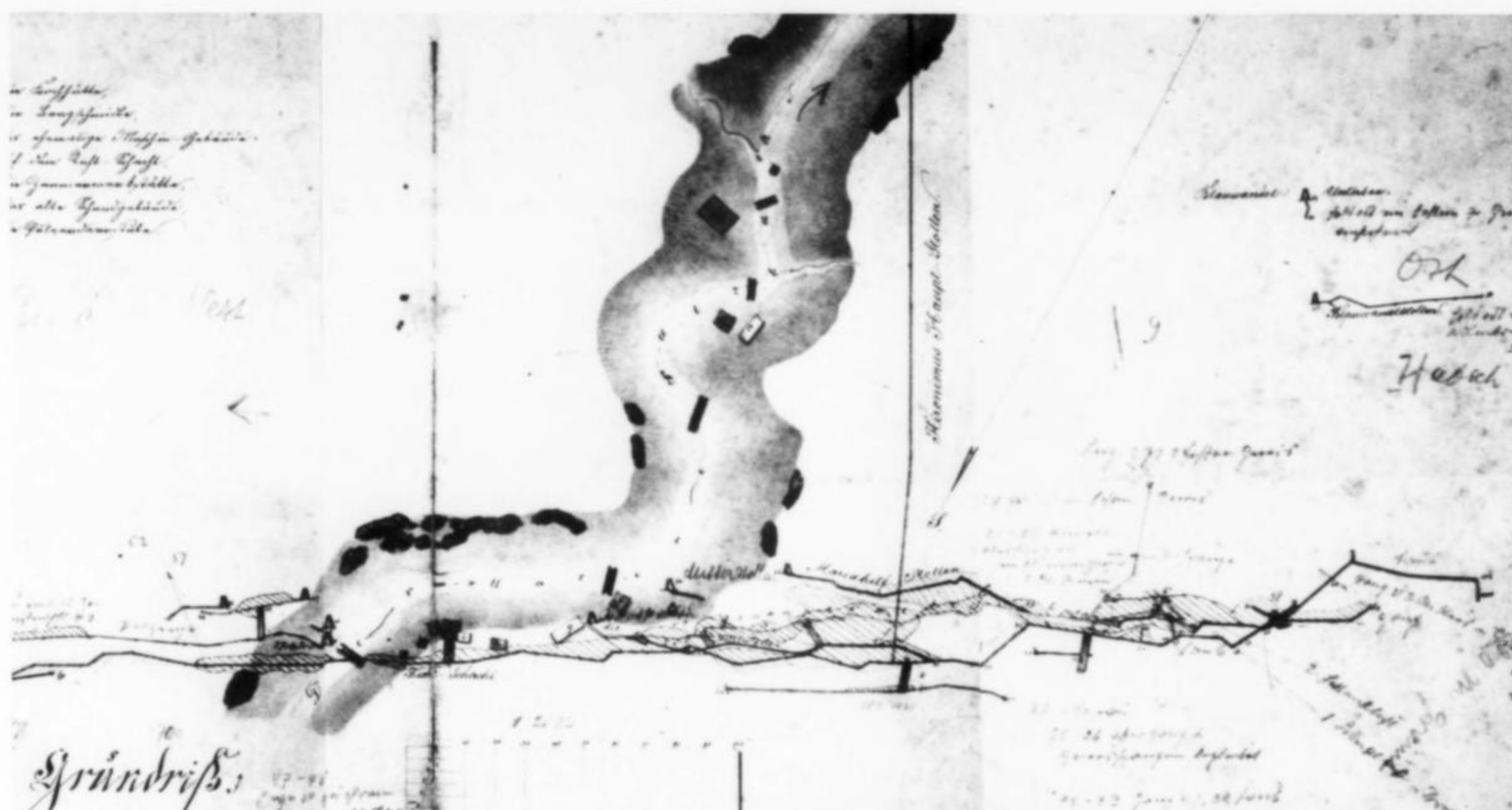
Figure 3. A portion of the Untersulzbachtal in 1785, showing extensive workings: the old copper mining area (across the bottom), and also the Blauwandel and Blauwandstollen (upper right) near the subsequently discovered Knappenwand.
